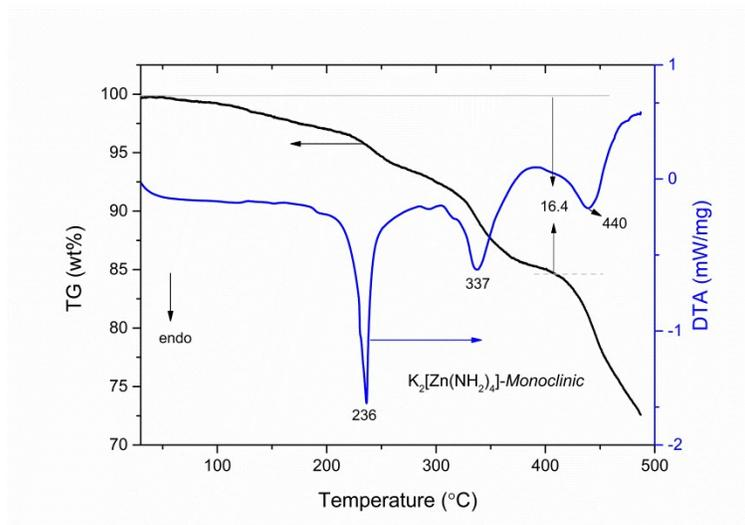
Fig. S1 TG-DTA curves of the monoclinic  $K_2[Zn(NH_2)_4]$  heating from 30 °C to 500 °C in Argon with a ramping rate of 5 °C/min.
