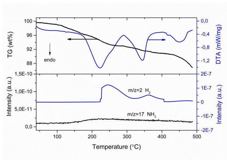
Fig. S2 TG-DTA-MS curves of the as ball milled  $K_2[Mn(NH_2)_4]-8LiH$  sample, heating from 30 °C to 500 °C in Argon with a ramping rate of 5 °C/min.
