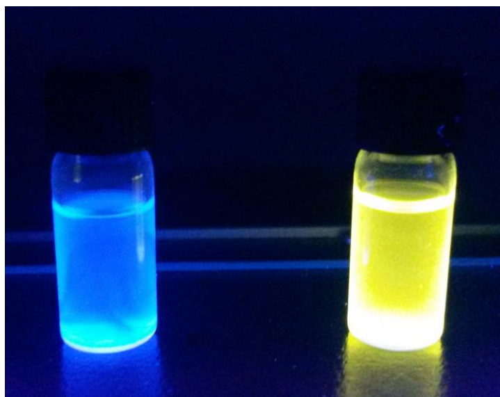
Figure S43 Fluorescence behaviour of PAT 1 (left) and pyrazoline 3 (right) irradiated with the UV hand lamp at 365 nm.
