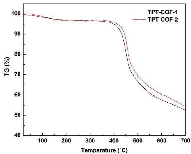
Fig. S11 TGA measurement for TPT-COF-1 (black) and TPT-COF-2 (red).
