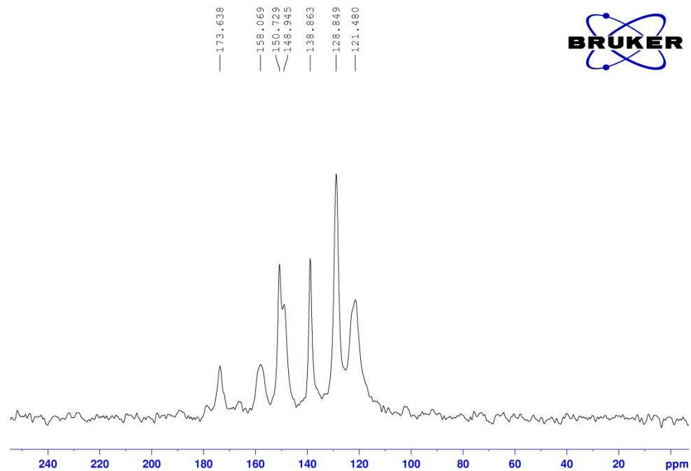
**Fig. S10**  $^{13}\text{C}$  CP-MAS NMR spectra for TPT-COF-2.
