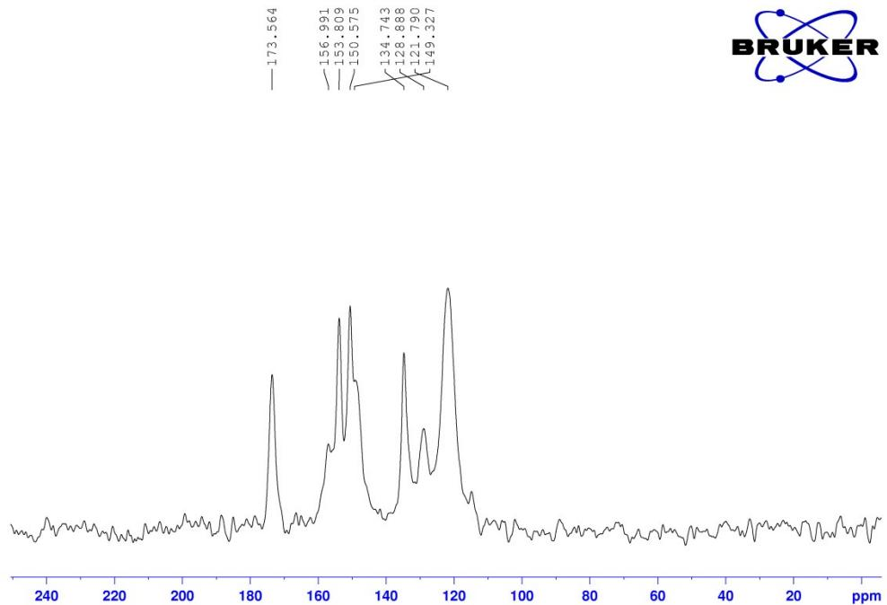
**Fig. S9**  $^{13}\text{C}$  CP-MAS NMR spectra for TPT-COF-1.
