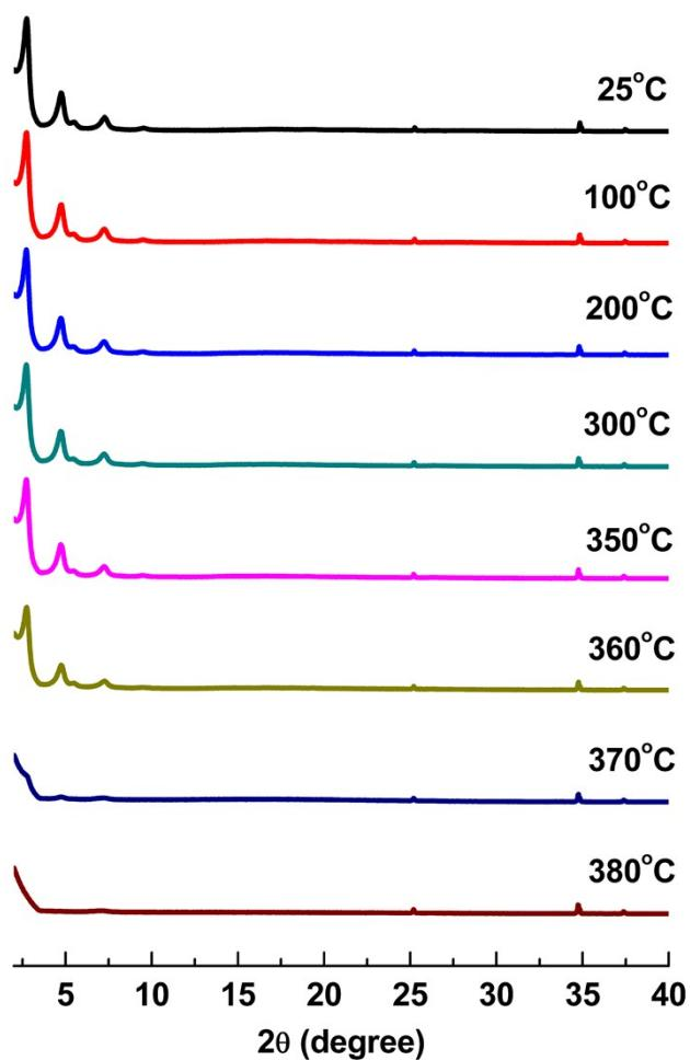
**Fig. S13** Variable temperature XRD for TPT-COF-2.
