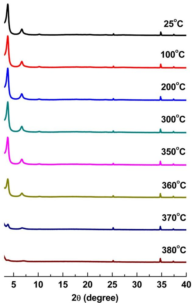
Fig. S12 Variable temperature XRD for TPT-COF-1.
