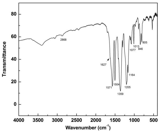
**Fig. S6** The FTIR spectra of TPT-COF-1.
