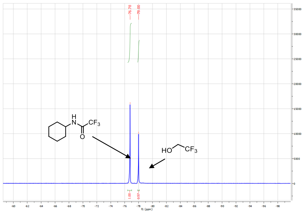
Figure S1. ^{19}\text{F}\{^1\text{H}\} NMR spectrum of the catalytic reaction of (4- N,N -dimethylphenyl)-2,2,2-trifluoroacetamide described in Table 2, entry 3 (ns = 1, d1 = 1 sec, \text{CDCl}_3 , 23 °C).
