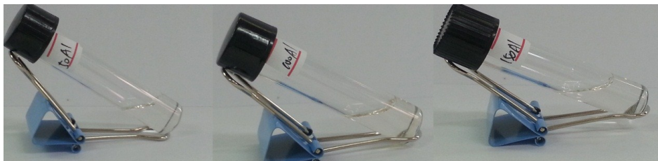
Fig. S2 Photographs of typical samples after 48 h. c_{\text{NDC}} = 100 \text{ mmol}\cdot\text{L}^{-1} and c_{\text{Al}^{3+}} (from left to right) = 50, 100, 150 \text{mmol}\cdot\text{L}^{-1} , respectively.
