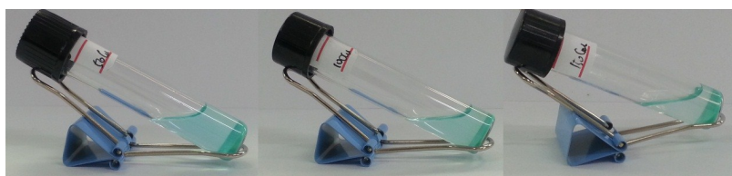
Fig. S4 Photographs of typical samples after 48 h. c_{\text{NDC}} = 100 \text{ mmol}\cdot\text{L}^{-1} and c_{\text{Cu}^{2+}} (from left to right) = 50, 100, 150 \text{mmol}\cdot\text{L}^{-1} , respectively.
