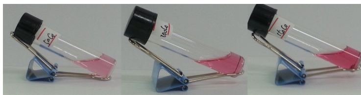
Fig. S3 Photographs of typical samples after 48 h. c_{\text{NDC}} = 100 \text{ mmol}\cdot\text{L}^{-1} and c_{\text{Co}^{2+}} (from left to right) = 50, 100, 150 \text{mmol}\cdot\text{L}^{-1} , respectively.
