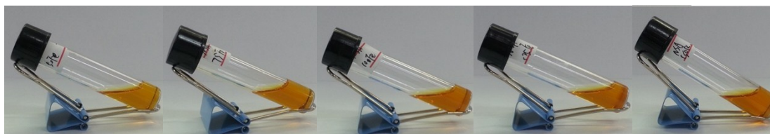
Fig. S5 Photographs of typical samples after 48 h. c_{\text{NSA}} = 100 \text{ mmol}\cdot\text{L}^{-1} and c_{\text{Fe}^{3+}} (from left to right, from top to bottom) = 50, 75, 100, 125, 150 \text{mmol}\cdot\text{L}^{-1} , respectively.
