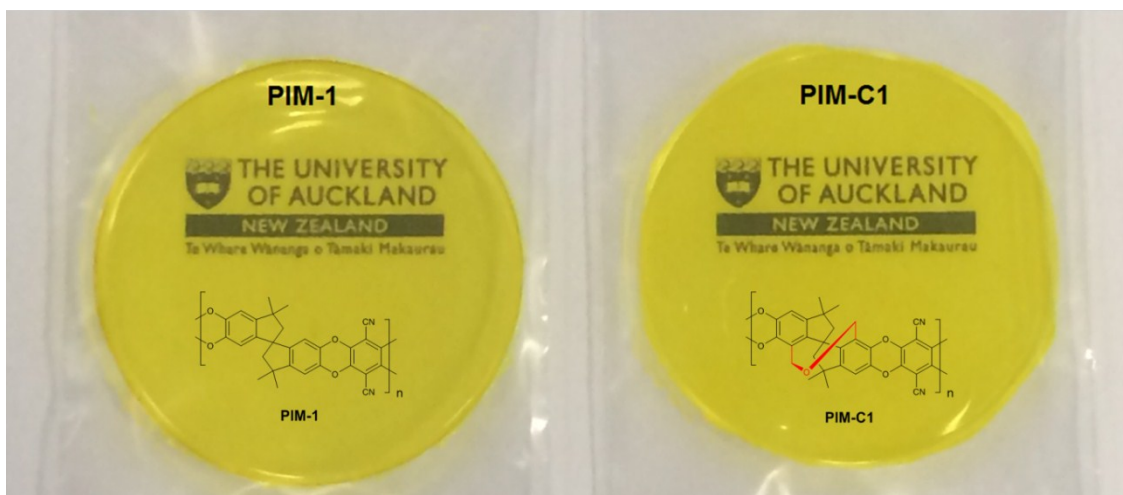
Fig. S8. Optically clear films of PIM-C1 and PIM-1 for gas permeation measurements.
