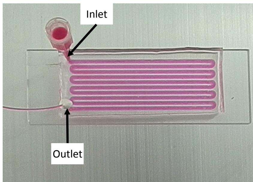
**Fig. S12 The photo of microfluidic device.**
