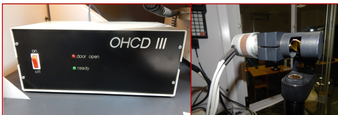
Figure S8. Optical Heating and Crystallization Device (OHCD).
