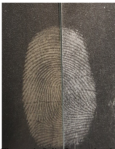
S.I. Figure 4. Split fingerprint developed with C-SiO 2 nanoparticles (left half) commercial WFP (right half). The image was captured under white light.
