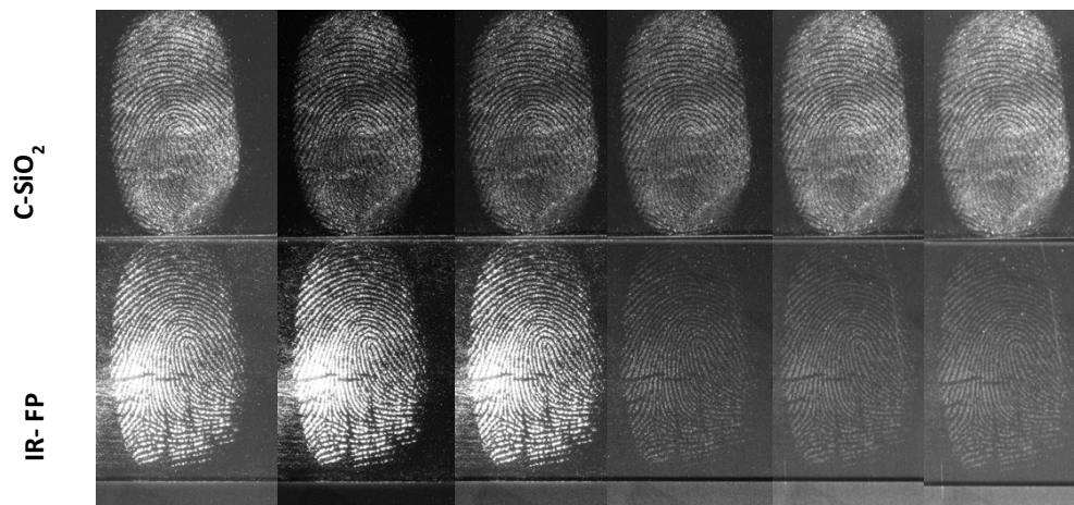
S.I. Figure 7. Comparison between the C-SiO 2 (upper images) and a commercial fluorescent fingerprint powder on a glass slide investigated on a crime lite imager.
