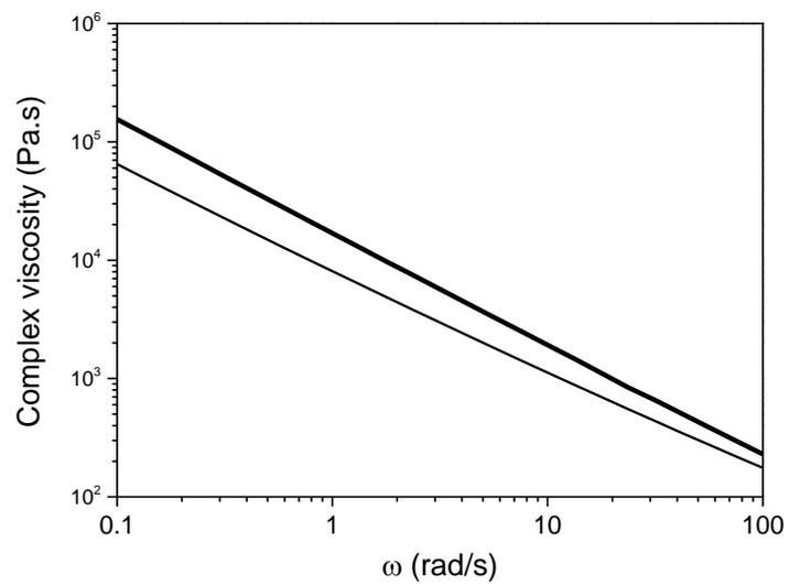
**Figure S11.** Complex viscosity versus angular frequency for elastomers **4** (thick line) and **5** (thin line).
