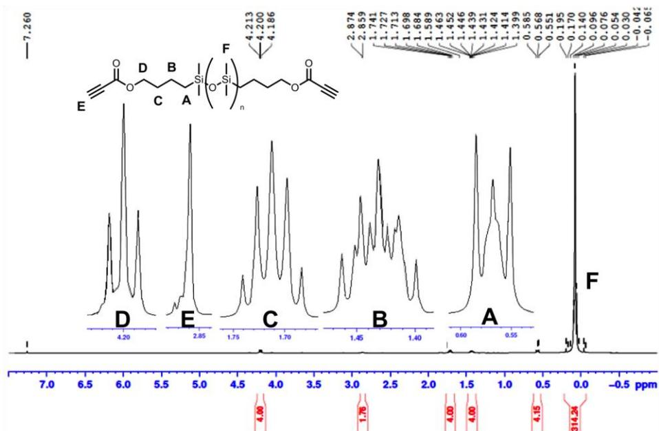
**Figure S3.** <sup>1</sup>H NMR spectra of propiolate-PDMS 2 in CDCl<sub>3</sub>:
