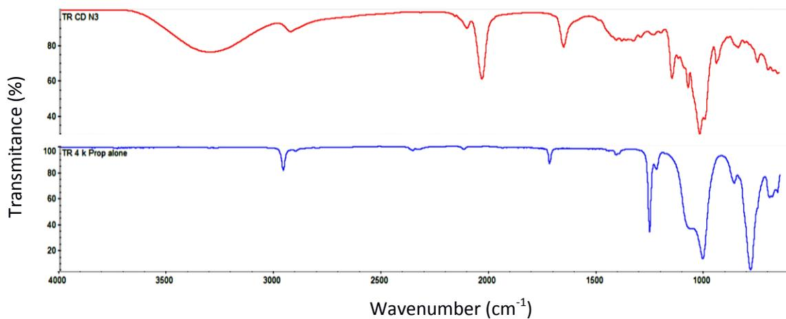
**Figure S2.** FTIR spectra of starting material: (top)  $N_3$ - $\beta$ -CD **1**; (bottom) Propiolate-PDMS **2**.
