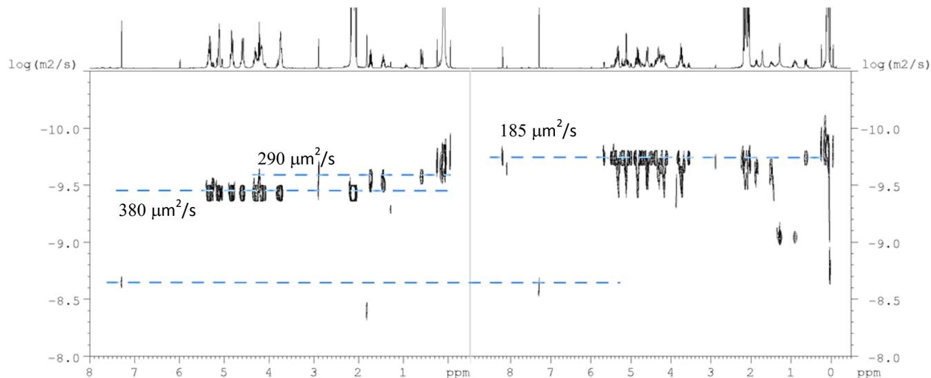
**Figure S16:** 2D DOSY maps of (left) the acetylated  $\beta$ -CD **6** and the propiolate PDMS **2** mixed together in  $\text{CDCl}_3$  and (right) the polymer **7** from click reaction in  $\text{CDCl}_3$ .
