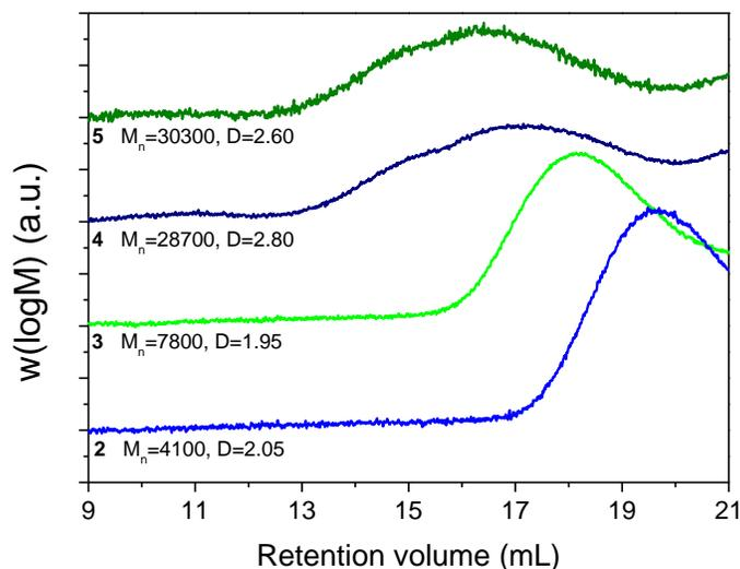
**Figure S15:** SEC analyses in THF of the original propiolate polymers **2**, **3** and final elastomers **4** and **5** after the click reaction with **1**, and solubilization in a chaotropic salt/THF solution. The fact that the molar masses of the complexes show an increased mass suggests that some aggregation is occurring owing to the poor THF solubility of the CD end chains.
