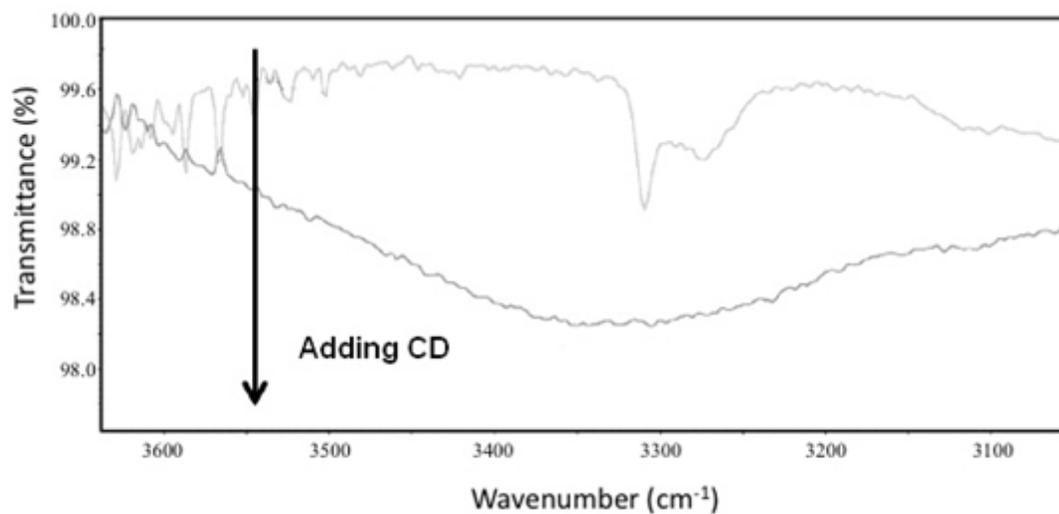
**Figure S5.** Zoom on the FTIR region of OH stretch for propiolate PDMS **2** (top) and elastomer **4** (bottom).
