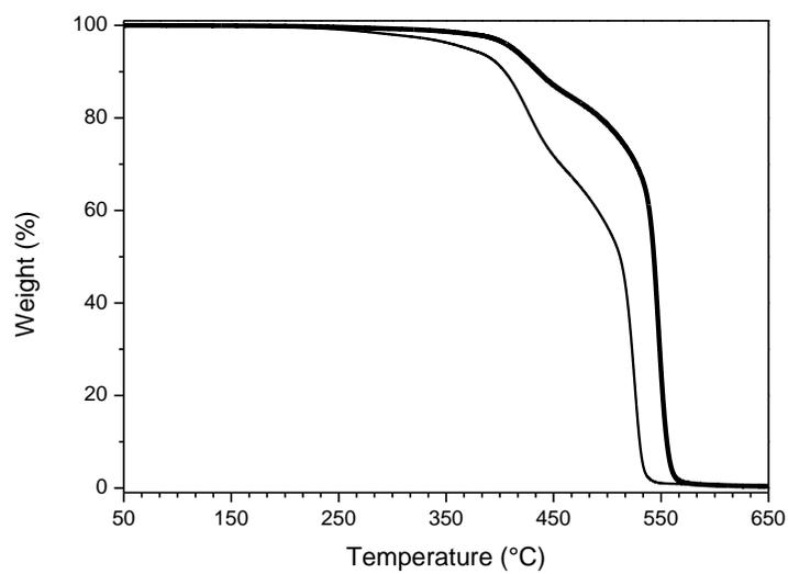
**Figure S8:** TGA of **4** (thin line) and **5** (thick line) elastomers.
