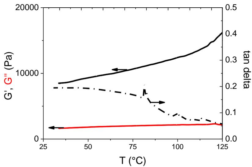
**Figure S10.** Temperature sweeps at constant strain for elastomer **4**.
