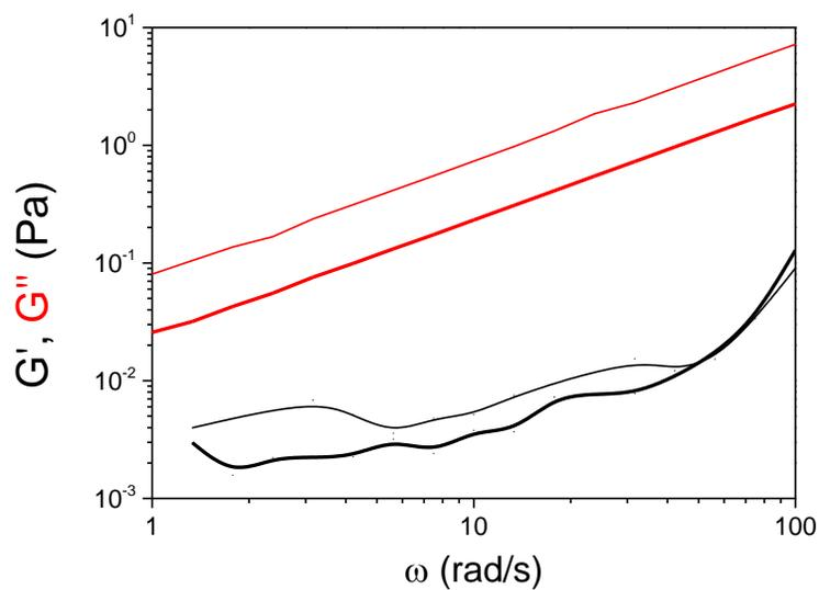
**Figure S9.** Frequency sweeps at constant strain for propriolate-PDMSs **2** (thick line) and **3** (thin line).
