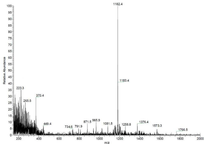
**Figure S1.** Electrospray-mass spectrum of  $N_3$ - $\beta$ -CD protonated by  $Na^+$  (main peak at 1183.4 g/mol).
