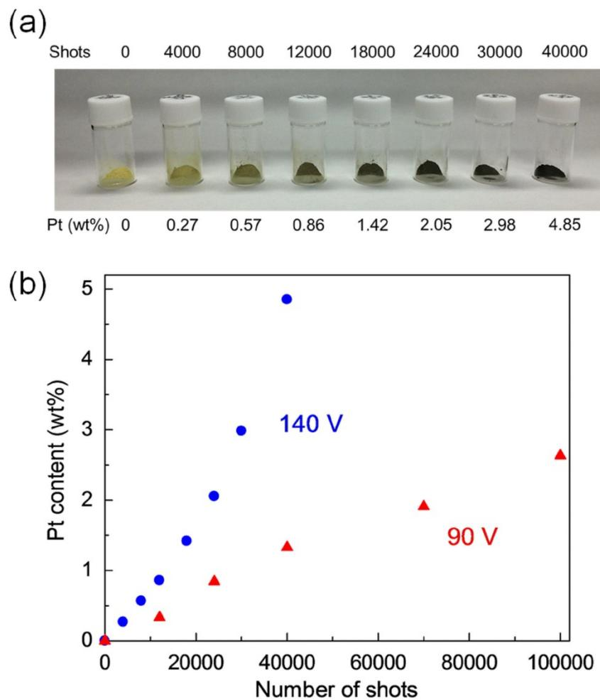
**Fig. S12** (a) Photos of samples of  $\text{Pt}^n/\text{Zn-MOF-74}$  (shot number  $n = 0, 4000, 8000, 12000, 18000, 24000, 30000,$  and  $40000$ ) prepared at the applied voltage of  $140\text{ V}$ . (b) Relation between number of shots and Pt content of the samples prepared at (blue)  $140\text{ V}$  and (red)  $90\text{ V}$ , estimated by ICP-AES measurements.
