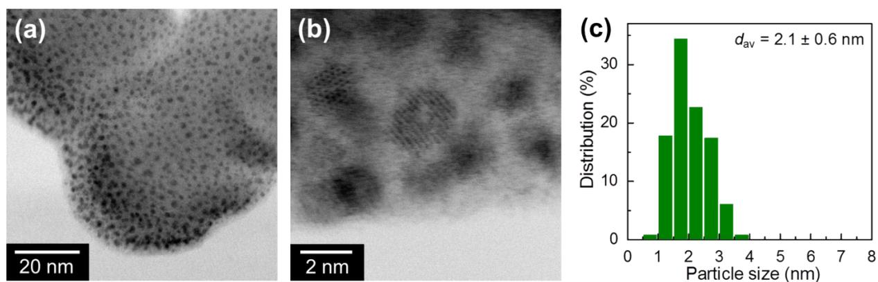
**Fig. S18** (a) STEM image, (b) HR-STEM image, and (c) size-distribution of **Pt-Co/ZIF-8**.
