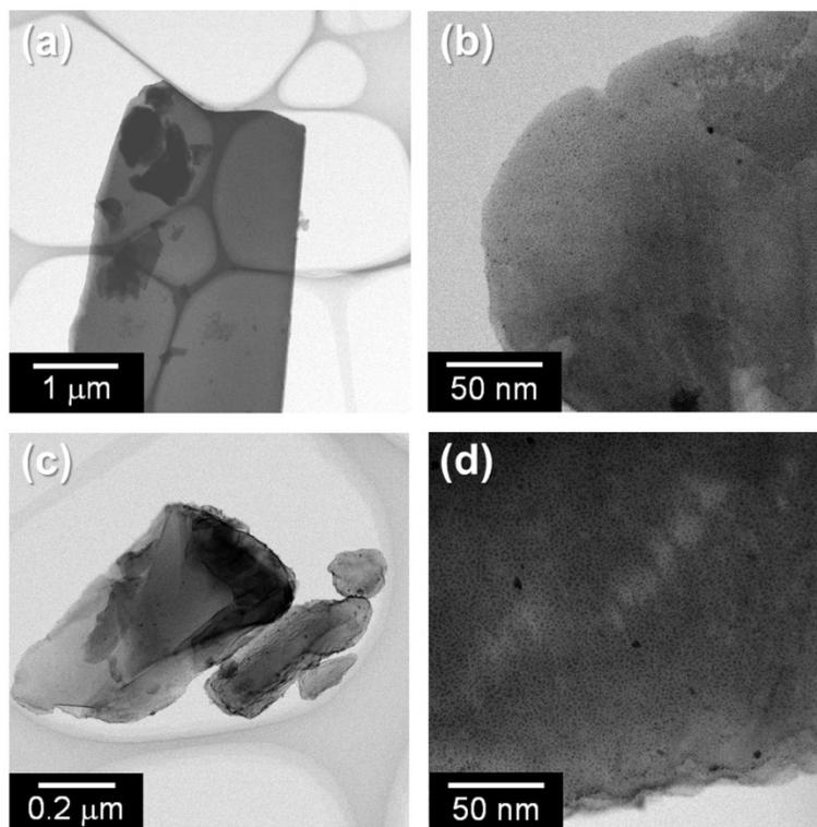
**Fig. S15** STEM images exemplified by (a, b)  $\text{Pt}^{24000}/\text{Zn-MOF-74}$  and (c, d)  $\text{Pt}^{70000}/\text{Zn-MOF-74}$  (prepared at 90 V).
