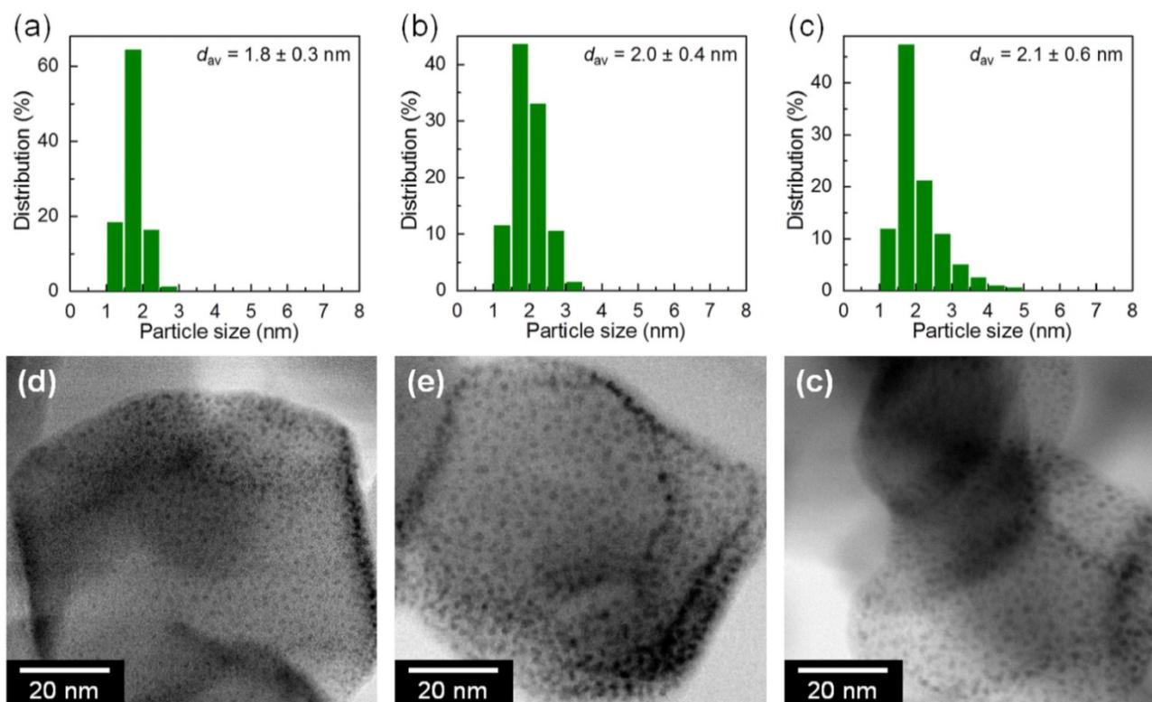
**Fig. S1** Particle-size distributions of (a) Pt/ZIF-8, (b) Pd/ZIF-8, and (c) Ru/ZIF-8. Additional STEM images of (d) Pt/ZIF-8, (e) Pd/ZIF-8, (f) Ru/ZIF-8.
