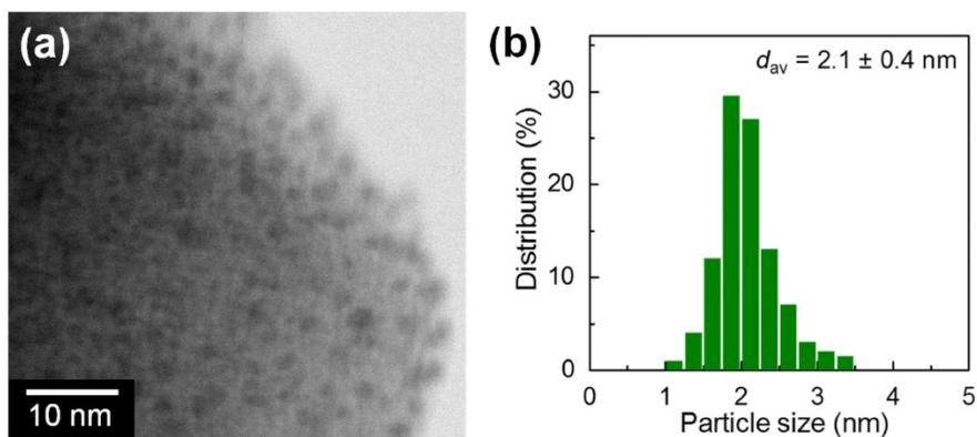
**Fig. S9** (a) STEM image and (b) size distribution of **Pd-PVP/Uio-66-NH<sub>2</sub>**.
