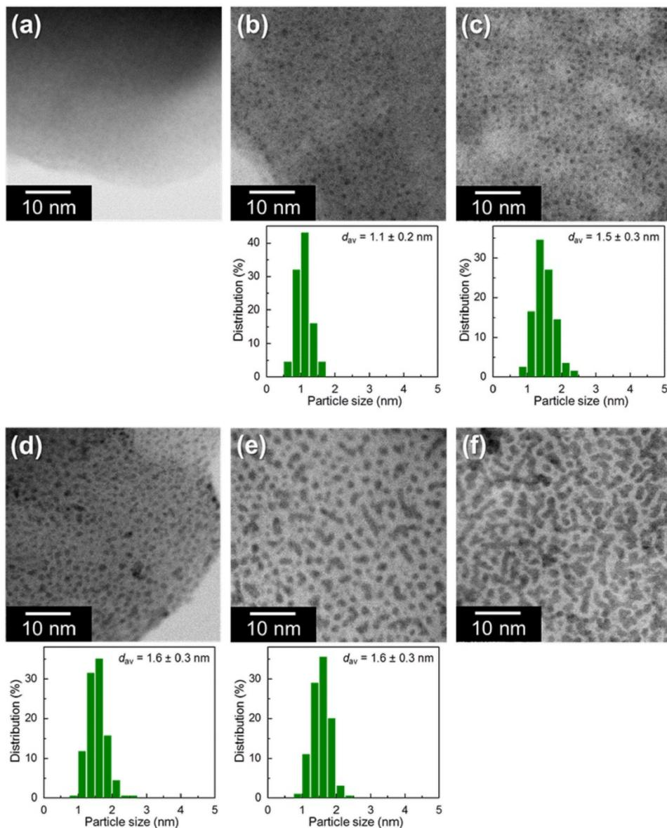
**Fig. S16** Magnified STEM images and size distributions of spherical particles (calculated by counting only the spherical particles, rods or films were not counted) of (a) blank Zn-MOF-74, (b)  $Pt^{12000}/Zn-MOF-74$ , (c)  $Pt^{24000}/Zn-MOF-74$ , (d)  $Pt^{40000}/Zn-MOF-74$ , (e)  $Pt^{70000}/Zn-MOF-74$ , (f)  $Pt^{100000}/Zn-MOF-74$ , prepared at 90 V.
