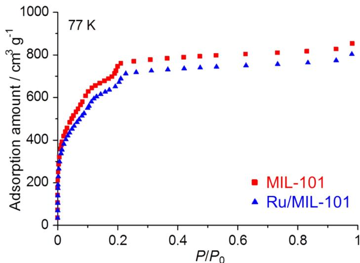
**Fig. S7** N<sub>2</sub> adsorption isotherms of (blue) Ru/MIL-101 and (red) blank MIL-101 at 77 K.
