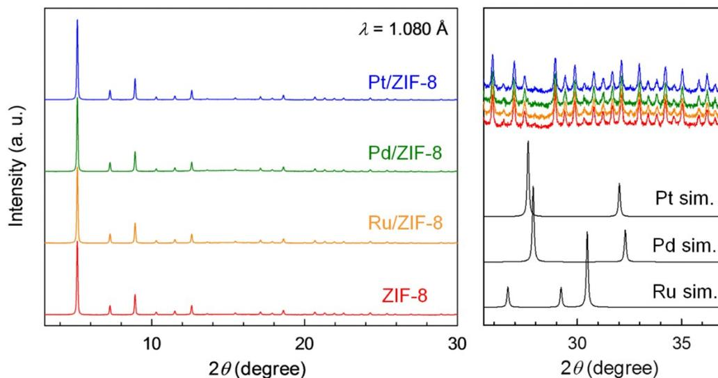
**Fig. S4** (left) XRPD patterns of **Pt/ZIF-8**, **Pd/ZIF-8**, **Ru/ZIF-8**, and blank ZIF-8 at room temperature. (right) Magnified XRPD patterns with simulated patterns of bulk Pt (fcc), Pd (fcc), and Ru (hcp). Blue, green, orange, and red correspond to **Pt/ZIF-8**, **Pd/ZIF-8**, **Ru/ZIF-8**, and blank ZIF-8, respectively.
