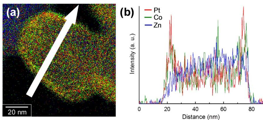
**Fig. S19** (a) STEM-EDS map of **Pt-Co/ZIF-8**. (b) Line profiles along the arrow described in the STEM-EDS map. Red, green, and blue correspond to EDS signals from Pt-M, Co-K, and Zn-K, respectively.
