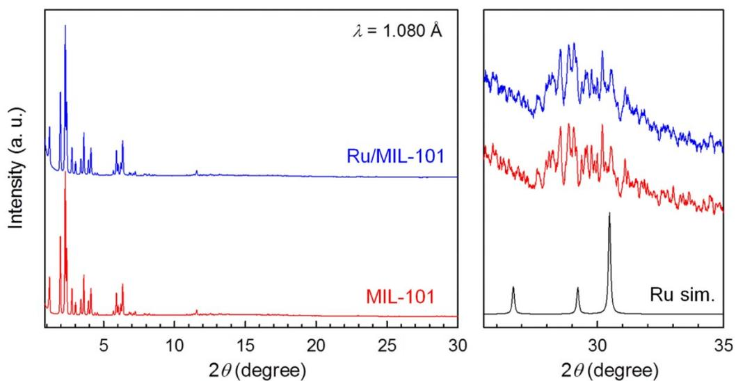
**Fig. S5** (left) XRPD patterns of **Ru/MIL-101**, and blank MIL-101 at room temperature. (right) Magnified XRPD patterns with simulated pattern of bulk Ru (hcp). Blue and red correspond to **Ru/MIL-101** and blank MIL-101, respectively.
