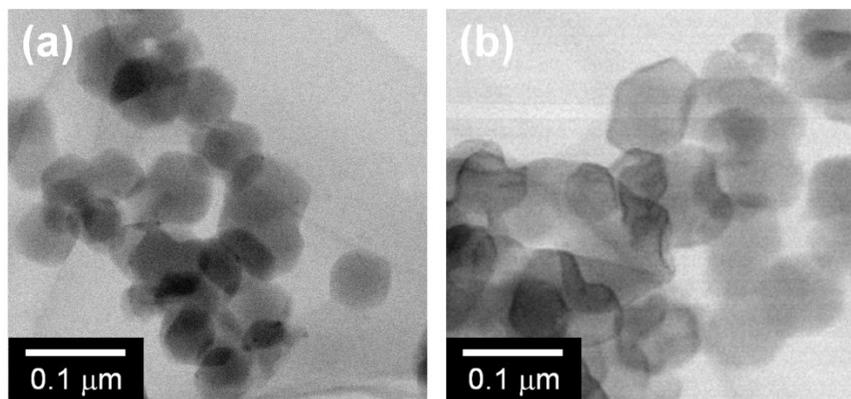
**Fig. S2** STEM images of (a) blank ZIF-8 and (b) **Pt/ZIF-8**. The dark contrast around the ZIF-8 crystal in **Pt/ZIF-8** is due to the deposited Pt, while there are some bare ZIF-8 crystals.
