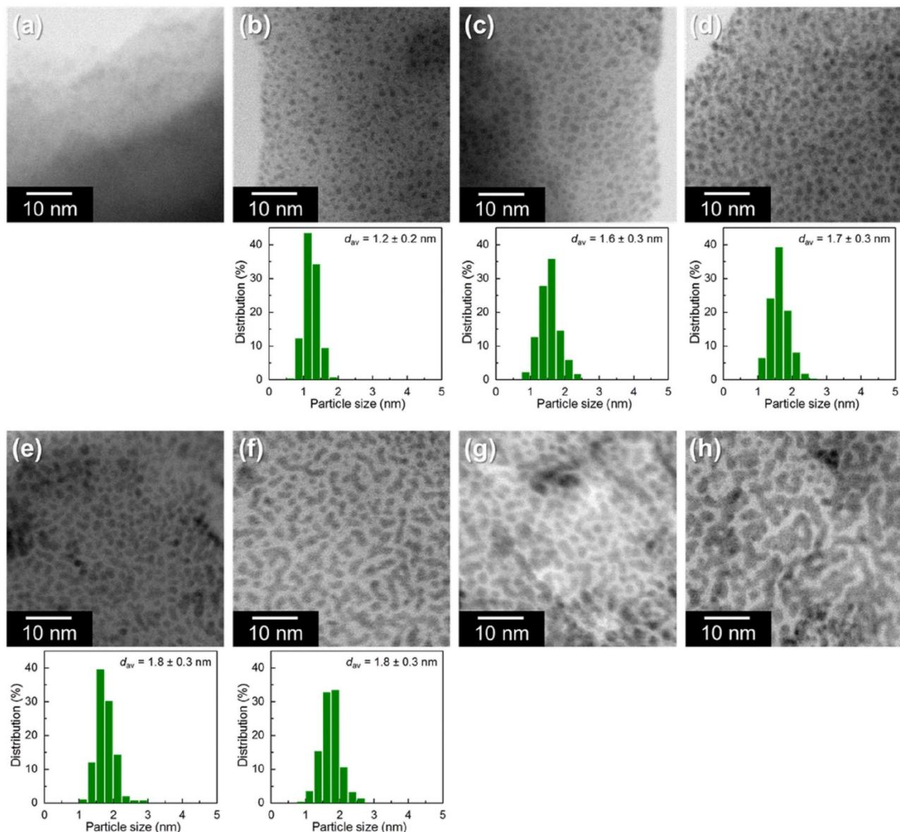
**Fig. S14** Magnified STEM images and size distributions of spherical particles (calculated by counting only the spherical particles, rods or films were not counted) of (a) blank Zn-MOF-74, (b) Pt<sup>4000</sup>/Zn-MOF-74, (c) Pt<sup>8000</sup>/Zn-MOF-74, (d) Pt<sup>12000</sup>/Zn-MOF-74, (e) Pt<sup>18000</sup>/Zn-MOF-74, (f) Pt<sup>24000</sup>/Zn-MOF-74, (g) Pt<sup>30000</sup>/Zn-MOF-74, and (h) Pt<sup>40000</sup>/Zn-MOF-74, prepared at 140 V.
