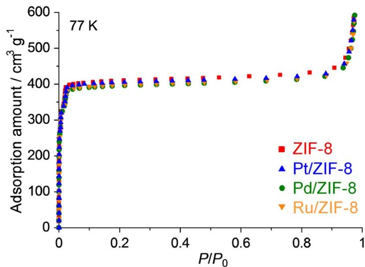
**Fig. S6** N<sub>2</sub> adsorption isotherms of (blue) Pt/ZIF-8, (green) Pd/ZIF-8, (orange) Ru/ZIF-8, and (red) blank ZIF-8 at 77 K.
