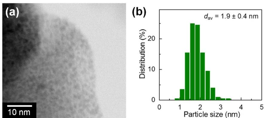
**Fig. S8** (a) STEM image and (b) size distribution of Pd/Uio-66-NH<sub>2</sub>.
