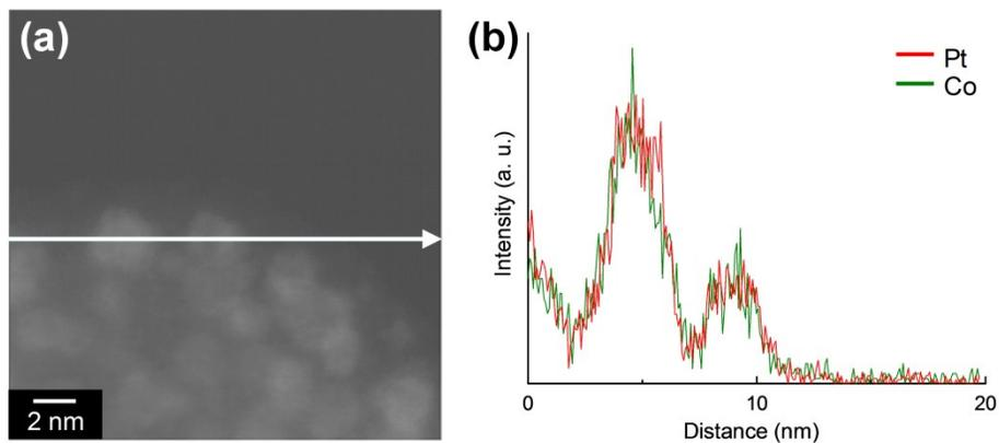
**Fig. S20** (a) A magnified HAADF-STEM image of **Pt-Co/ZIF-8**. (b) Line profile of STEM-EDS analysis along the arrow in the left figure. Green and red correspond to Co-K and Pt-M, respectively.
