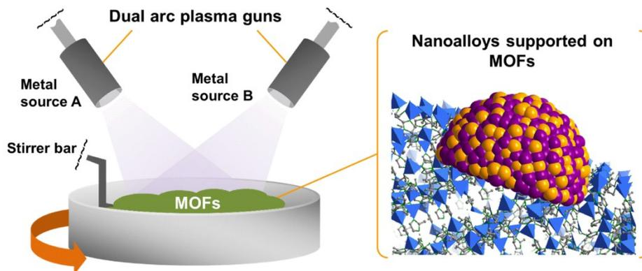
**Fig. S17** Schematic illustration of the experimental settings for alloy synthesis on MOF supports with the APD method.
