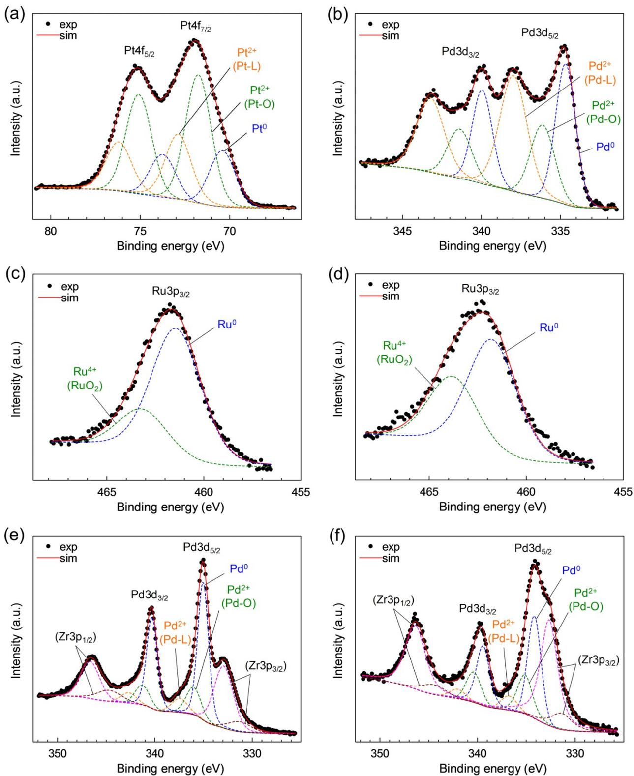
**Fig. S11** XPS spectra of (a) Pt/ZIF-8, (b) Pd/ZIF-8, (c) Ru/ZIF-8, (d) Ru/MIL-101, (e) Pd/UiO-66-NH<sub>2</sub>, and (f) Pd-PVP/UiO-66-NH<sub>2</sub>. (L: ligand)
