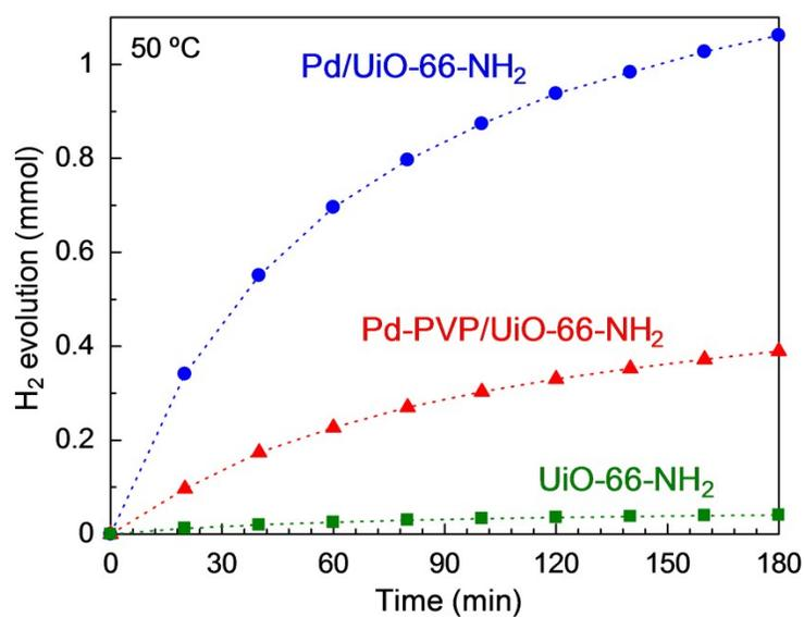
**Fig. S10** H<sub>2</sub> production from formic acid using different catalysts of (blue) **Pd/Uio-66-NH<sub>2</sub>** (50 mg, the amount of Pd is 0.55 mg) prepared through the APD method, (red) **Pd-PVP/Uio-66-NH<sub>2</sub>**, (73 mg, the amount of Pd is 0.60 mg), (green) **Uio-66-NH<sub>2</sub>** (50 mg, no Pd).
