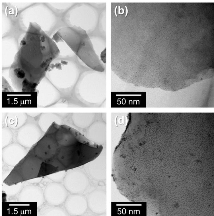
**Fig. S13** STEM images exemplified by (a, b)  $\text{Pt}^{12000}/\text{Zn-MOF-74}$  and (c, d)  $\text{Pt}^{24000}/\text{Zn-MOF-74}$  (prepared at 140 V).
