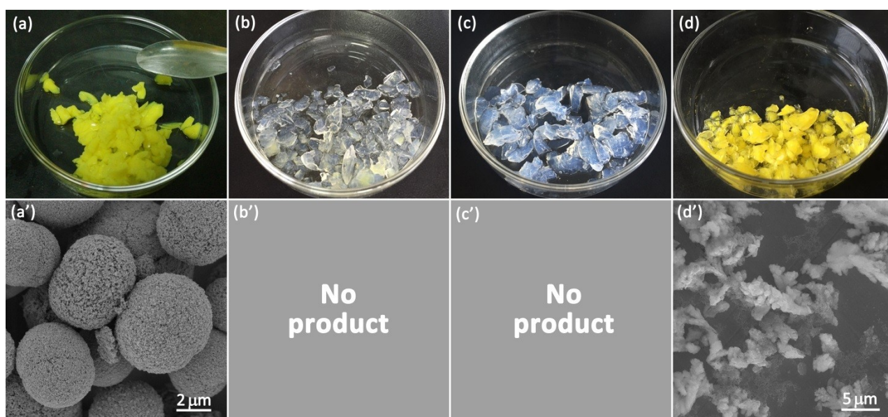
Fig. S7. Photos of silica templates obtained in different control experiments (after hydrothermal treatment): (a) Control experiment 1, (b) Control experiment 2, (c) Control experiment 3, and (d) Control experiment 4. FE-SEM images of the products obtained in different control experiments: (a') Control experiment 1 and (d') Control experiment 4.
