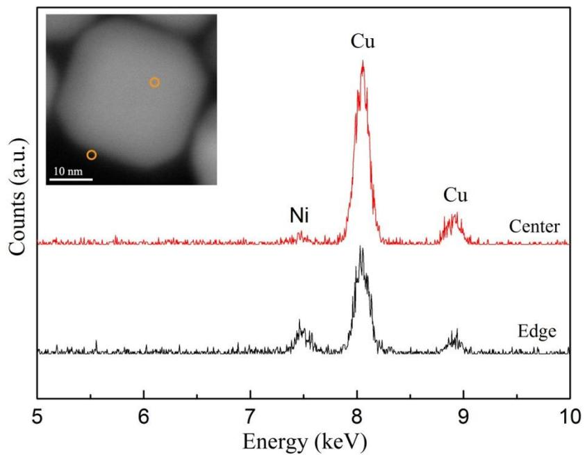
**Fig. S2** EDS analysis on the center and edge of a Cu-Ni core-shell nanocube.
