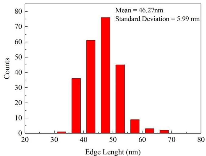
**Fig. S1** Statistic result of the edge length distribution of the typical Cu nanocube seeds.
