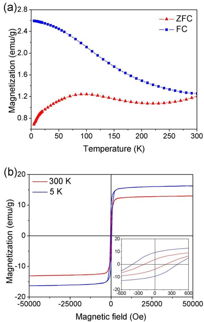
**Fig. 6** ZFC-FC curves obtained in a measuring field and cooling field of 100 Oe (a) and magnetic hysteresis loops (b) of the corn-like Cu-Ni core-shell nanowires.
