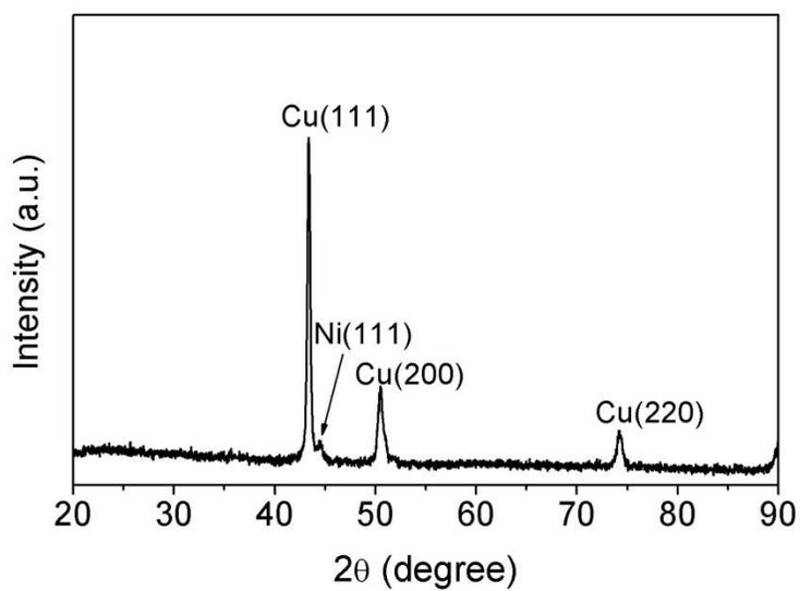
**Fig. S4** XRD pattern of Cu-Ni core-shell nanowires with a corn-like morphology.
