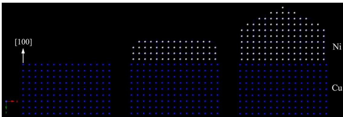
**Fig. S3** Simulated reticular pattern and interface of Cu (blue) and Ni (white).
