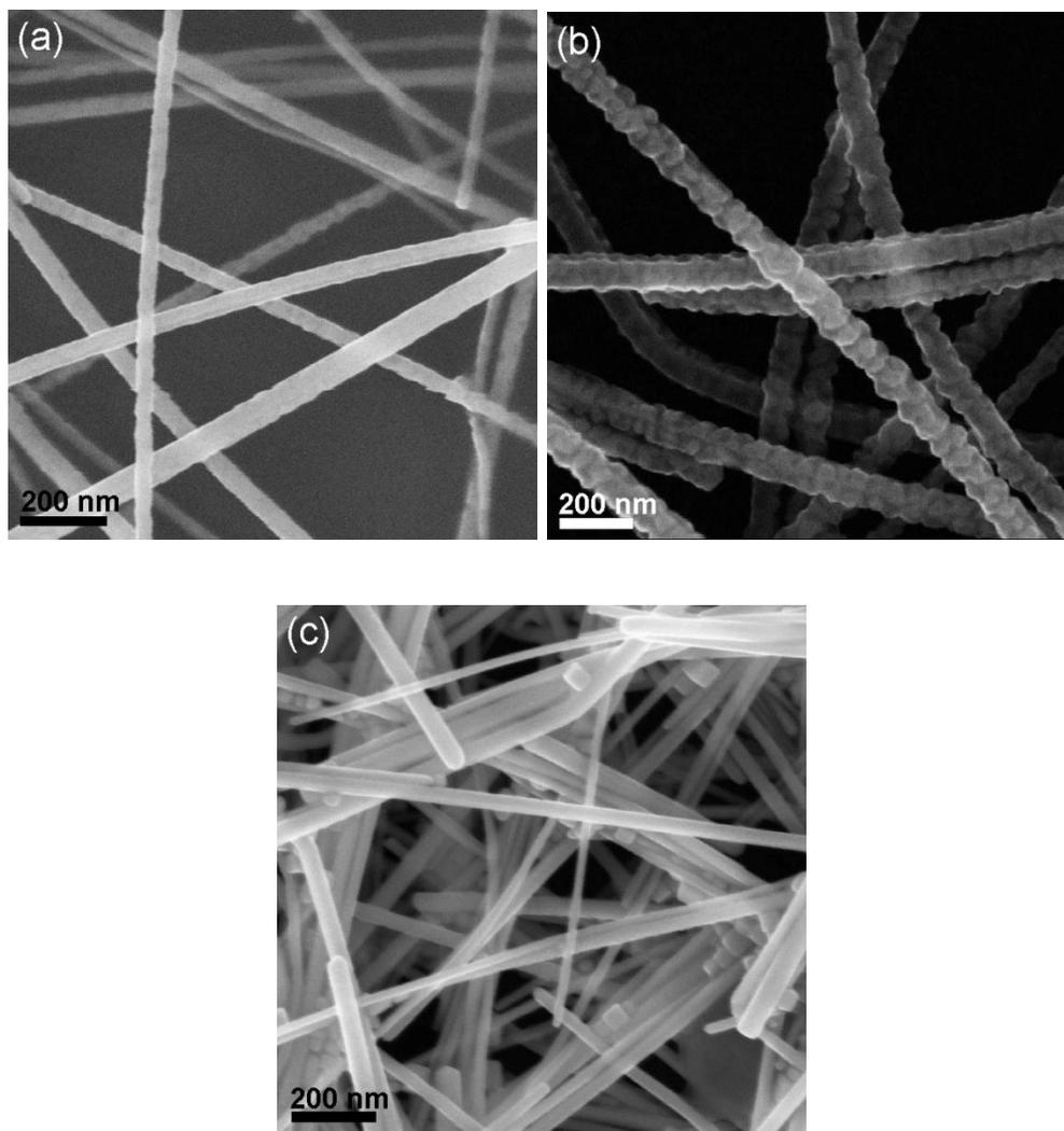
**Fig. 5** SEM images of the Cu-Ni core-shell nanowires synthesized using different stirring speeds.
