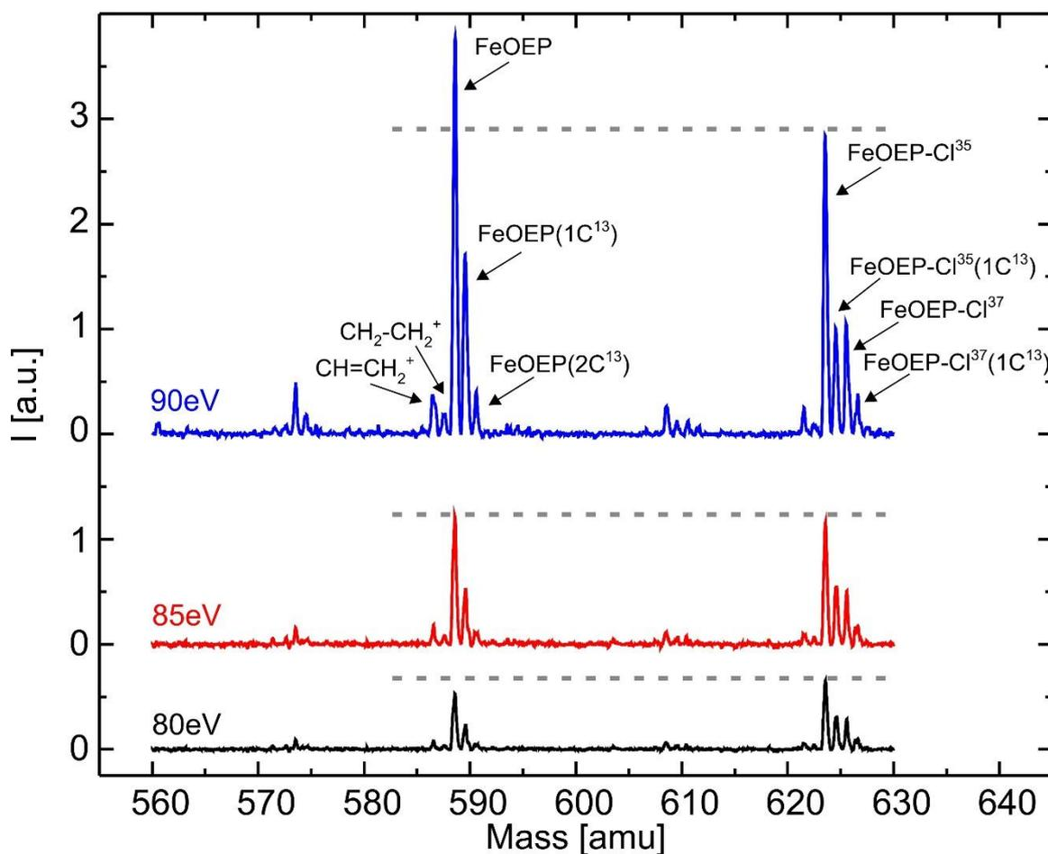
Fig. S 1: QMS data of FeOEP and FeOEP-Cl for different electron energies used for ionization.
