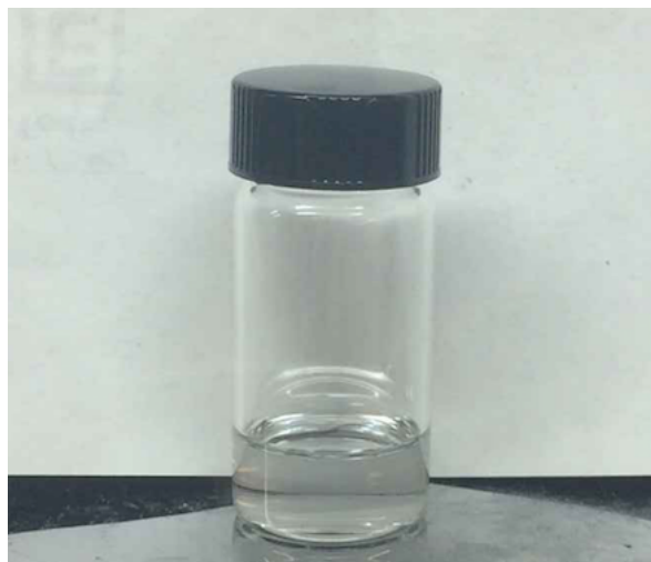
Figure S1. A transparent solution for 0.4 \text{ M NaAlCl}_4 with 0.2 \text{ M } [\text{Mg}_2(\mu\text{-Cl})_2][\text{AlCl}_4]_2 in DME.
