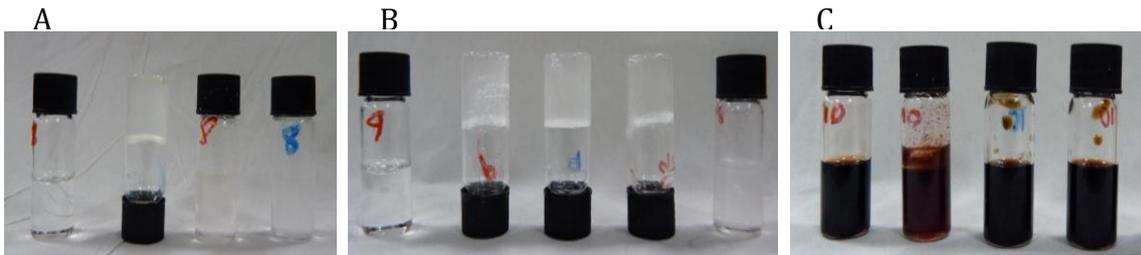
Figure S15. NC gels of A) hydrochlorothiazide, B) 4-aminopyridine and C) 5-aminosalicylic acid.
