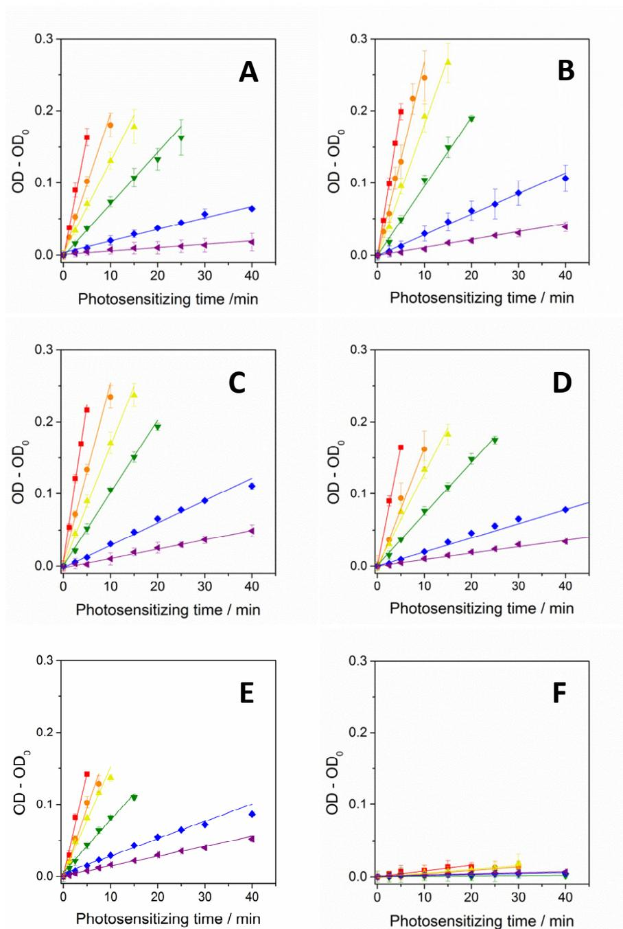
**Figure S1.** Linear parts of the plots in Figure 1 (main text), from which the slopes in Figure 2 and Table 1 are calculated. A) MiniSOG, B) Q103L, C) Q103V, D) W81F, E) FMN, F) EGFP, at different concentrations: 20.0 (red), 10.0 (orange), 6.6 (yellow), 3.3 (green), 1.0 (blue) and 0.5  $\mu$ M (purple)
