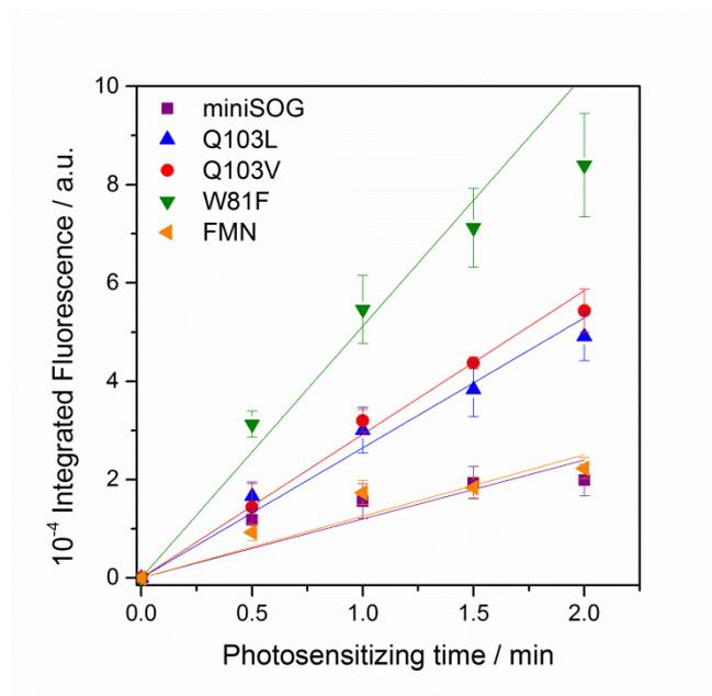
**Figure S5.** Determination of the photosensitization of ROS other than singlet oxygen using the fluorescent probe dihydroethidium.
