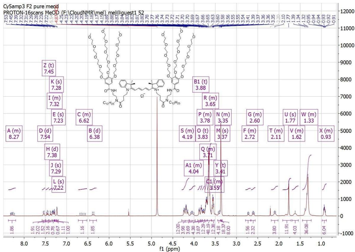
**Figure S29.** <sup>1</sup>H NMR spectrum of compound Cy5A. Partial aggregation of the dye may limit the resolution of this spectrum.
