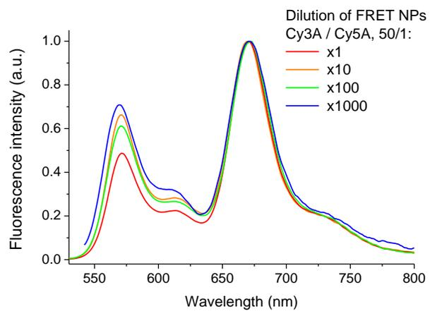
**Figures S6.** Normalized fluorescence spectra of FRET NPs at different dilutions. Initial concentration of Cy3A, Cy5A and F5-TPB in non-diluted (x1) solution were 1, 0.02 and 10  $\mu\text{M}$ , respectively. NPs were diluted to different extent in milliQ water.
