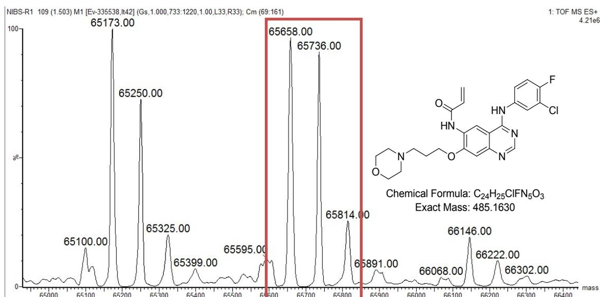
**Figure S5. Characterization of Canertinib-labeled recombinant HER2.** Reaction conditions for probe ligation to the HER2 were as follows: 5  $\mu$ M HER2, 100  $\mu$ M Canertinib, 10 mM MgCl<sub>2</sub>, 1 mM EGTA, 2.5 mM DTT, and 0.5 mM Na<sub>3</sub>VO<sub>4</sub> in HEPES buffer (pH 7.6) at room temperature for 4h. TOF-MS analysis showed the recombinant HER2 could be modified by Canertinib after 4 h incubation at room temperature.
