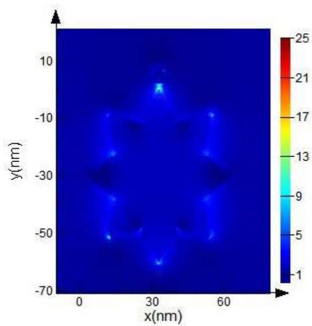
**Fig. S2** FDTD simulation of the normalized EM-field intensity distribution ( $|E|/|E_0|$ ) for single AuNF-single DAuNP model.
