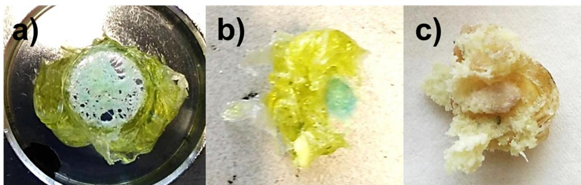
**Figure S4.** Compression of **PU-1** as well as reference polyurethane with solution blended HABI. a) **PU-1** after compression in the pellet press and b) outside the pellet press on white background. c) Compression of solution blended reference polyurethane.
