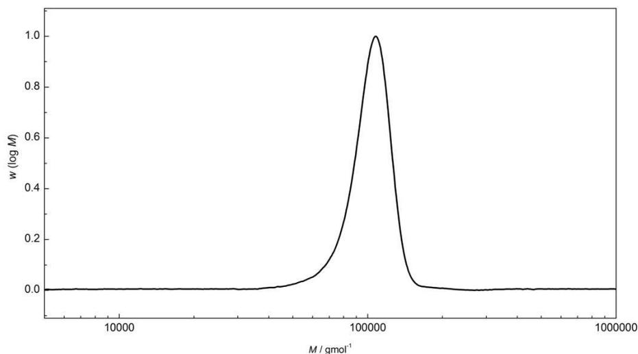
**Figure S1.** Differential molecular weight distribution of GPC RI chromatogram of **PMA-2**.
