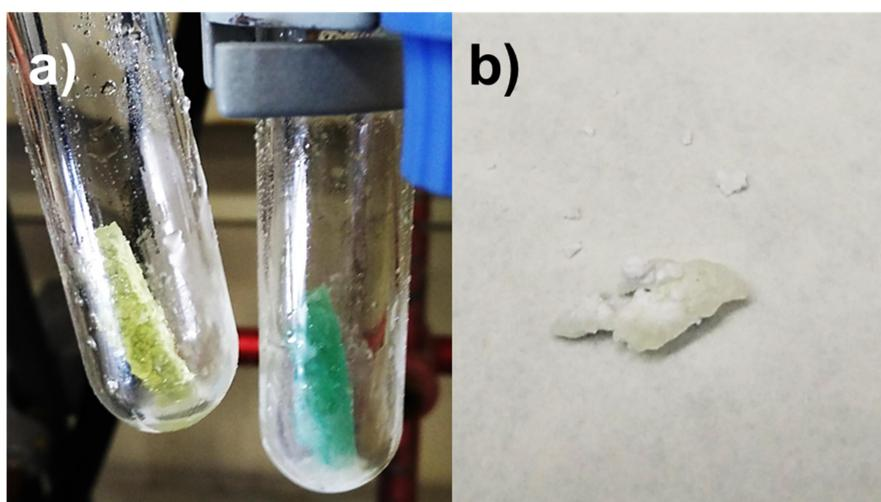
**Figure S5.** a) Freezing of PU-1 swollen in either a 50/50 mol% mixture of ethylene glycol dimethacrylate and 3-mercaptopropionate (left) as well as only in ethylene glycol dimethacrylate (right). b) Solid residue obtained after freezing induced radical polymerization.
