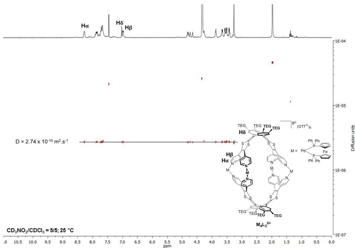
Figure S6.  $^1\text{H}$  DOSY NMR of  $M_4L_2^{8+}$  in  $\text{CDCl}_3/\text{CD}_3\text{NO}_2 = 5/5$  ( $2 \times 10^{-3} \text{ M}$ ).
