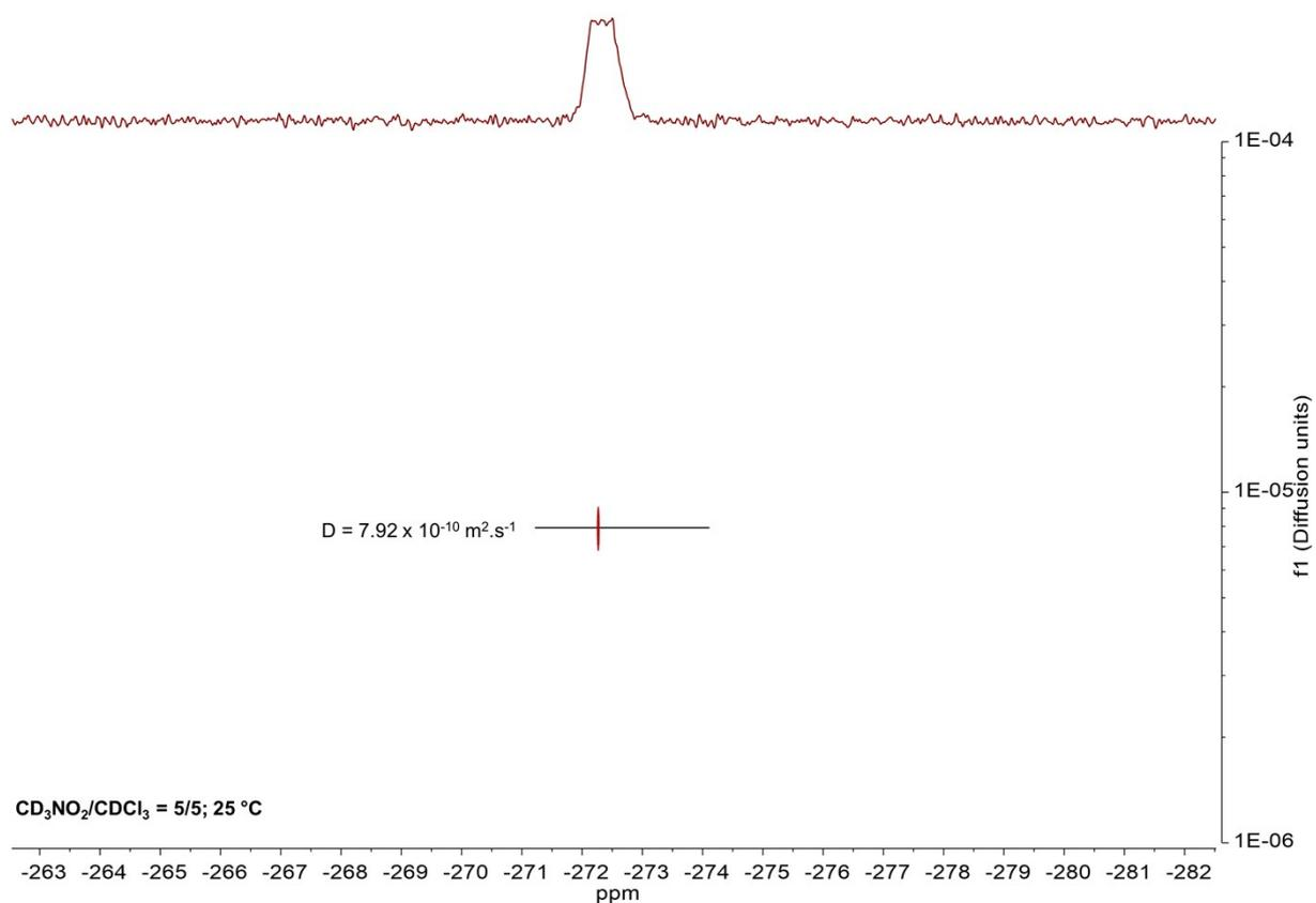
**Figure S29.**  $^{19}\text{F}$  DOSY NMR spectrum of  $\text{TBA}_2 \text{B}_{12}\text{F}_{12}$  in  $\text{CD}_3\text{NO}_2/\text{CDCl}_3 = 1/1$  ( $2 \times 10^{-3} \text{ M}$ ).
