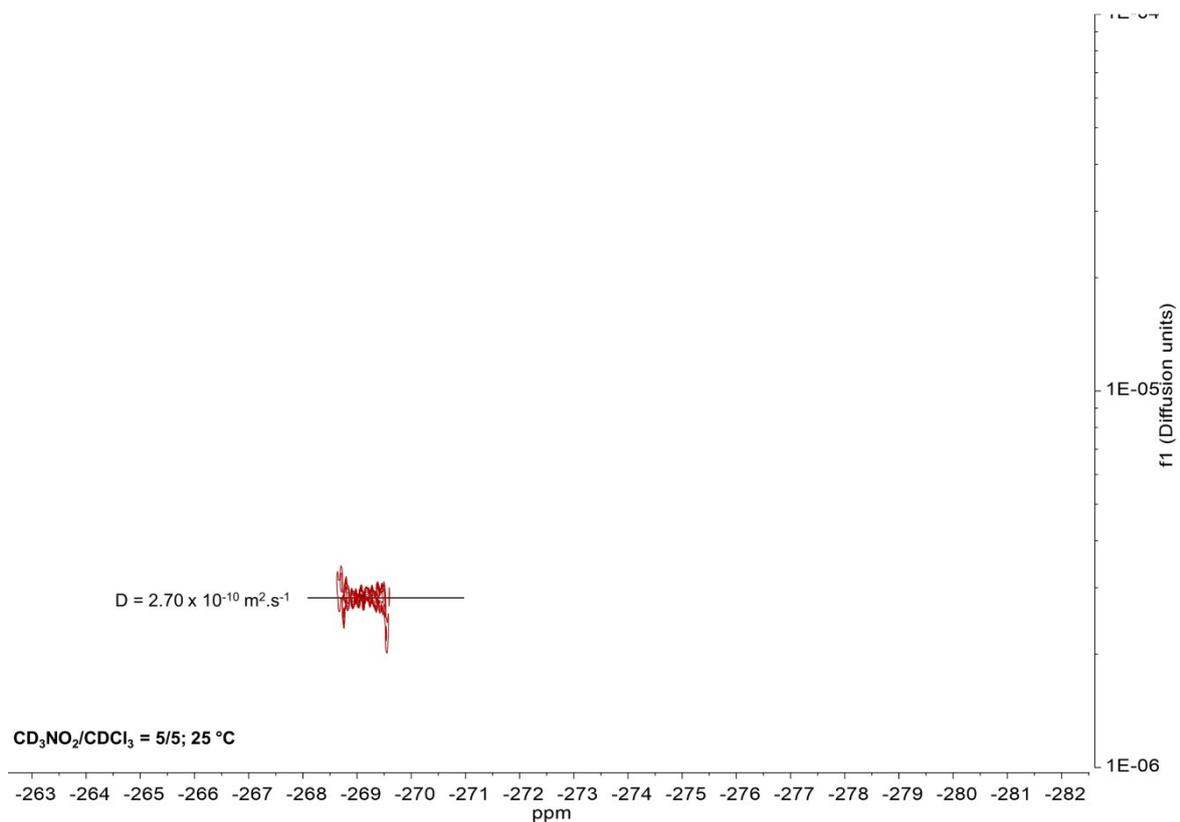
Figure S31.  $^{19}\text{F}$  DOSY NMR spectrum of a stoichiometric mixture of  $\text{TBA}_2\text{B}_{12}\text{F}_{12}$  and  $\text{M}_4\text{L}_2^{8+}(\text{BF}_4^-)_8$  in  $\text{CD}_3\text{NO}_2/\text{CDCl}_3 = 1/1$  ( $2 \times 10^{-3} \text{ M}$ ).
