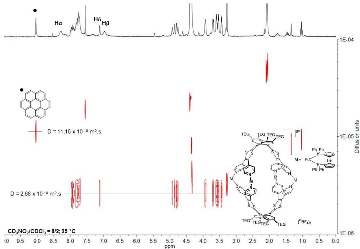
Figure S28.  $^1\text{H}$  DOSY NMR spectrum of a stoichiometric mixture of coronene and  $\text{M}_4\text{L}_2^{8+}(\text{BF}_4)_8$  in  $\text{CD}_3\text{NO}_2/\text{CDCl}_3 = 8/2$  ( $1 \times 10^{-3}$  M).
