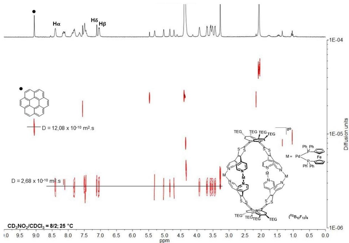
Figure S27.  $^1\text{H}$  DOSY NMR spectrum of a stoichiometric mixture of coronene and  $\text{M}_4\text{L}_2^{8+}(\text{B}_{12}\text{F}_{12}^{2-})_4$  in  $\text{CD}_3\text{NO}_2/\text{CDCl}_3 = 8/2$  ( $1 \times 10^{-3}$  M).
