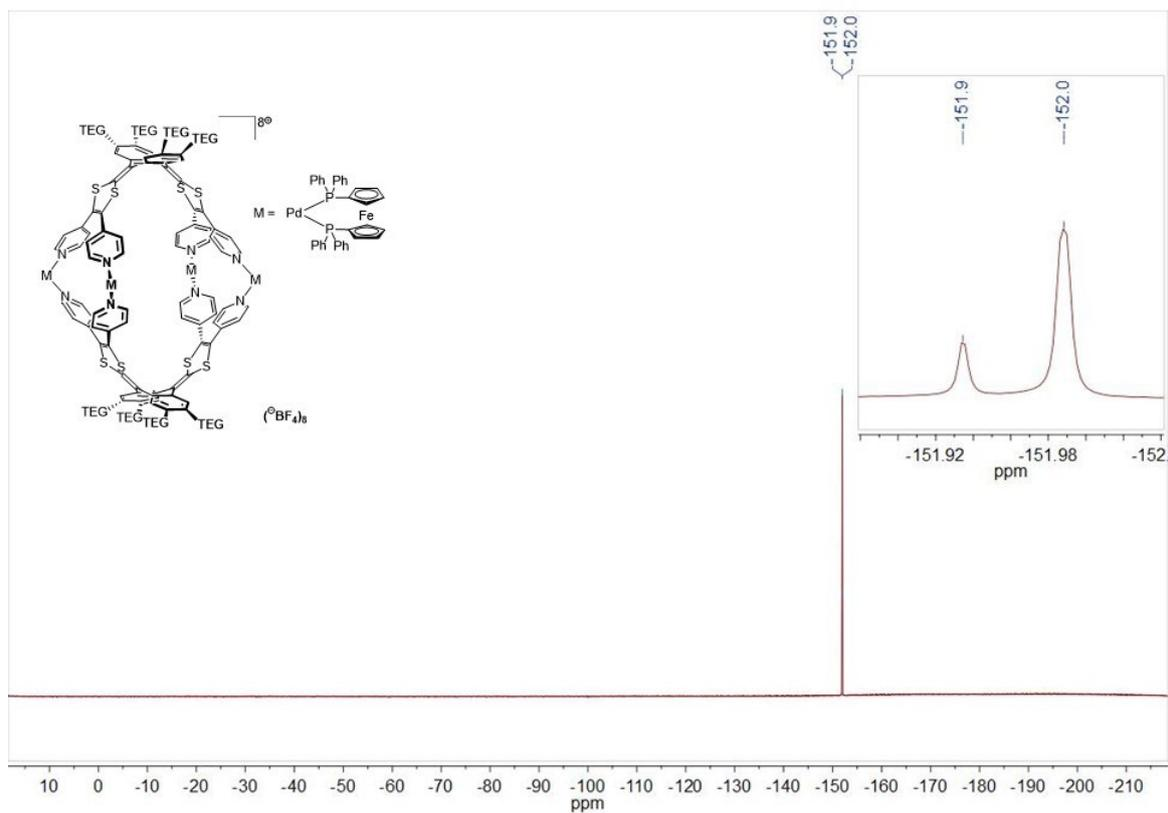
Figure S26.  $^{19}\text{F}$ -NMR spectrum of  $\text{M}_4\text{L}_2^{8+}(\text{BF}_4^-)_8$  in  $\text{CD}_3\text{NO}_2$ .
