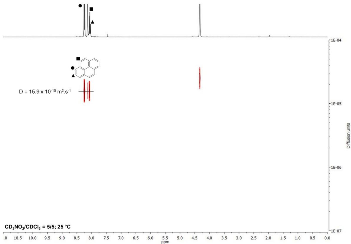
Figure S17.  $^1\text{H}$  DOSY NMR spectrum of pyrene in  $\text{CD}_3\text{NO}_2/\text{CDCl}_3 = 5/5$  ( $2 \times 10^{-3} \text{ M}$ ).
