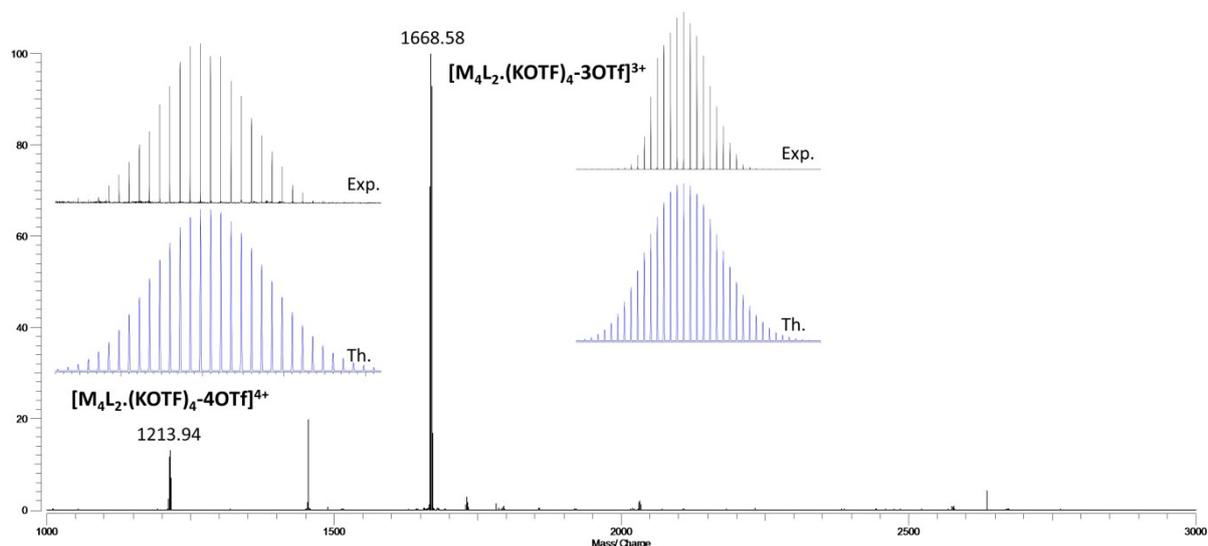
Figure S5. ESI-FTICR spectrum of  $\text{M}_4\text{L}_2 \cdot (\text{KOTf})_4$  recorded in  $\text{CH}_2\text{Cl}_2/\text{CH}_3\text{NO}_2 = 5/5$ .
