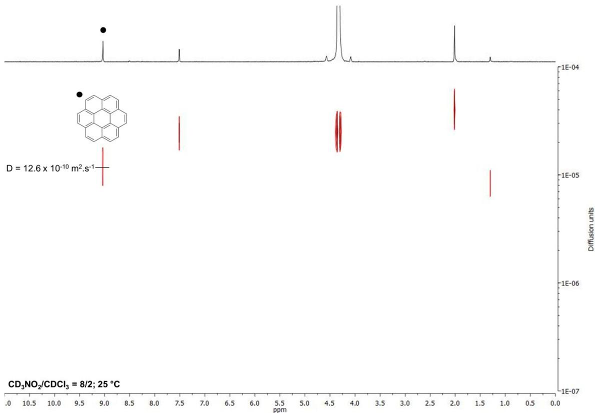
Figure S10.  $^1\text{H}$  DOSY NMR spectrum of coronene in  $\text{CD}_3\text{NO}_2/\text{CDCl}_3 = 8/2$  ( $2 \times 10^{-3} \text{ M}$ ).
