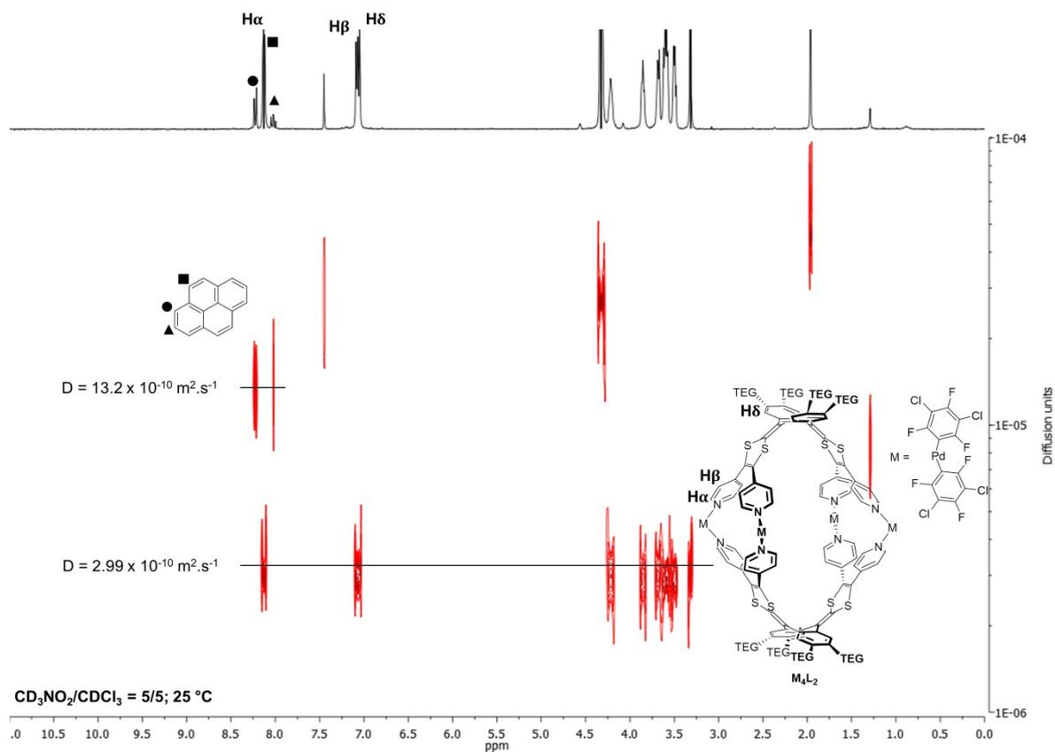
Figure S19.  $^1\text{H}$  DOSY NMR spectrum of a stoichiometric mixture of pyrene and  $\text{M}_4\text{L}_2$  in  $\text{CD}_3\text{NO}_2/\text{CDCl}_3 = 5/5$  ( $2 \times 10^{-3} \text{ M}$ ).
