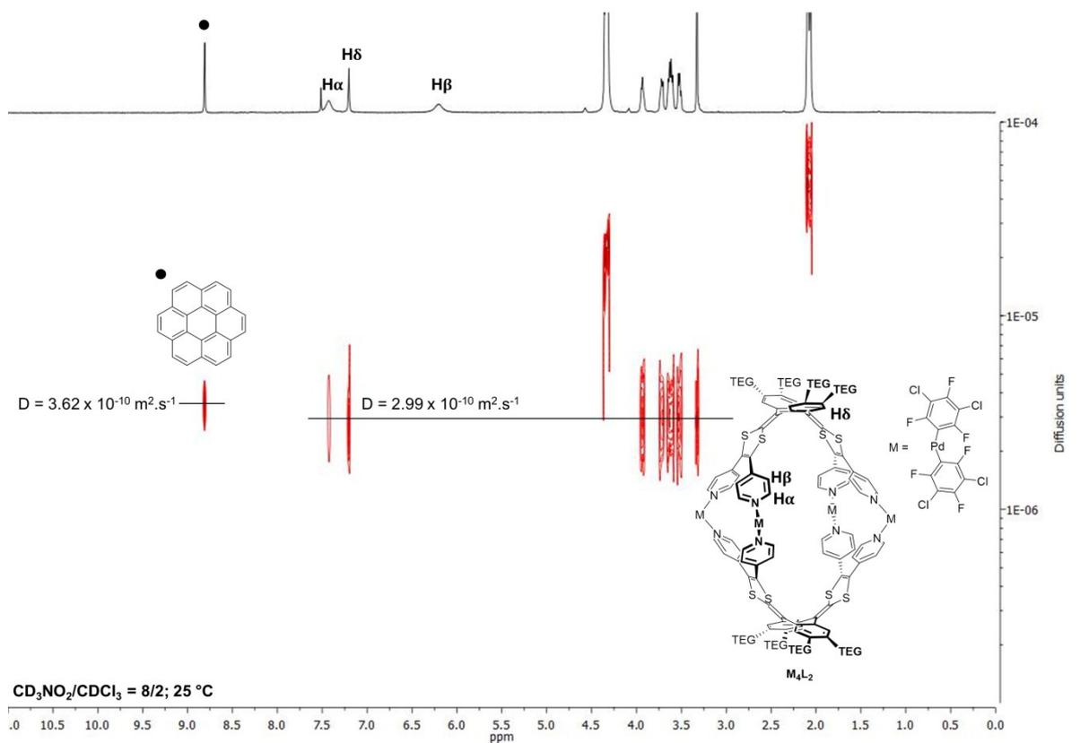
Figure S13.  $^1\text{H}$  DOSY NMR spectrum of a stoichiometric mixture of coronene and  $\text{M}_4\text{L}_2$  in  $\text{CD}_3\text{NO}_2/\text{CDCl}_3 = 8/2$  ( $2 \times 10^{-3}$  M).
