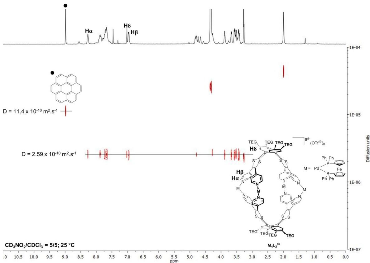
Figure S8.  $^1\text{H}$  DOSY NMR spectrum of a stoichiometric mixture of coronene and  $\text{M}_4\text{L}_2^{8+}$  in  $\text{CD}_3\text{NO}_2/\text{CDCl}_3 = 5/5$  ( $2 \times 10^{-3} \text{ M}$ ).
