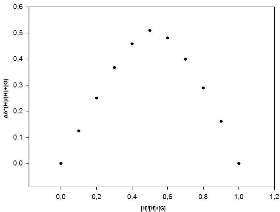
Figure S32. Job plots for complexation of receptor  $\text{M}_4\text{L}_2$  (H) with Coronene (G) determined by  $^1\text{H}$  NMR ( $\text{M}_4\text{L}_2$   $\text{H}_\beta$ ) in  $\text{CDCl}_3/\text{CD}_3\text{NO}_2$  1/1 at 298K,  $[\text{H}] + [\text{G}] = 10^{-3} \text{ mol} \cdot \text{L}^{-1}$ .
