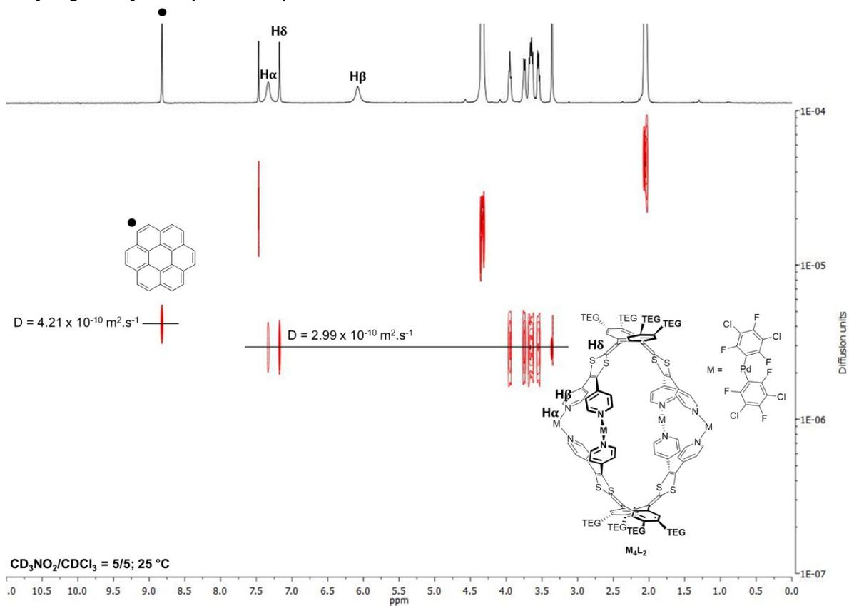
Figure S9.  $^1\text{H}$  DOSY NMR spectrum of a stoichiometric mixture of coronene and  $\text{M}_4\text{L}_2$  in  $\text{CD}_3\text{NO}_2/\text{CDCl}_3 = 5/5$  ( $2 \times 10^{-3} \text{ M}$ ).
