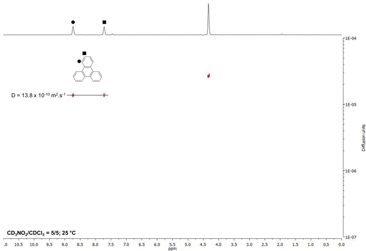
Figure S20.  $^1\text{H}$  DOSY NMR spectrum of triphenylene in  $\text{CD}_3\text{NO}_2/\text{CDCl}_3 = 5/5$  ( $2 \times 10^{-3} \text{ M}$ ).
