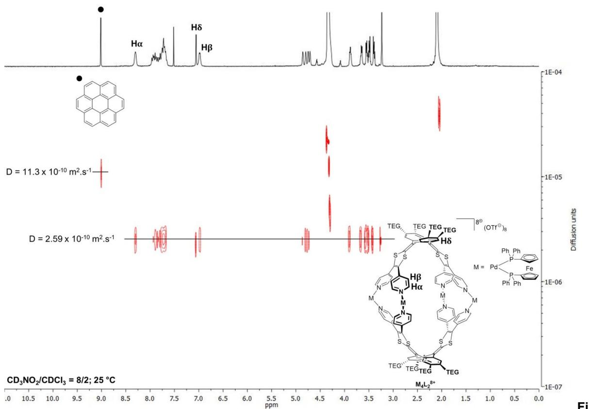
Figure S12.  $^1\text{H}$  DOSY NMR spectrum of a stoichiometric mixture of coronene and  $M_4L_2^{8+}$  in  $\text{CD}_3\text{NO}_2/\text{CDCl}_3 = 8/2$  ( $1 \times 10^{-3} \text{ M}$ ).
