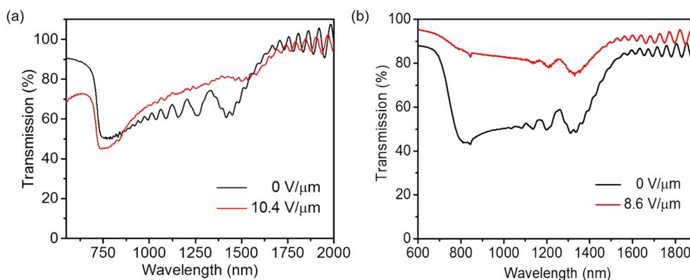
Fig. S1 Transmission spectrum of broadband reflector with (a) 3 wt% and (b) 0.7 wt% of the crosslinker concentration at on and off state (reproduce with permission from Nature Publishing Group).<sup>S1</sup>
