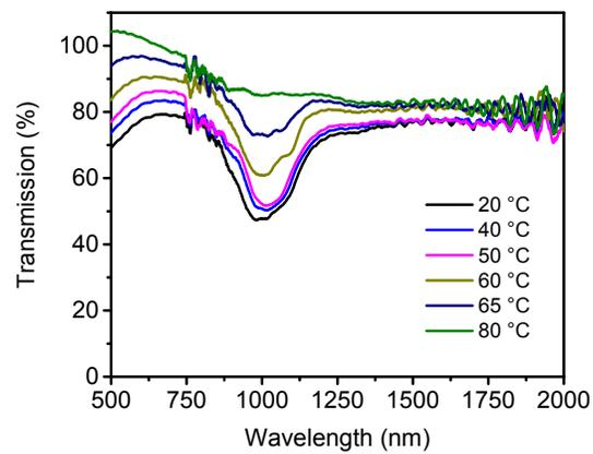
Fig. S3 Temperature dependent transmission spectra of the uniformly distributed polymer stabilized narrowband reflector with 2 wt% crosslinker.
