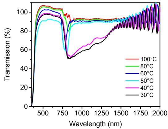
Fig. S2 Transmission spectrum of the 2 wt% broadband reflector on cooling from 100°C to room temperature.
