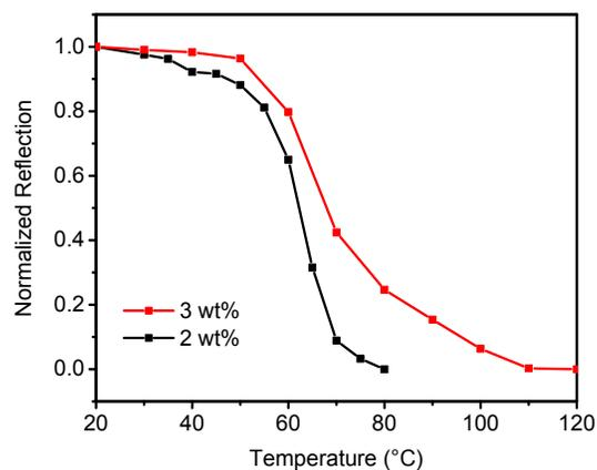
Fig. S4 Temperature dependent normalized reflection of narrowband reflectors with 2 and 3 wt% crosslinker. This graph shows that isotropic transition temperature increases with increase in crosslinker concentration.
