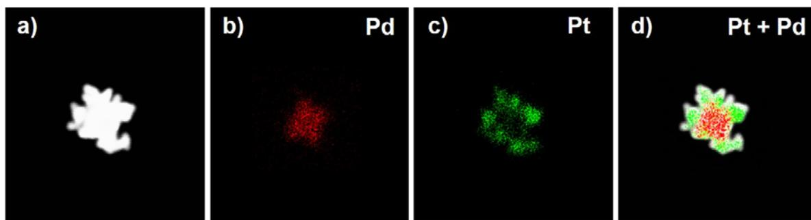
**Figure S12.** Dark-field STEM image (a), and Pt (b), Pd (c), and combined Pd and Pt (d) elemental mapping obtained from an individual octopodal Pd@Pt Nanoparticle prepared using solution with 0.476 mM Pt precursor concentration.
