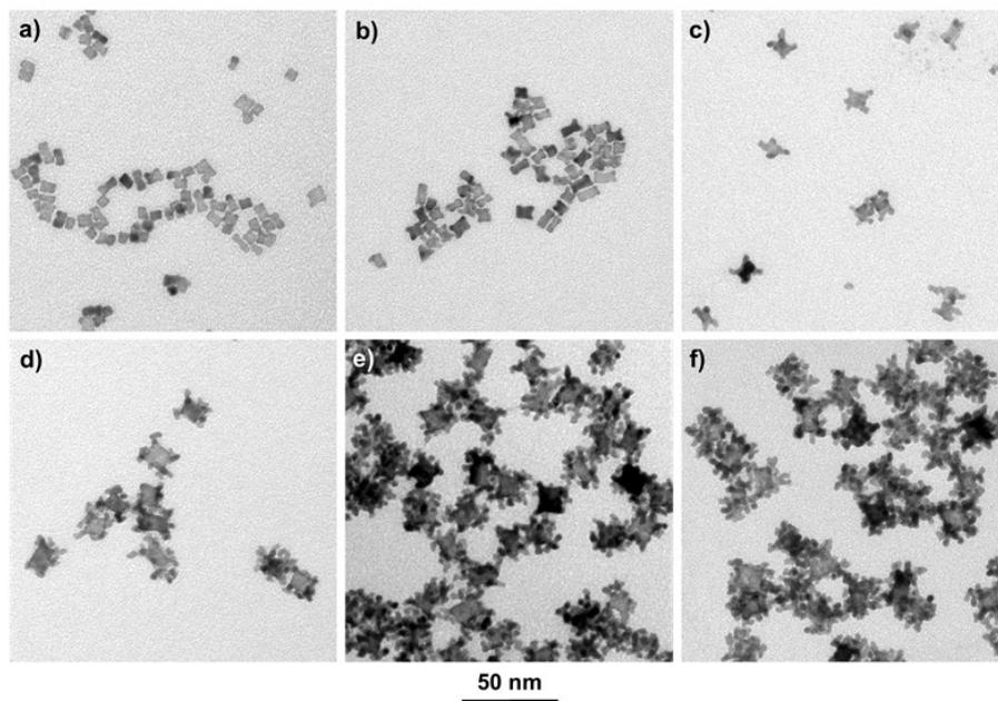
**Figure S11.** TEM images of Pd@Pt nanoparticles prepared using solutions with different Pt concentrations. Pt concentrations are a) 0.079, b) 0.159, c) 0.238, d) 0.317, e) 0.397, and f) 0.476 mM.
