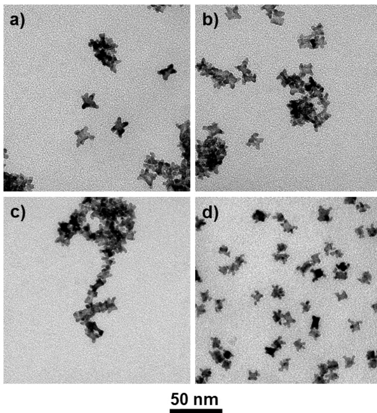
**Figure S7.** TEM images of Pd@Pt nanoparticles prepared using solutions with different amount of F127. Added F127 in reaction solutions are a) 0.35, b) 0.71, c) 11.35, and d) 90.82 mg.
