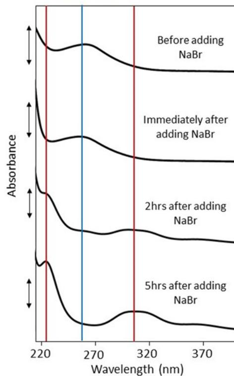
**Figure S3.** UV-Vis spectra of  $\text{H}_2\text{PtCl}_6$  solution before and after adding NaBr. Blue line shows peak position before adding NaBr and red lines show peak positions appeared after adding NaBr. Black double arrows show 0.4 (A.U).
