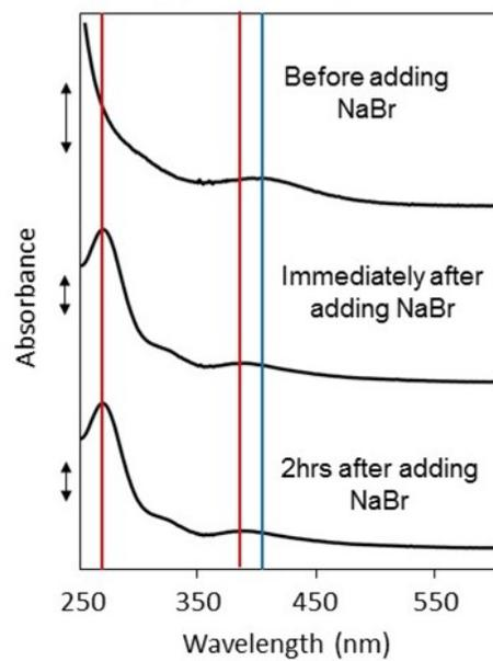
**Figure S2.** UV-Vis spectra of  $\text{H}_2\text{PdCl}_4$  solution before and after adding NaBr. Blue line shows peak position before adding NaBr and red lines show peak positions appeared after adding NaBr. Black double arrows show 0.04 (A.U).
