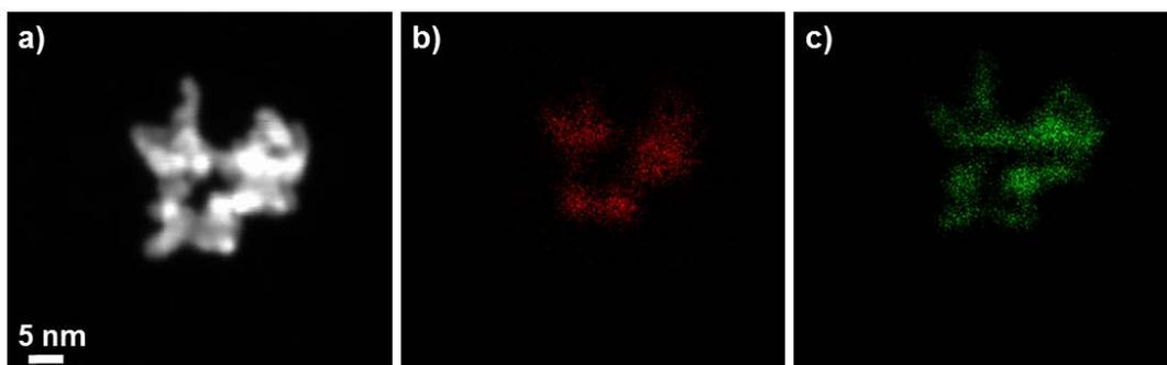
**Figure S8.** Dark-field STEM image (a), and Pt (b), and Pd (c) elemental mapping obtained from Pd@Pt sample prepared using solutions with 0.71 mg F127
