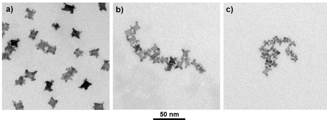
**Figure S10.** TEM images of Pd@Pt nanoparticles prepared using solutions with different total metal ion concentrations. Total metal ions concentrations ( $[\text{Pt}^{4+}] + [\text{Pd}^{2+}]$ ) in reaction solutions are a) 0.24, b) 0.48, and c) 0.96 mM.
