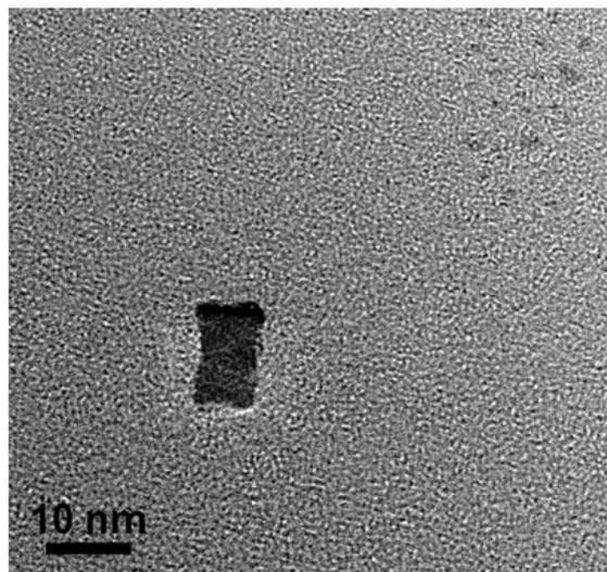
**Figure S4.** TEM image of Pd nanocubes and small Pt particles taken after 1 h of reaction.
