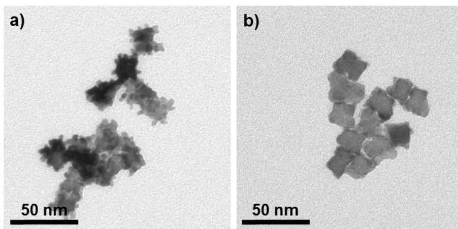
**Figure S13.** TEM images of Pd@Pt nanoparticles prepared using solutions with a) 0.25ml, and b) 1ml HCl (1N).
