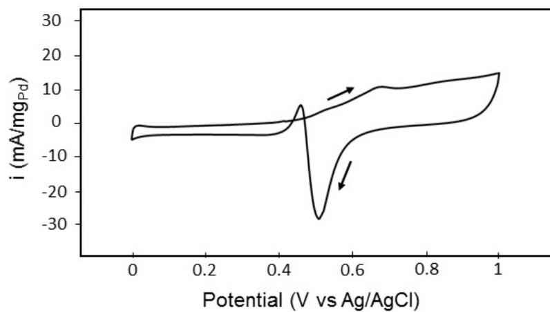
**Figure S14.** Cyclic voltammograms (CVs) of methanol oxidation using Pd cubes. The measured current is normalized to loaded Pt mass.
