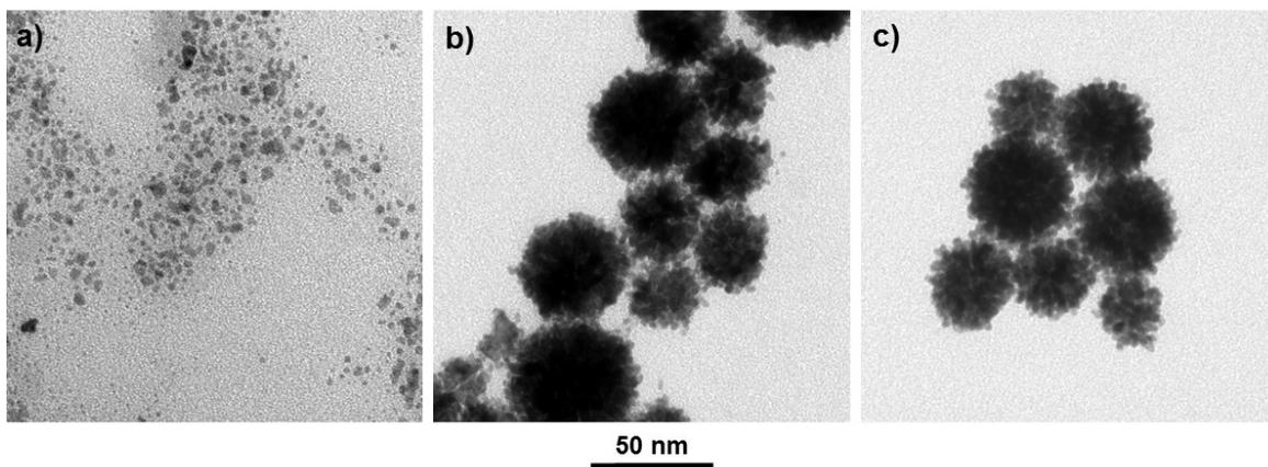
**Figure S6.** TEM images of Pd@Pt nanoparticles prepared using standard procedure, except for replacing NaBr by a) NaI b) NaCl, and c) NaCitrate.
