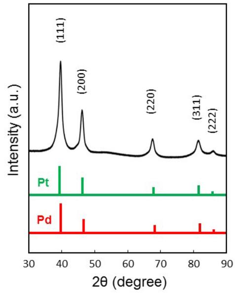
**Figure S1.** Wide-angle XRD profile of octopodal Pd@Pt nanoparticles. Green lines show the fcc Pt phase (JCPDS 04-0802) and red lines show the fcc Pd phase (JCPDS 05-0681).
