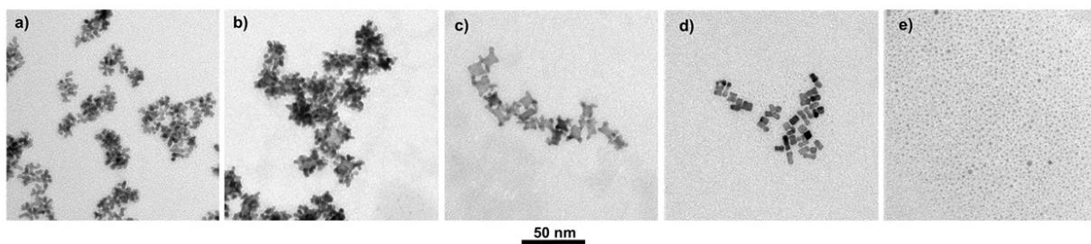
**Figure S9.** TEM images of Pd@Pt nanoparticles prepared using solutions with different Pt:Pd molar ratios. Pt:Pd molar ratios are a) 1:0, b) 3:1, c) 1:1, d) 1:3, and e) 0:1.
