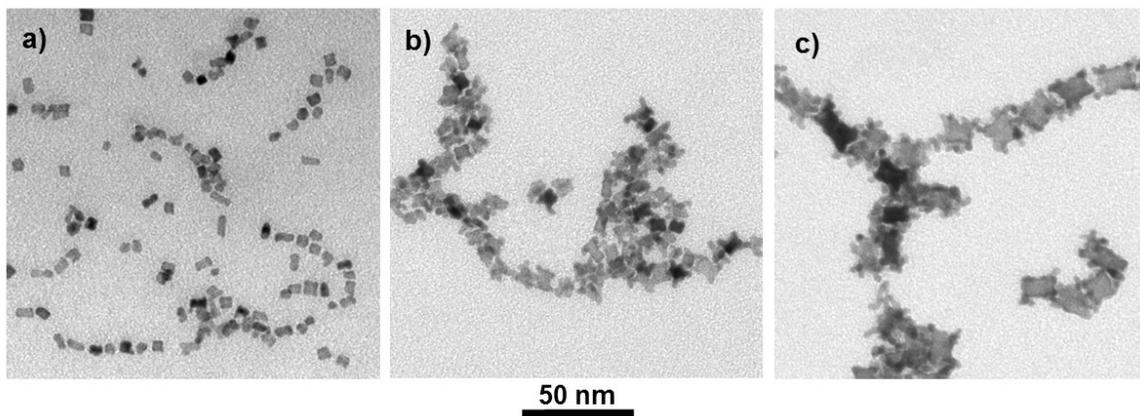
**Figure S5.** TEM images of Pd@Pt nanoparticles prepared using solutions with different NaBr concentrations. NaBr concentrations are a) 3.96, b) 7.93, and c) 23.78 mM.
