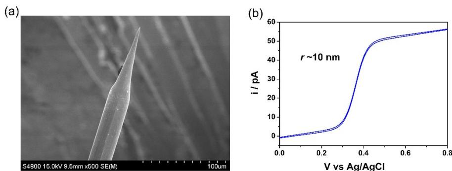
Fig. S1. (a) SEM image of the sharpened Pt wire. (b) The steady-state diffusion-limited current of the Pt disk electrode prior to etching. The radius was estimated to be ~10 nm.
