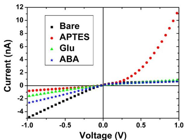
Fig. S4. Monitoring of the modification stages (silica hydroxyl groups ■, amino groups ●,
