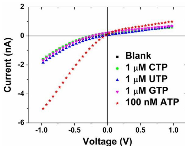
Fig. S7. I-V curves of ABA-modified single glass conical nanopore in 1 mM KCl (pH = 7.4) solution with the addition of 1  $\mu\text{M}$  CTP, 1  $\mu\text{M}$  UTP, 1  $\mu\text{M}$  GTP and 100 nM ATP, respectively. Error bars indicate the standard deviations of three independent measurements.
