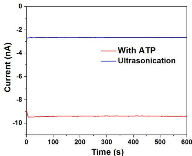
Fig. S8. The current traces at -1V of ABA-modified glass conical nanopore in the presence of ATP and after ultrasonication. The electrolyte is 1 mM KCl PBS buffer (pH = 7.4).
