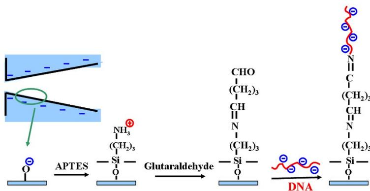
Fig. S2. Schematic description of the covalent modification procedures of glass nanopore surface with DNA strands.
