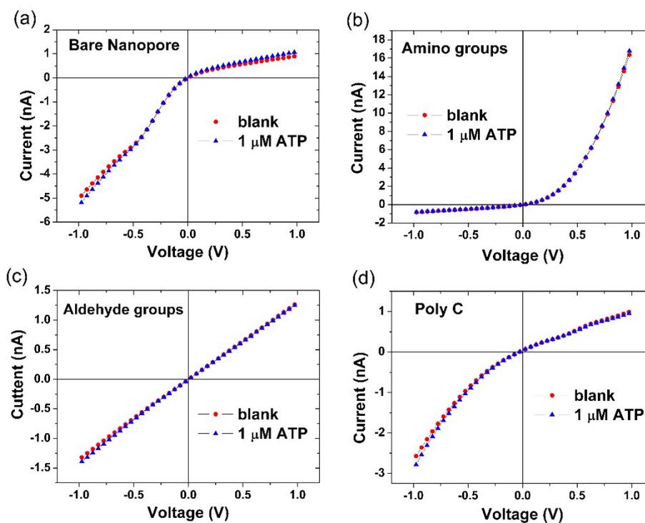
Fig. S6. I-V curves of a single glass conical nanopore in the 1 mM KCl (pH = 7.4) solution prior
