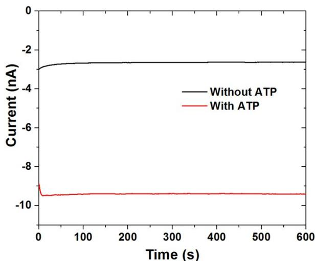
Fig. S5. The current traces at -1V of ABA-modified glass conical nanopore in the absence and presence of ATP. The electrolyte is 1 mM KCl PBS buffer (pH = 7.4).
