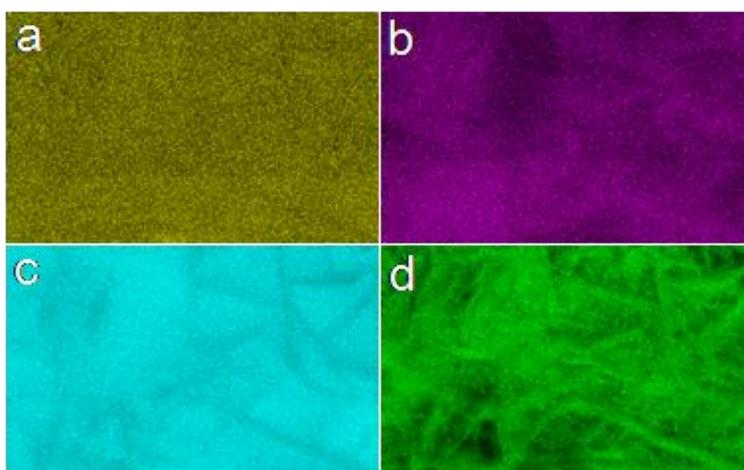
Figure S3. The EDX mapping of SFO-CFO nanocomposites with a ratio of 40:1. a. Co; b. Sr; c. Fe, d. O elements.
