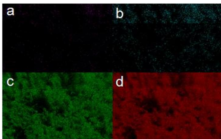
Figure S2. The EDX mapping of SFO-CFO nanocomposites with a ratio of 10:1. a. Co; b. Sr; c. Fe, d. O elements.
