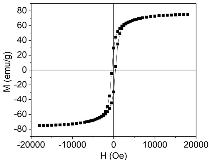
Figure S9. The M-H loop of the sample prepared by annealing the mixture of  $\text{Fe}(\text{acac})_3$  and  $\text{Sr}(\text{acac})_2$  at  $1000\text{ }^\circ\text{C}$  for 4h.
