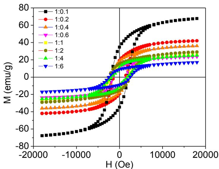
Figure S5. The M-H loops of CFO-SFO nanocomposites with different ratios (CFO:SFO) show the decrease of  $M_s$  and the increase of  $H_c$ , as increasing SFO due to exchange coupling.
