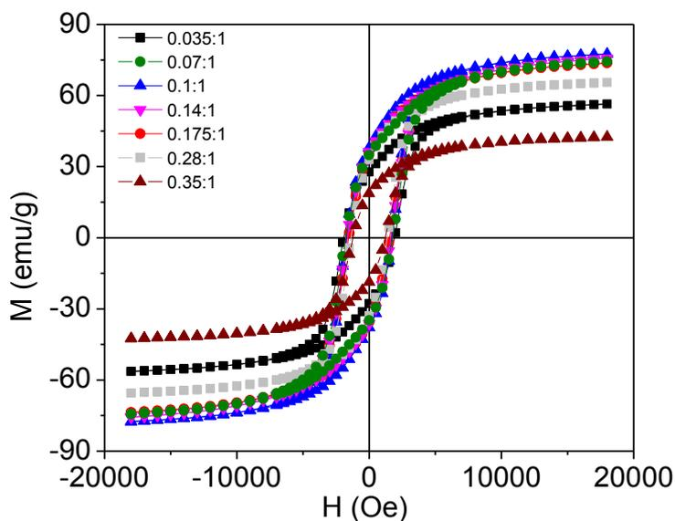
Figure S7. The M-H loops of CFO:SFO nanocomposites with different ratios (SFO:CFO) show the decrease of Ms and the increase of Hc, as increasing SFO due to exchange coupling.
