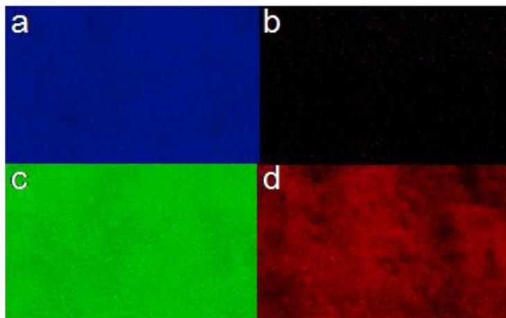
Figure S1. The EDX mapping of SFO-CFO nanocomposites with a ratio of 0.3:1. a. Co; b. Sr; c. Fe, d. O elements.
