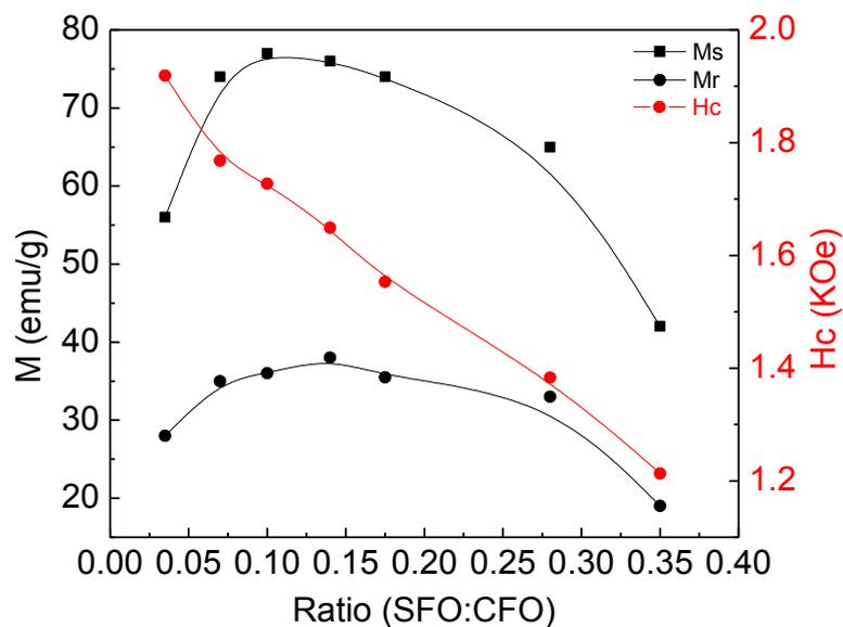
Figure S8. The magnetic characteristics ( $M_s$ ,  $M_r$  and  $H_c$ ) obtained from the M-H loops of CFO:SFO nanocomposites at different composition ratios.
