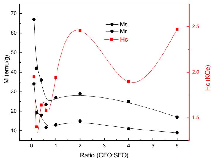
Figure S6. The magnetic characteristics (Ms, Mr and Hc) obtained from the M-H loops of CFO-SFO nanocomposites at different composition ratios.
