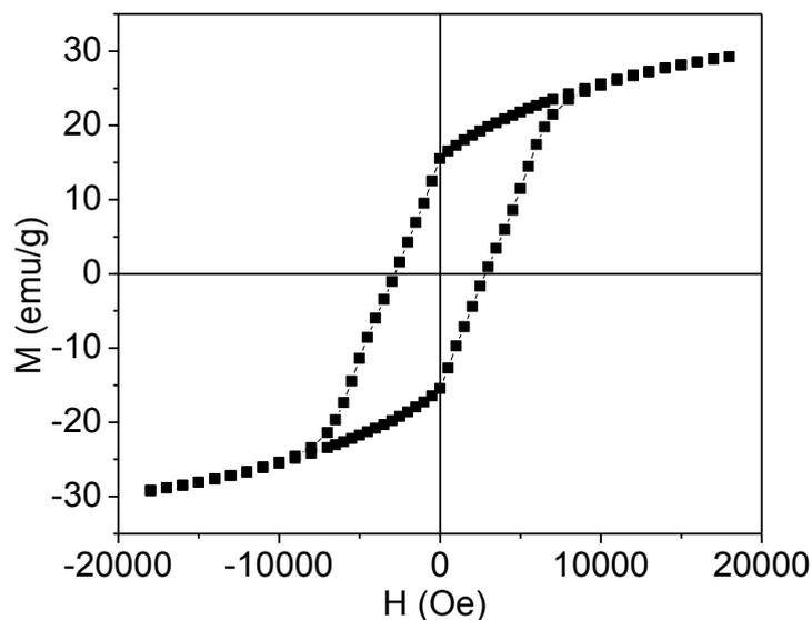
Figure S4. The M-H loop of the mixture between the CFO and SFO nanoparticles, exhibiting the magnetic decoupling behavior.
