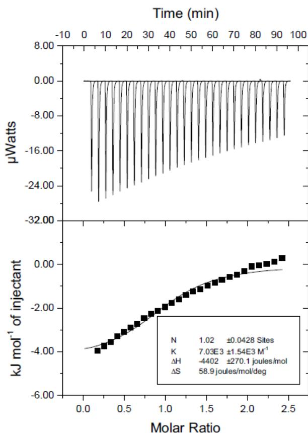
**Fig. S28** Microcalorimetric titration of **AP5** with **G5** in PBS (pH 7.2) at 303.15 K. Top: Raw ITC data for 26 sequential injections (10 μL per injection) of a **G5** solution (20.0 mM) into an **AP5** solution (1.00 mM). Bottom: Net reaction heat obtained from the integration of the calorimetric traces.
