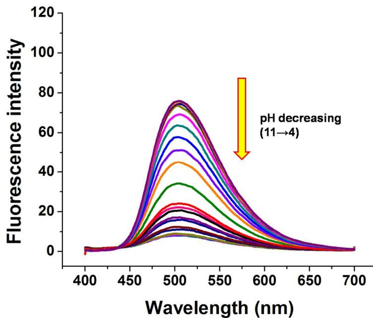
**Fig. S14** Fluorescence titration of a solution of salicylaldehyde ( $5.00 \times 10^{-4}$  M,  $\lambda_{\text{ex}} = 370$  nm,  $\lambda_{\text{em}} = 502$  nm) upon lowering pH in water.
