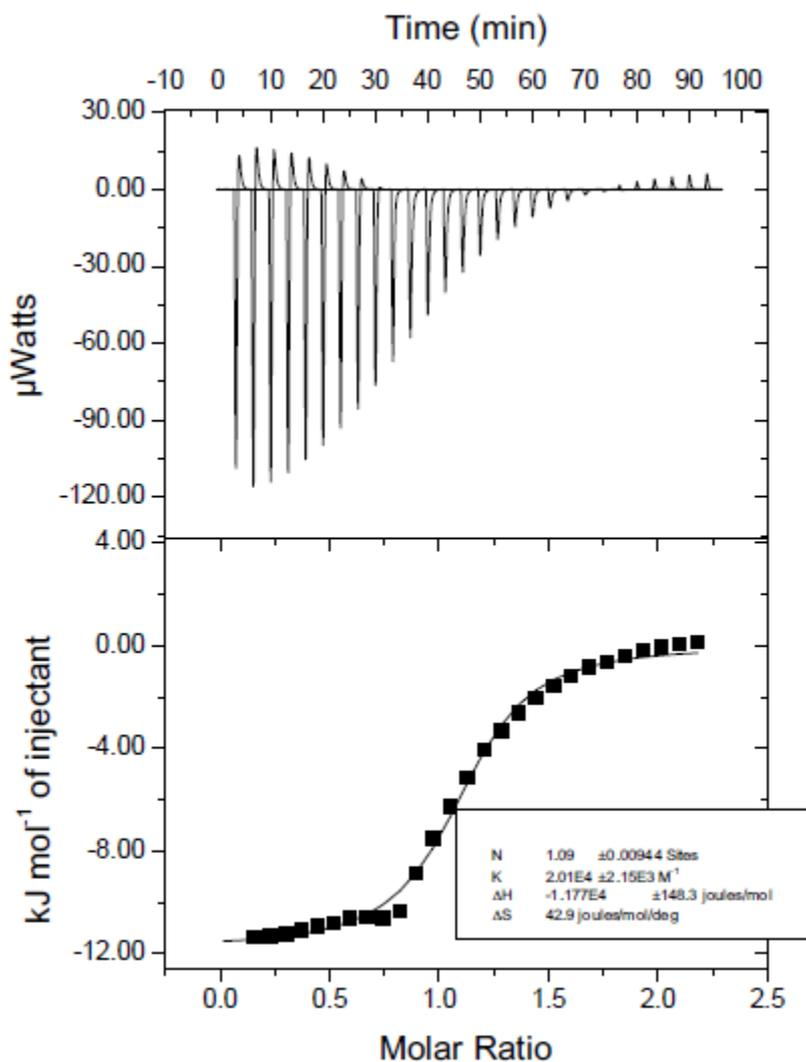
**Fig. S13** Microcalorimetric titration of **AP5** with **SA<sup>-</sup>** in aqueous solution (pH 11) at 303.15 K. Top: Raw ITC data for 26 sequential injections (10 μL per injection) of a **SA<sup>-</sup>** solution (20.0 mM) into an **AP5** solution (1.00 mM). Bottom: Net reaction heat obtained from the integration of the calorimetric traces.
