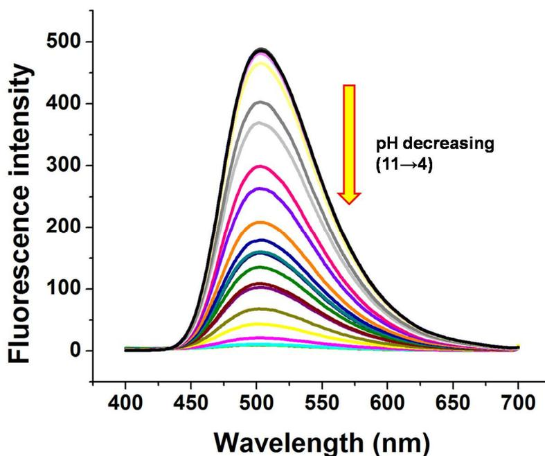
**Fig. S15** Fluorescence titration of a 2:1 mixture of AP5 and salicylaldehyde upon lowering pH in water ( $5.00 \times 10^{-4}$  M salicylaldehyde,  $\lambda_{\text{ex}} = 370$  nm,  $\lambda_{\text{em}} = 502$  nm).
