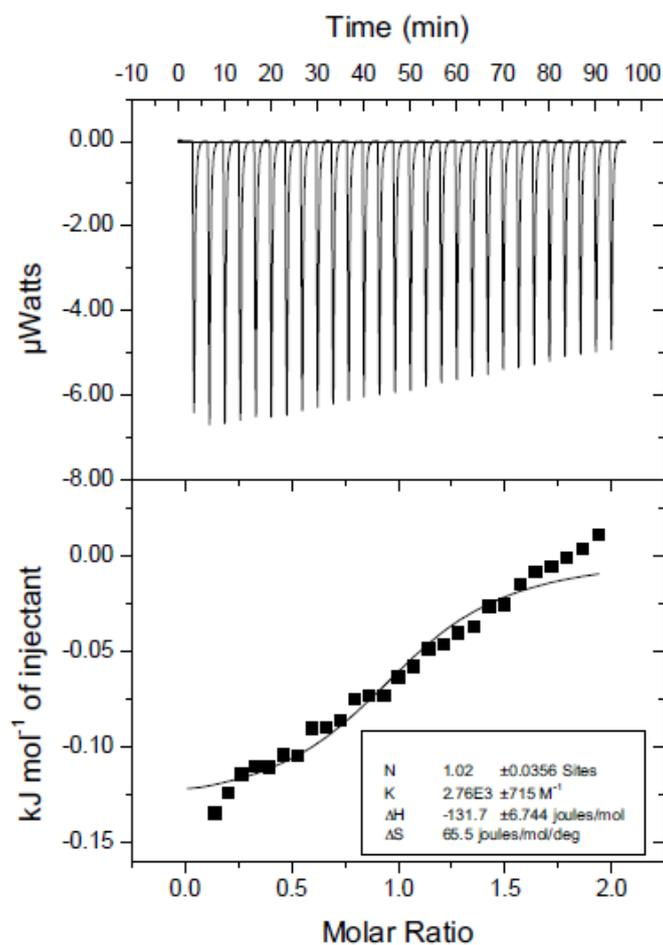
**Fig. S8** Microcalorimetric titration of **AP5** with **SA** in aqueous solution (pH 4) at 303.15 K. Top: Raw ITC data for 26 sequential injections (10  $\mu$ L per injection) of a **SA** solution (20.0 mM) into an **AP5** solution (1.00 mM). Bottom: Net reaction heat obtained from the integration of the calorimetric traces.
