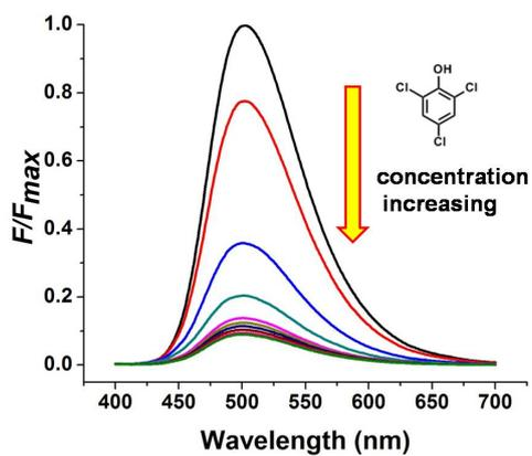
**Fig. S36** Fluorescence titration for the competitive displacement of salicylaldehyde (0.500 mM) from AP5 (1.00 mM) by G6 (0, 0.250, 0.750, 1.50, 2.50, 3.75, 5.00, 6.25, 7.50, and 8.75 mM) in PBS at pH 7.2 ( $\lambda_{\text{ex}} = 370 \text{ nm}$ ,  $\lambda_{\text{em}} = 502 \text{ nm}$ ).
