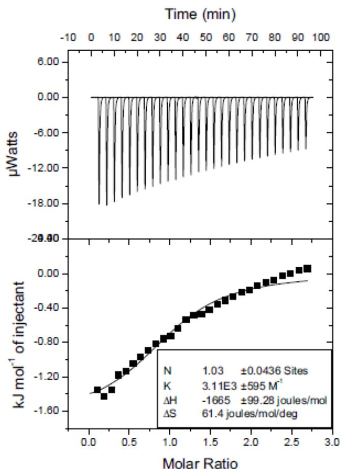
**Fig. S17** Microcalorimetric titration of *AP5* with salicylaldehyde in PBS (pH 7.2) at 303.15 K. (Top) Raw ITC data for 26 sequential injections (10  $\mu\text{L}$  per injection) of a salicylaldehyde-containing solution (20.0 mM) into an *AP5* solution (1.00 mM). (Bottom) Net reaction heat obtained from the integration of the calorimetric traces.
