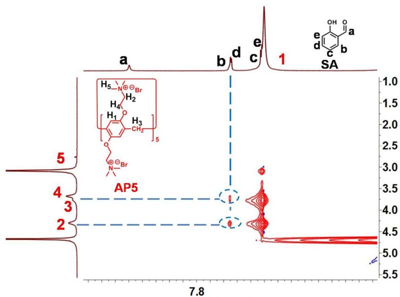
**Fig. S4** Partial NOESY NMR spectrum (500 MHz, D<sub>2</sub>O, room temperature) of SA (10.0 mM) and AP5 (5.00 mM) at pD 4.0.
