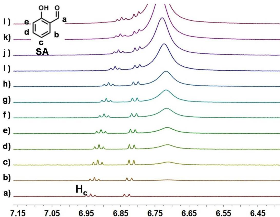
**Fig. S6** Partial <sup>1</sup>H NMR spectra (D<sub>2</sub>O, pD 4.0, 293 K, 400 MHz) of SA at a concentration of 1.00 mM with different concentrations of AP5: a) 0.000 mM, b) 0.200 mM, c) 0.370 mM, d) 0.520 mM, e) 0.670 mM, f) 0.880 mM, g) 1.20 mM, h) 1.61 mM, i) 3.02 mM, j) 4.61 mM, k) 5.70 mM, and l) 6.67 mM.
