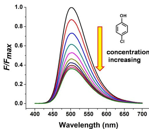
**Fig. S32** Fluorescence titration for the competitive displacement of salicylaldehyde (0.500 mM) from AP5 (1.00 mM) by G2 (0, 0.250, 0.750, 1.50, 2.50, 3.75, 5.00, 6.25, 7.50, and 8.75 mM) in PBS at pH 7.2 ( $\lambda_{\text{ex}} = 370$  nm,  $\lambda_{\text{em}} = 502$  nm).
