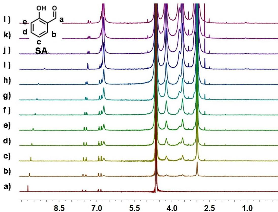
**Fig. S5** <sup>1</sup>H NMR spectra (D<sub>2</sub>O, pD 4.0, 293 K, 400 MHz) of SA at a concentration of 1.00 mM with different concentrations of AP5: a) 0.000 mM, b) 0.200 mM, c) 0.370 mM, d) 0.520 mM, e) 0.670 mM, f) 0.880 mM, g) 1.20 mM, h) 1.61 mM, i) 3.02 mM, j) 4.61 mM, k) 5.70 mM, and l) 6.67 mM.
