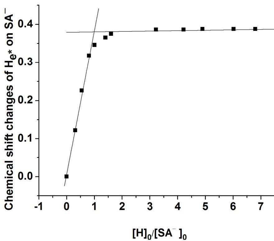
**Fig. S12** Mole ratio plot for the complexation between SA<sup>-</sup> and AP5, indicating a 1:1 stoichiometry.
