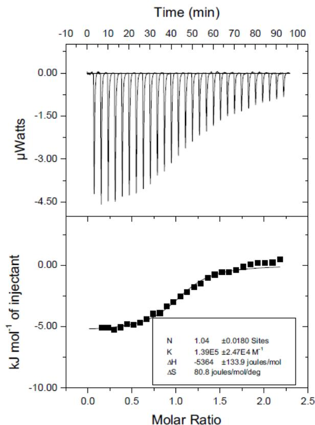
**Fig. S30** Microcalorimetric titration of **AP5** with **G6** in PBS (pH 7.2) at 303.15 K. Top: Raw ITC data for 26 sequential injections (10  $\mu\text{L}$  per injection) of a **G6** solution (20.0 mM) into an **AP5** solution (1.00 mM). Bottom: Net reaction heat obtained from the integration of the calorimetric traces.
