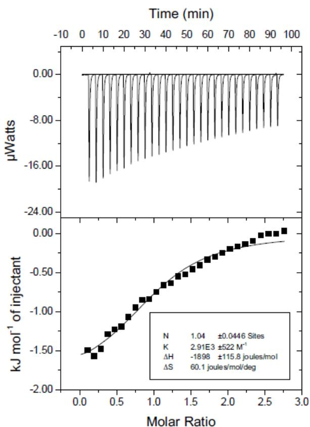
**Fig. S26** Microcalorimetric titration of AP5 with G4 in PBS (pH 7.2) at 303.15 K. Top: Raw ITC data for 26 sequential injections (10  $\mu\text{L}$  per injection) of a G4 solution (20.0 mM) into an AP5 solution (1.00 mM). Bottom: Net reaction heat obtained from the integration of the calorimetric traces.
