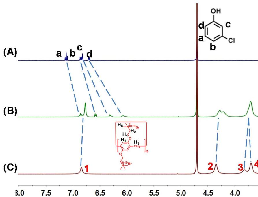
**Fig. S23**  $^1\text{H}$  NMR spectra (400 MHz,  $\text{D}_2\text{O}$ , 293 K): (A) **G3** (4.00 mM); (B) **G3** (4.00 mM) and **AP5** (2.00 mM); (C) **AP5** (2.00 mM).
