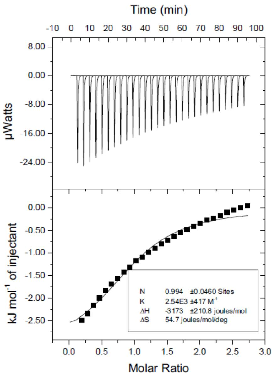
**Fig. S22** Microcalorimetric titration of **AP5** with **G2** in PBS (pH 7.2) at 303.15 K. Top: Raw ITC data for 26 sequential injections (10  $\mu$ L per injection) of a **G2** solution (20.0 mM) into an **AP5** solution (1.00 mM). Bottom: Net reaction heat obtained from the integration of the calorimetric traces.
