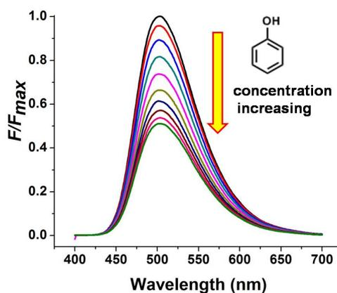
**Fig. S31** Fluorescence titration for the competitive displacement of salicylaldehyde (0.500 mM) from AP5 (1.00 mM) by G1 (0, 0.250, 0.750, 1.50, 2.50, 3.75, 5.00, 6.25, 7.50, and 8.75 mM) in PBS at pH 7.2 ( $\lambda_{\text{ex}} = 370$  nm,  $\lambda_{\text{em}} = 502$  nm).
