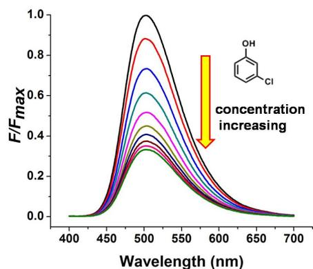
**Fig. S33** Fluorescence titration for the competitive displacement of salicylaldehyde (0.500 mM) from AP5 (1.00 mM) by **G3** (0, 0.250, 0.750, 1.50, 2.50, 3.75, 5.00, 6.25, 7.50, and 8.75 mM) in PBS at pH 7.2 ( $\lambda_{\text{ex}} = 370 \text{ nm}$ ,  $\lambda_{\text{em}} = 502 \text{ nm}$ ).
