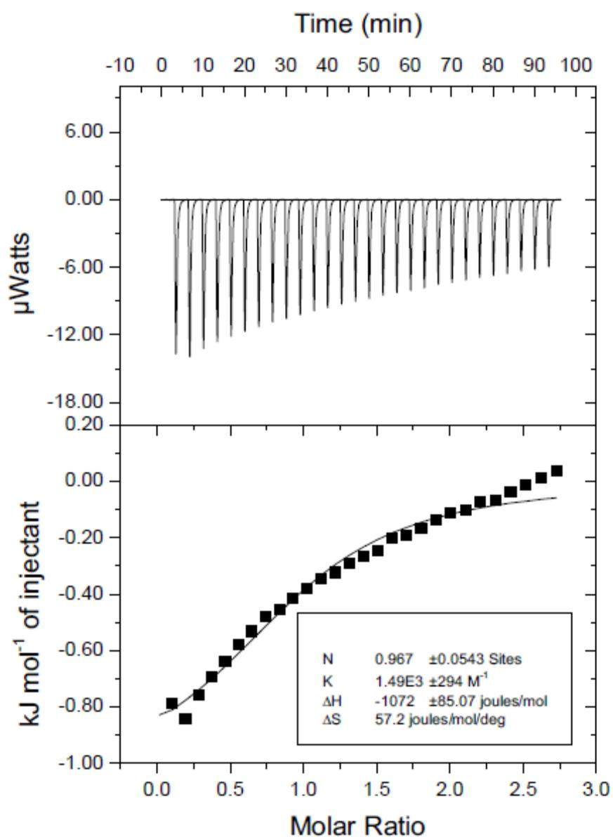
**Fig. S20** Microcalorimetric titration of **AP5** with **G1** in PBS (pH 7.2) at 303.15 K. Top: Raw ITC data for 26 sequential injections (10  $\mu$ L per injection) of a **G1** solution (20.0 mM) into an **AP5** solution (1.00 mM). Bottom: Net reaction heat obtained from the integration of the calorimetric traces.
