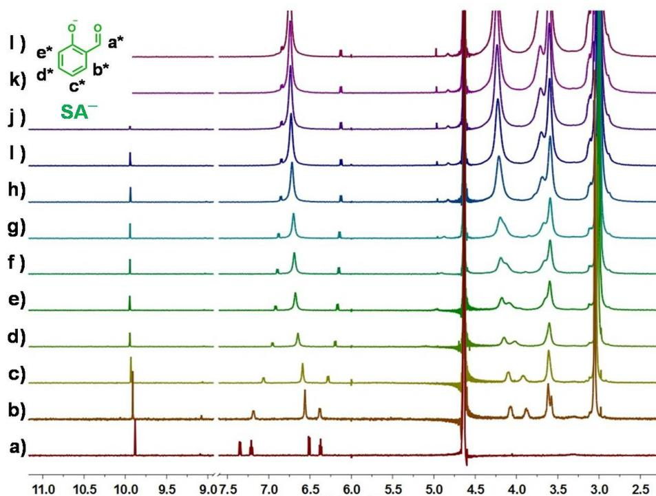
**Fig. S10** <sup>1</sup>H NMR spectra (D<sub>2</sub>O, pD 11.0, 293 K, 400 MHz) of SA<sup>-</sup> at a concentration of 1.00 mM with different concentrations of AP5: a) 0.000 mM, b) 0.310 mM, c) 0.550 mM, d) 0.810 mM, e) 1.01 mM, f) 1.40 mM, g) 1.60 mM, h) 3.22 mM, i) 4.22 mM, j) 4.90 mM, k) 6.02 mM, and l) 6.80 mM.
