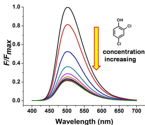
**Fig. S35** Fluorescence titration for the competitive displacement of salicylaldehyde (0.500 mM) from AP5 (1.00 mM) by **G5** (0, 0.250, 0.750, 1.50, 2.50, 3.75, 5.00, 6.25, 7.50, and 8.75 mM) in PBS at pH 7.2 ( $\lambda_{\text{ex}} = 370 \text{ nm}$ ,  $\lambda_{\text{em}} = 502 \text{ nm}$ ).
