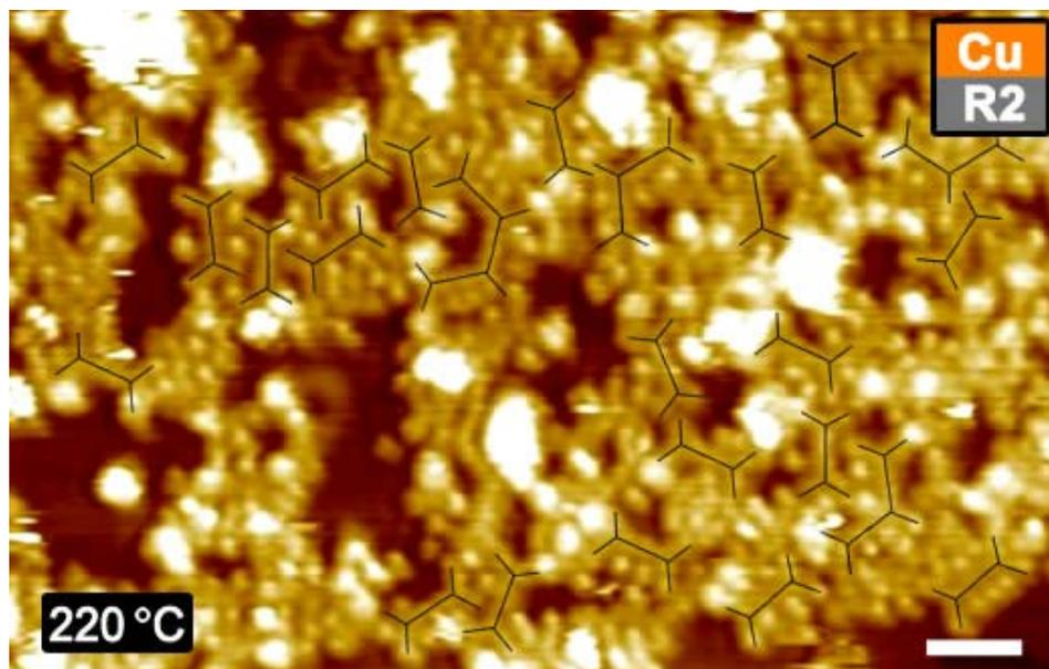
**Figure S2:** STM image of the oligomers coupled from TBB monomers after 220 °C annealing using the Cu R2 protocol. As highlighted by the black line symbols, over half of the molecules have been coupled to dimers. Uncoupled monomers still exist and detached Br atoms could be found located around the oligomers. Due to the more dosage of Cu, the clusters make the scanning a hard task. Scale bar: 2 nm.
