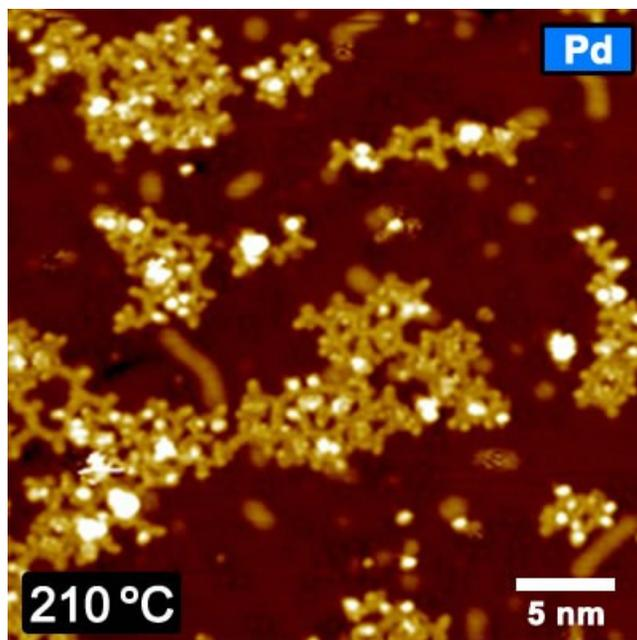
**Figure S3:** Overview STM image of the oligomers formed by the Pd-catalyzed coupling of TBB molecules on BN/Ni(111) after 210 °C annealing. Majority of the oligomers are of dimeric size, and Pd-involved intermediates could be hardly observed.
