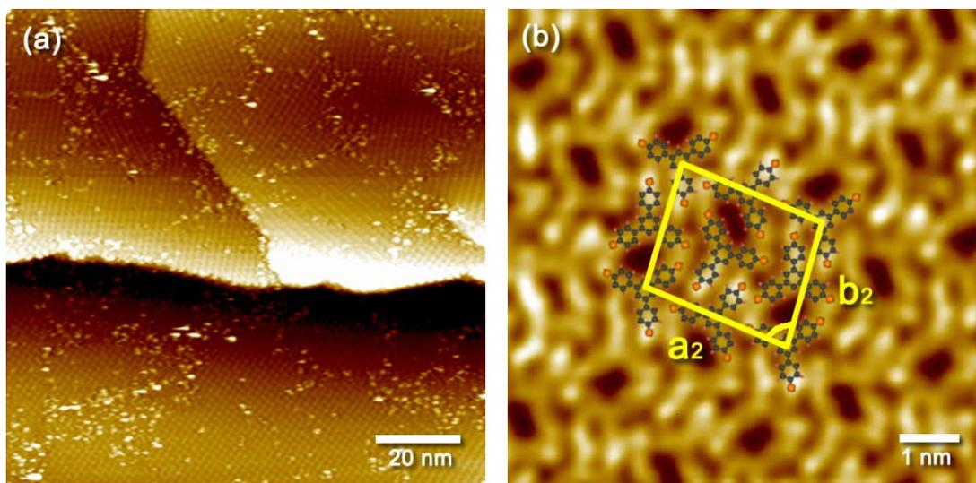
**Figure S1:** (a) STM images of the large-scale view of the TBB monolayer on h-BN/Ni(111). (b) The other assembly phase in addition to the one shown in Fig. 1a. Ordered domains are separated by the line defects of the h-BN underneath. Unit cell:  $a_2 = 2.6$  nm and  $b_2 = 2.1$  nm with an angle of  $84^\circ$ , containing four molecules. All the molecules are organized via halogen-hydrogen and halogen-halogen interactions.
