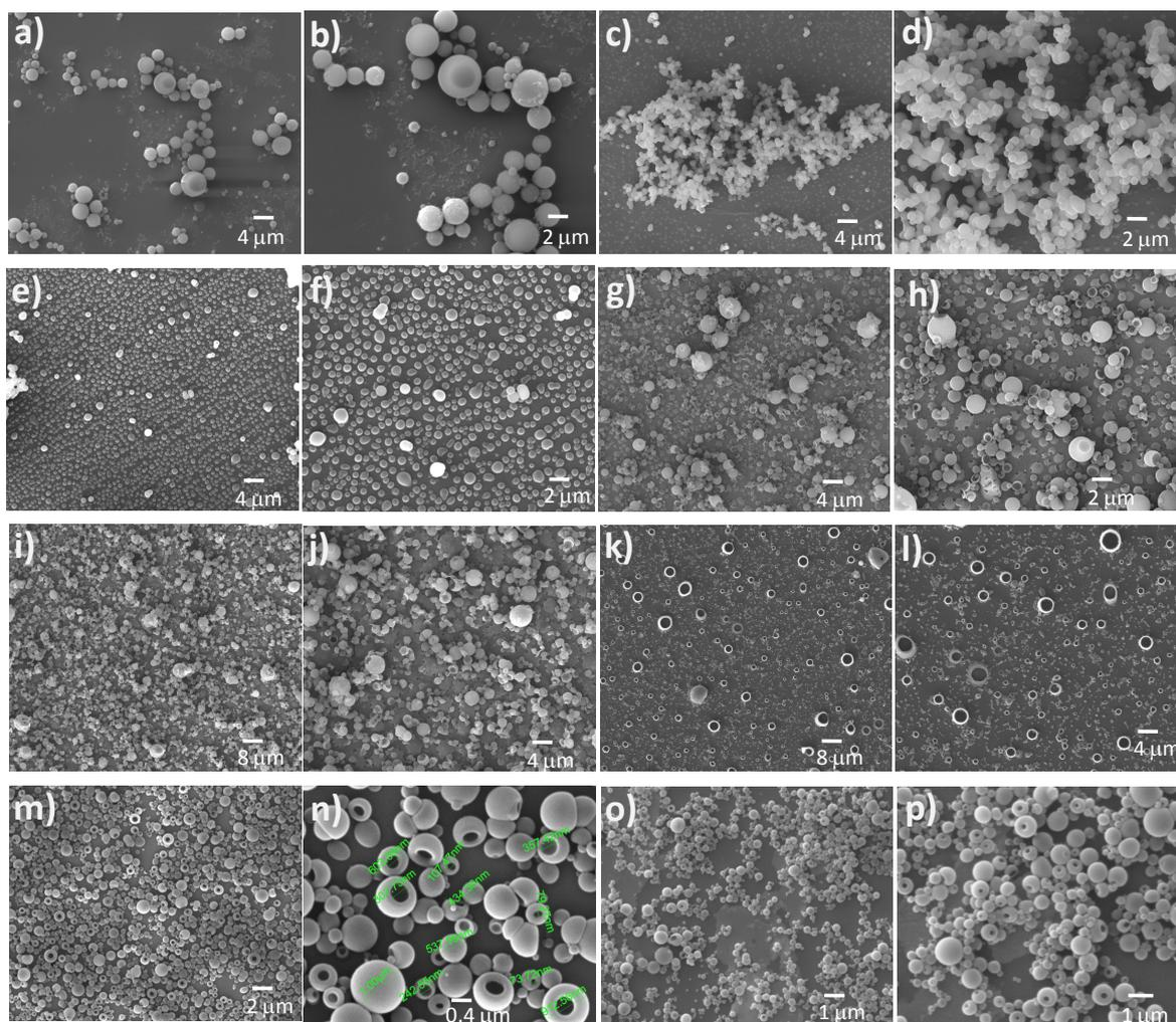
**Fig. S1** Self-assembly of octapeptide **2**. Large area SEM images of octapeptide **2** at a concentration of 1 mg/0.5 mL: (a, b) methanol, showing the association of particles to generate twins, triplets, or even multiplets; (c, d) 9:1 methanol-toluene; (e, f) 8:2 methanol-toluene; (g, h) 6:4 methanol-toluene; (i, j) 5:5 methanol-toluene; (k, l) 2:8 methanol-toluene; (m, n) 1:9 methanol-toluene and (o, p) 0.8:9.2 methanol-toluene.
