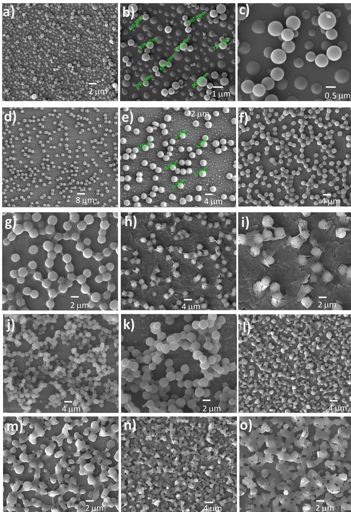
**Fig. S4** Self-assembly of octapeptide **2** at a concentration of 1 mg/0.5 mL. SEM images from different solvent ratios: (a-c) TFE; (d,e) 9:1 TFE-DMSO; (f,g) 8:2 TFE-DMSO; (h,i) 5:5 TFE-DMSO; (j,k) 2:8 TFE-DMSO; (l,m) 1:9 TFE-DMSO and (n,o) DMSO.
