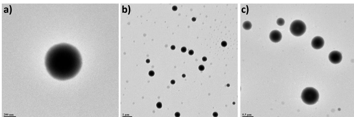
**Fig. S9** TEM images of the spherical assembly formed by compound **1** in MeOH at a concentration of 1 mg/1 mL.
