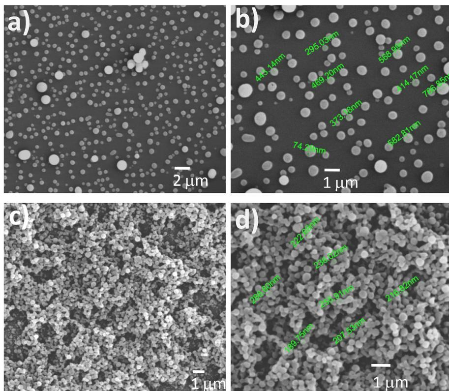
**Fig. S5** Self-assembly of octapeptide **2** at a concentration of 1 mg/0.5 mL. SEM images from different solvent mixtures: (a,b) 5:5 methanol-chloroform and (c,d) 5:5 methanol-water.
