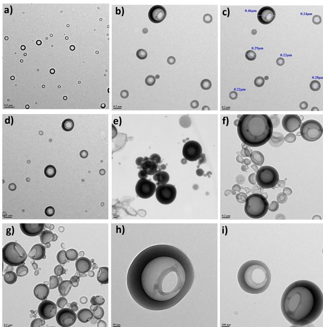
**Fig. S2** Self-assembly of octapeptide **2** at a concentration of 1 mg/mL from 1:9 methanol-toluene solvent mixture. TEM images and scale bars are: (a) 0.5 μm; (b-g) 0.2 μm; (h) 50 nm and (i) 100 nm.
