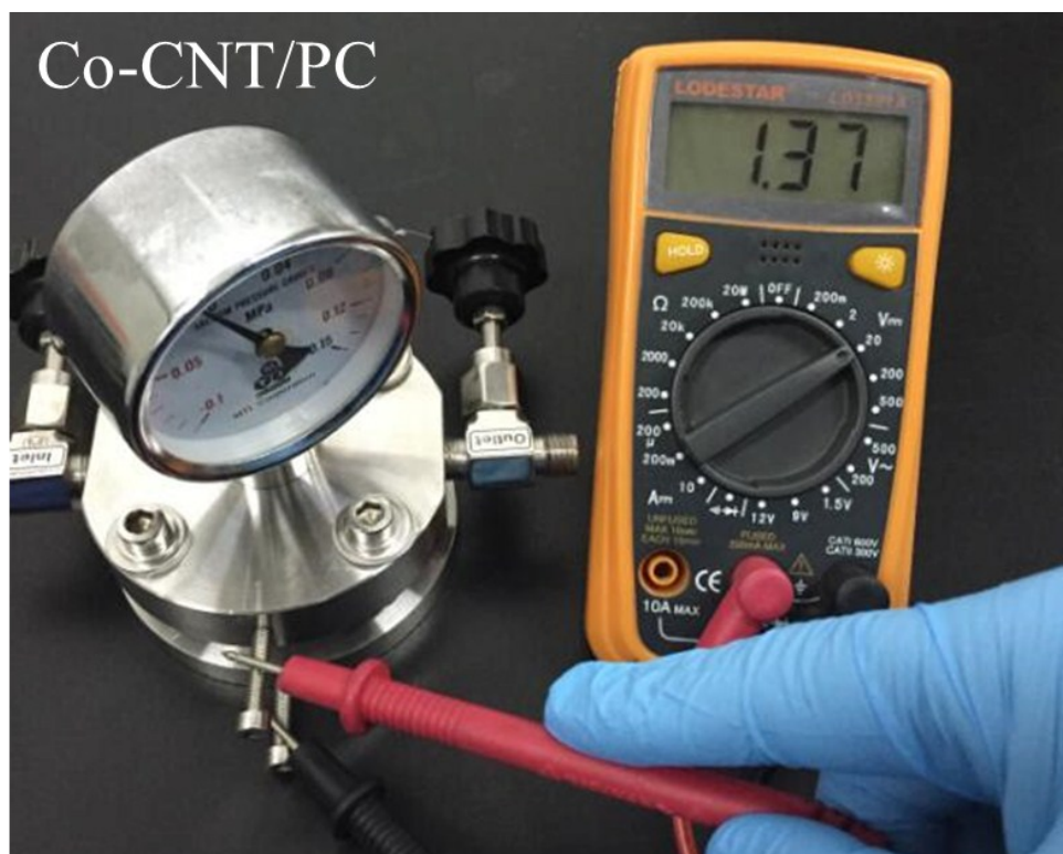
Figure S18. The optical photograph of rechargeable Zn-air battery with an open circuit potential of 1.37 V using Co-CNT/PC as air electrode.
