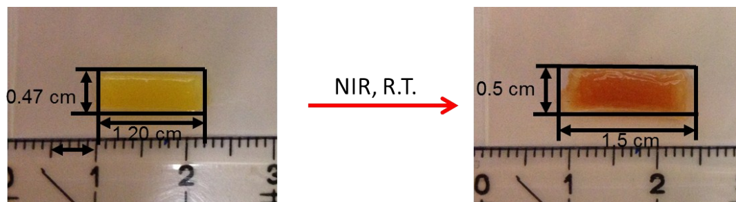
Figure S5. Nanocomposite hydrogel in the water solution (1.5 mL, pH = 3.5) before and after NIR light irradiation ( 5.5 \text{ W/cm}^2 , 15 min) at room temperature.
