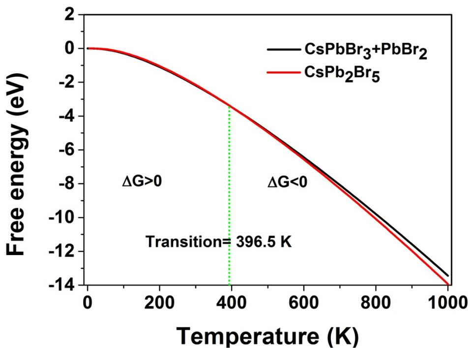
Fig. S4 The free energy of CsPbBr<sub>3</sub>+PbBr<sub>2</sub>, CsPb<sub>2</sub>Br<sub>5</sub>, as well as active temperature.
