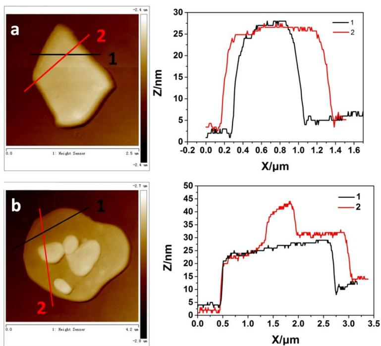
**Fig. S6** AFM images of CsPb<sub>2</sub>Br<sub>5</sub> nanosheets obtained at 2 h.
