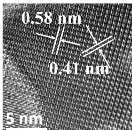
**Fig. S1** The HRTEM image of orthorhombic CsPbBr<sub>3</sub> nanosheets obtained at 1h. The 0.58 nm and 0.41 nm could be indexed to the (110) and (020)/(200) crystal planes of orthorhombic CsPbBr<sub>3</sub>.
