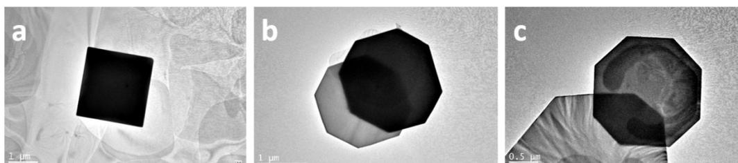
Fig. S5 The typical TEM images of CsPb<sub>2</sub>Br<sub>5</sub> nanosheets.
