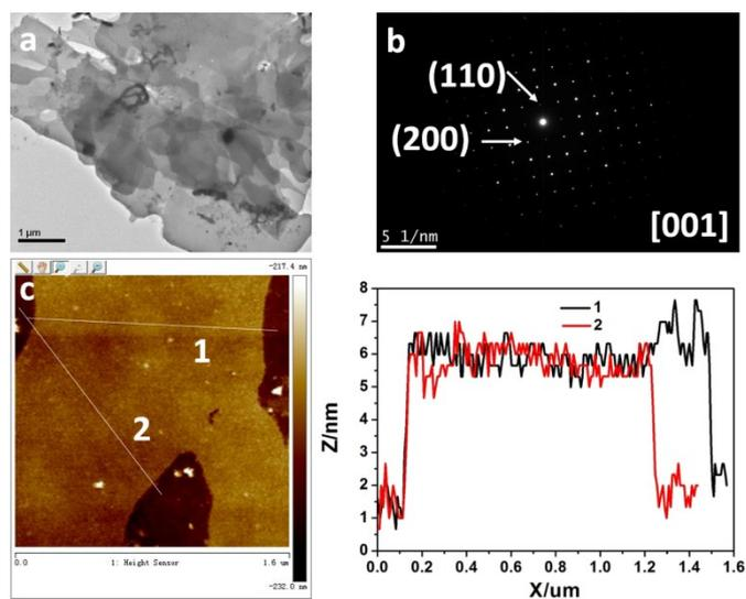
**Fig. S7** The (a) TEM, (b) SAED and (c) AFM images of ultrathin CsPb<sub>2</sub>Br<sub>5</sub> nanosheets.
