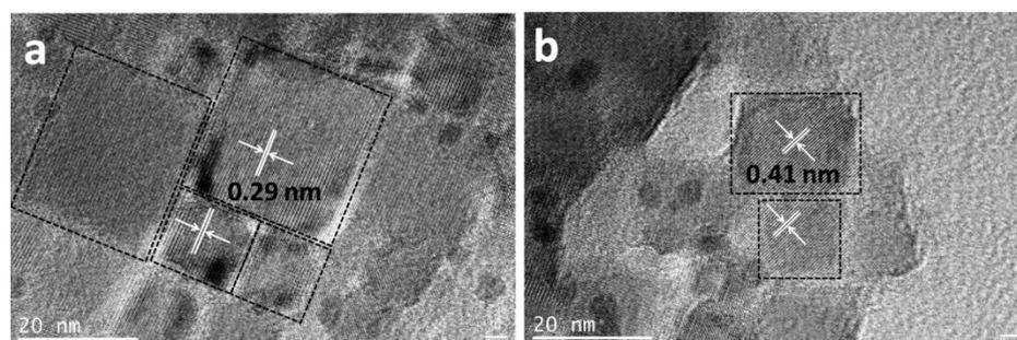
**Fig. S2** Typical HRTEM images showing the CsPbBr<sub>3</sub> nanocubes coalescence via OA mechanism at 10 min. The arrows show the traces of coalescence. The 0.29 nm and 0.41 nm could be indexed to (220) and (020)/(200) crystal planes of orthorhombic CsPbBr<sub>3</sub>.
