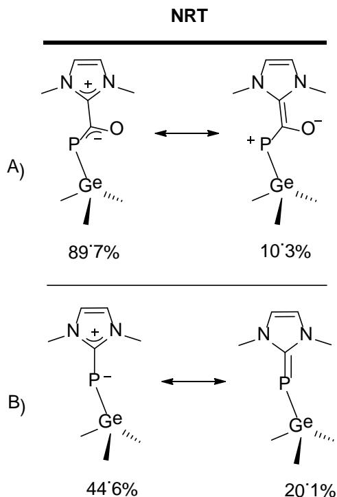
**Scheme S1.** Main resonance structures (NRT) of NHC-phosphaketene adduct (A) and NHC-phosphanide adduct (B).
