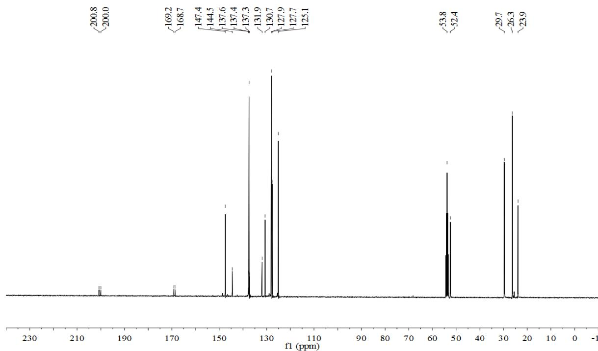
**Figure S8.**  $^{13}\text{C}\{\text{H}\}$  NMR spectrum of **2ca** in  $\text{CD}_2\text{Cl}_2$ .
