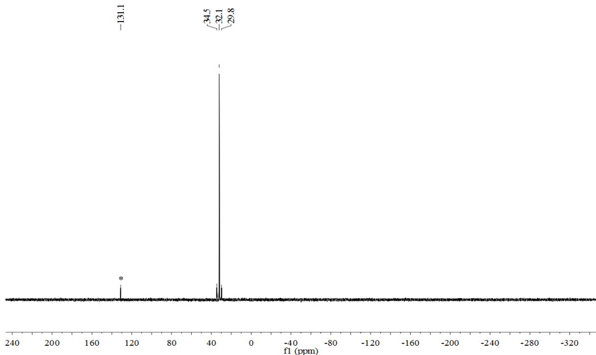
**Figure S3.**  $^{31}\text{P}\{\text{H}\}$  NMR spectrum of **2aa** in  $\text{C}_6\text{D}_6$ . \*Small impurity.
