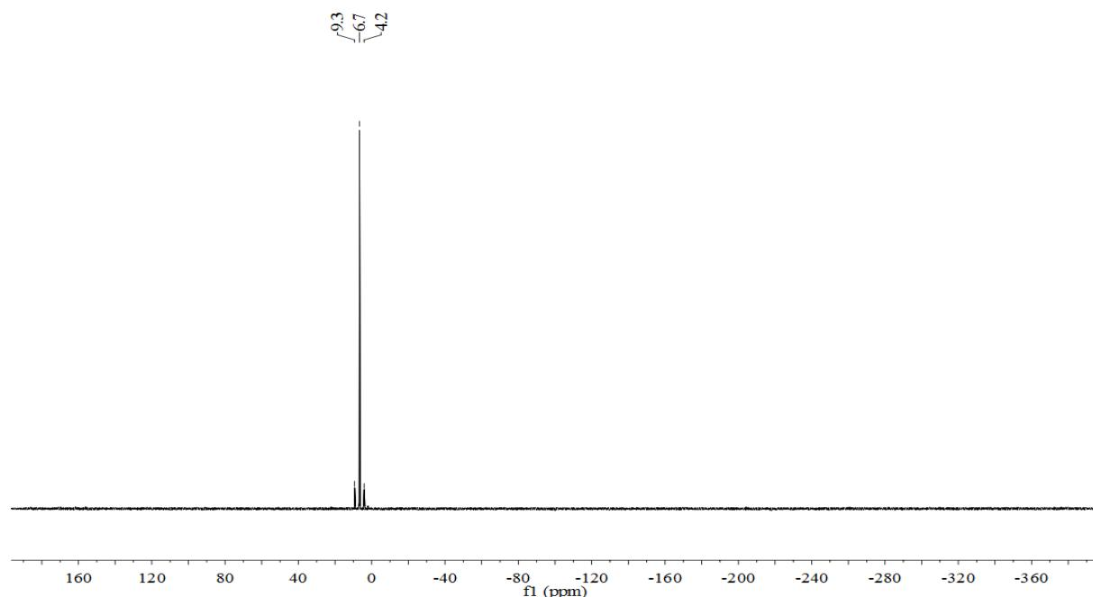
**Figure S9.**  $^{31}\text{P}\{\text{H}\}$  NMR spectrum of **2ca** in  $\text{CD}_2\text{Cl}_2$ .
