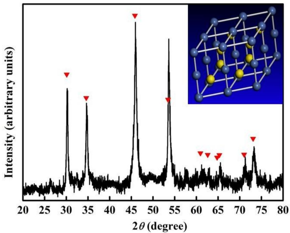
Fig. S2 XRD patterns and hexagonal unit-cell structure of NiS sample.
