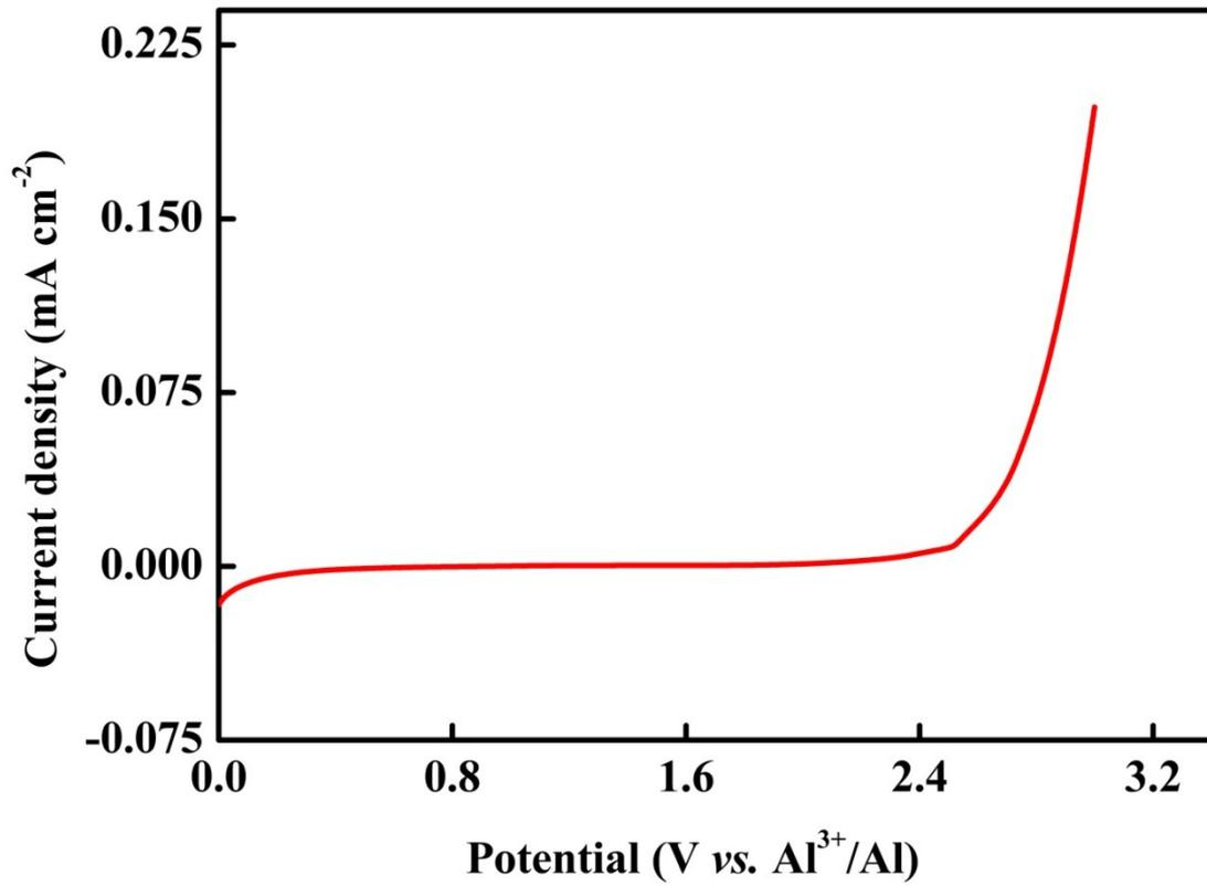
**Figure S1** The polarization curve of tantalum current collector in the AlCl<sub>3</sub>/[EMIm]Cl ionic liquid electrolyte system.
