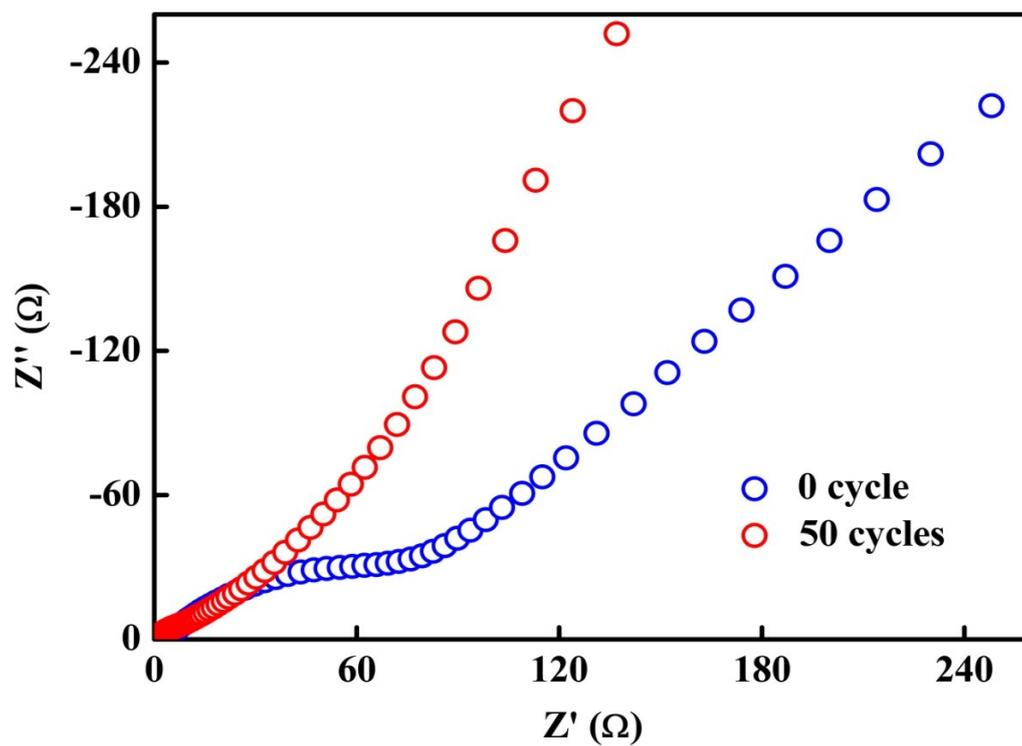
Fig. S5 AC impedance spectra of as-prepared NiS nanobelts for Al-ion batteries
