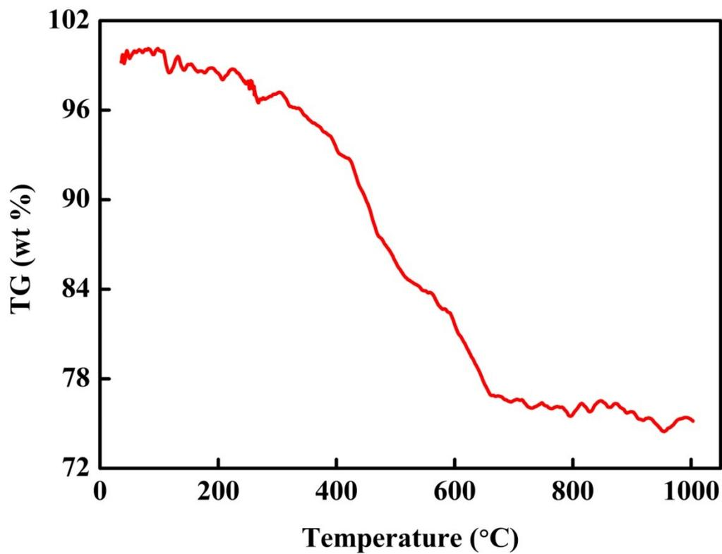
**Fig S3** TGA diagram of the as-prepared NiS nanobelts.
