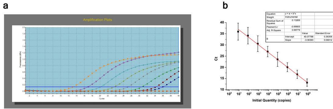
Figure S4 Typical amplification plots and corresponding standard curve for qRT-PCR analysis of miRNA-21.
