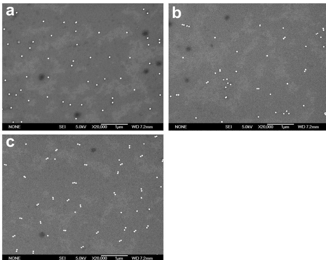
Figure S1 SEM images of the sensing system in the presence of different concentration of cDNA: a. 0 M; b. 64 pM; c. 1024 pM.
