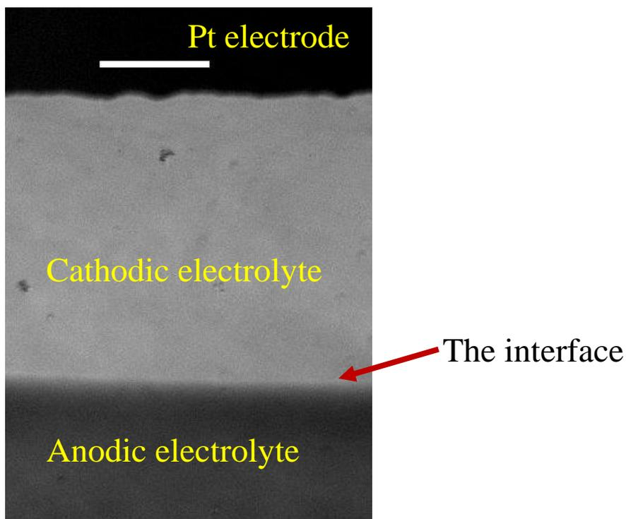
Figure S6. The micrograph of laminar flow formed by the evaporation pump with 40 cm EPT. Scale bar is 160  $\mu\text{m}$ .
