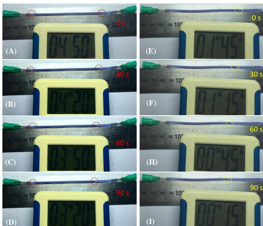
Figure S1. The solvent evaporation testing in 10 cm PVC tubes. The meniscus position in PVC tubes were recorded at an interval of 30 seconds. (A-D) are the photos of PVC tube with two blocked ends. (E-I) are the photos of PVC tube with one open end.
