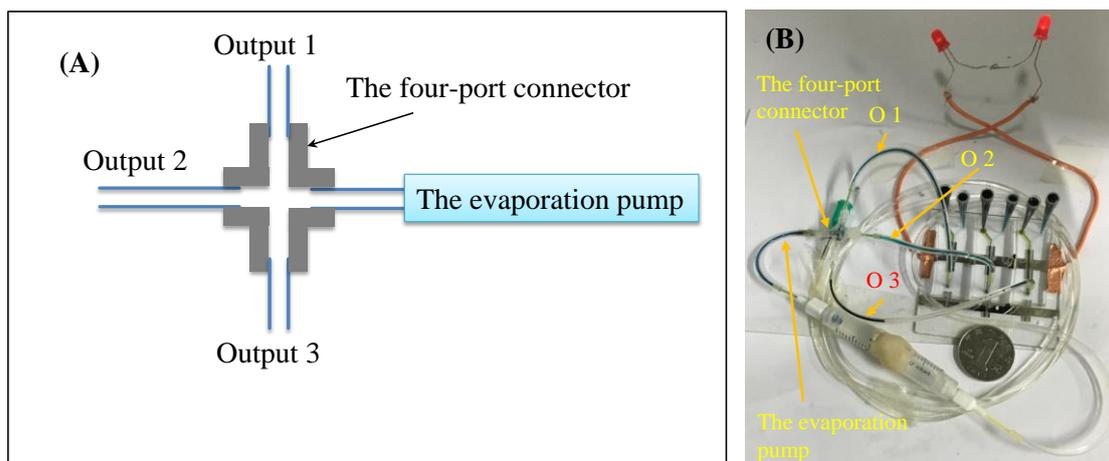
Figure S8. (A) Schematic of fluid delivery system with a four-port connector. (B) Two LEDs are lighted by installing three cells in series. The three cells are driven by the evaporation pump shown in (A).
