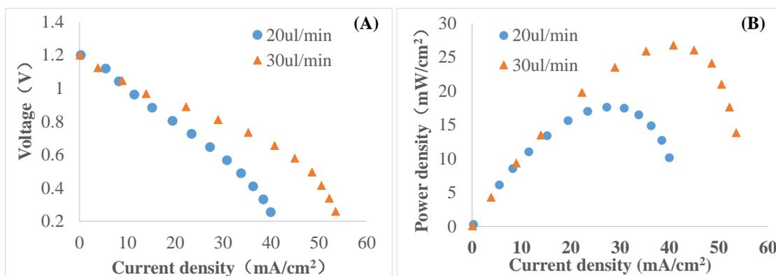
Figure S7. The steady-state polarized curves (A) and the power density curves of the cells driven by two syringes pumps under different flow rates. The anodic and cathodic electrolytes are pushed into the cell with identical flow rate (20  $\text{mL}/\text{min}$  or 30  $\text{mL}/\text{min}$ ).
