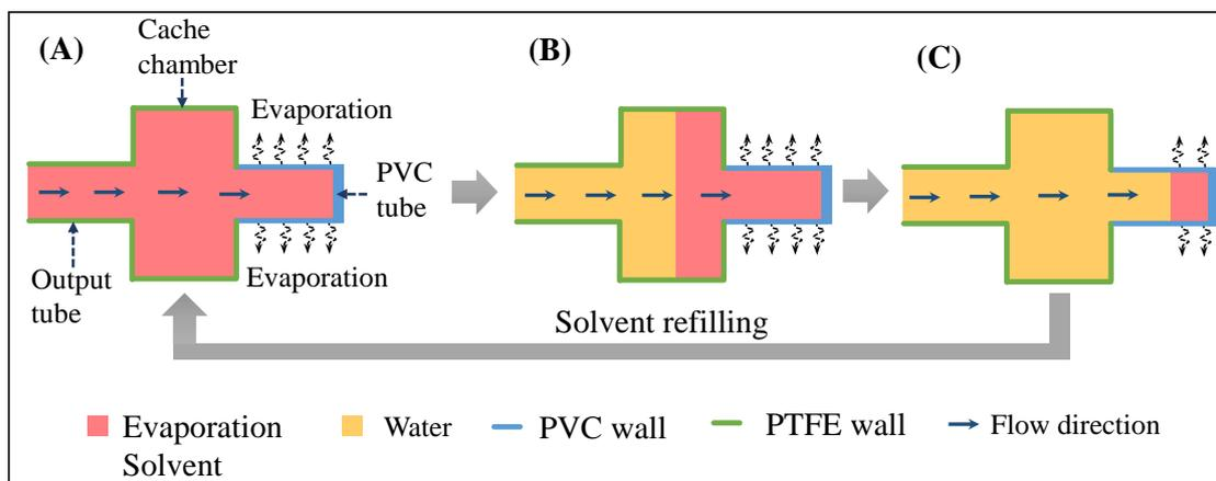
Figure S3. Schematic of fluid delivery using the evaporation pump. The system is filled with evaporation solvent, and one end of the PVC tube is blocked by the sealing plug (A). The solvent continuously diffuses into the surrounding environment via PVC wall, resulting in that the pressure in the system is reduced and water solution are sucked into the system (B). The solvent in the cache chamber flows back into the PVC tube to ensure constant evaporation area until the solvent is exhausted (C).
