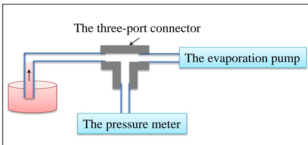
Figure S4. Schematic of the fluid delivery system used in pressure measurement. Fluid is driven by the evaporation pump.
