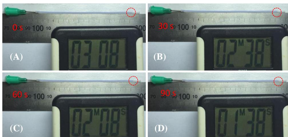
Figure S2. The solvent evaporation testing in 10 cm PTFE tubes. (A-D) are the photos of meniscus position in PTFE tubes with an interval of 30 seconds.
