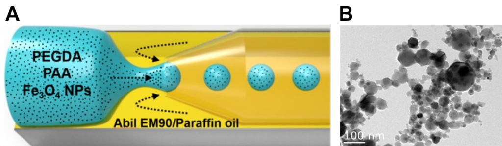
Figure S1. (A) Schematic illustration of a micro-capillary device for the generation of magnetic NPs-containing precursor W/O emulsion drops. (B) TEM image of Fe 3 O 4 NPs.
