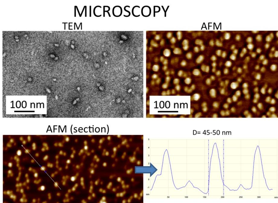
**Figure S9.** Polymeric micelles made of **3e** via the nanoprecipitation 2 method.
