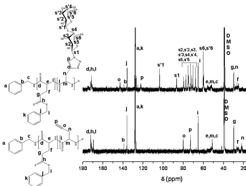
**Figure S4.**  $^{13}\text{C}$  NMR of PBLG-b-PG before and after lactose coupling
