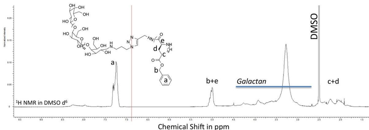
**Figure S5 :**  $^1\text{H}$  NMR of galactan-*block*-poly( $\gamma$ -benzyl-L-glutamate) **4a** in  $\text{DMSO-d}^6$  (solvent in which galactan alone is poorly soluble).
