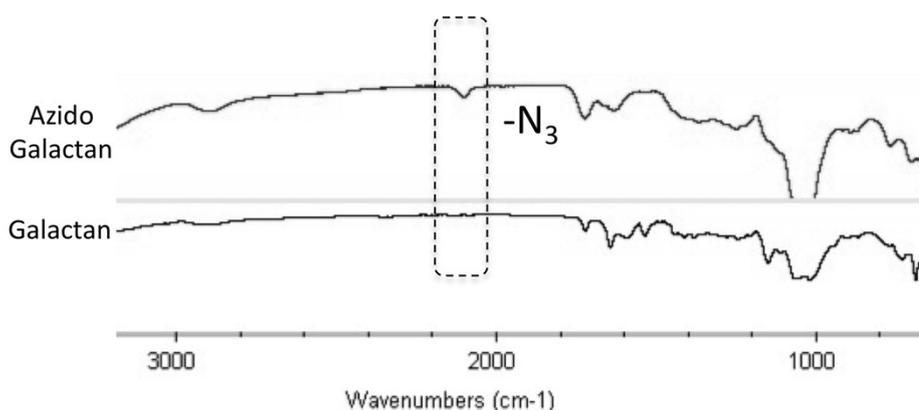
**Figure S2 :** FTIR of  $\alpha$ -azidogalactan before and after purification (% transmittance).
