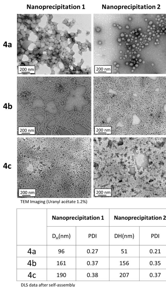
**Figure S8.** TEM images of polymeric nanoparticles made of galactan-based glycopolypeptides depending on the nanoprecipitation method used.
