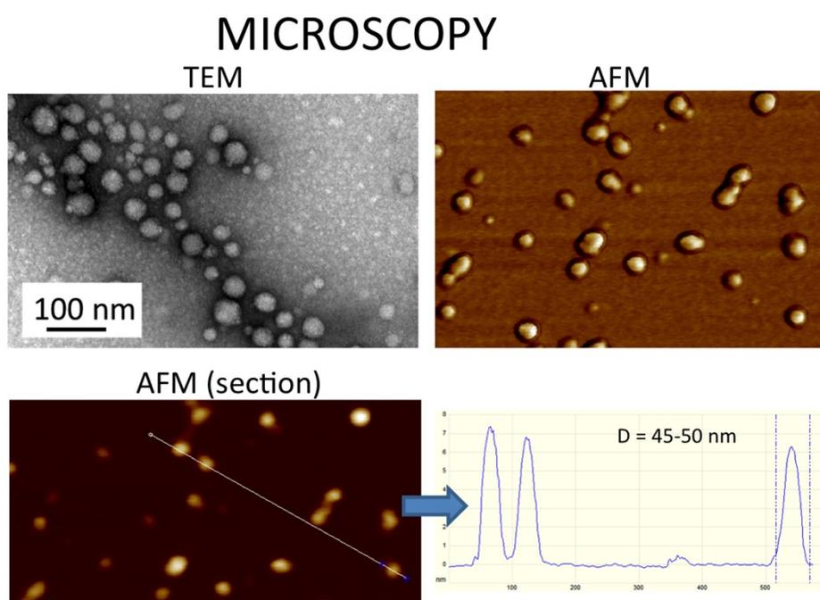
**Figure S10.** Polymeric micelles made of **4a** via the nanoprecipitation 2 method.
