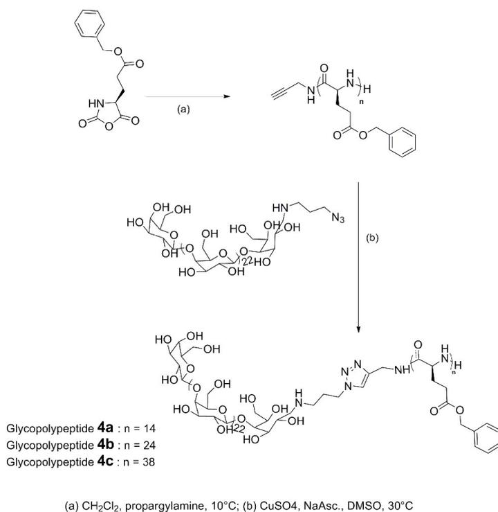
**Scheme S2.** Synthesis of poly( $\gamma$ -benzyl-L-glutamate)-block-galactan **4a-c**.
