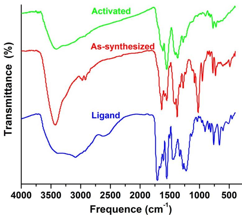
Fig. S8. Infrared spectra of the ligand TTTT, as-synthesized and activated HNUST-5. Note the absence of the vibration frequencies of the solvent DMF, DMSO and acetone molecules in the activated samples.
