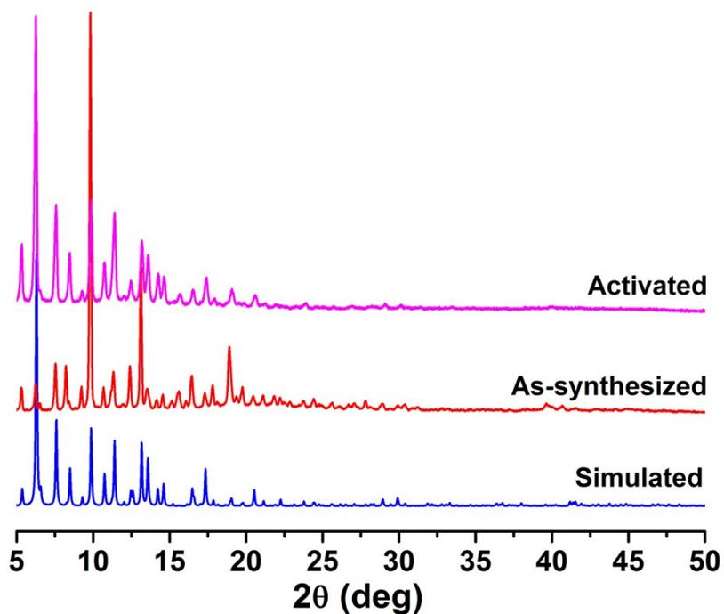
**Fig. S4.** PXR D patterns of **HNUST-5**, simulated (blue), as-synthesized (red) and activated (magent).
