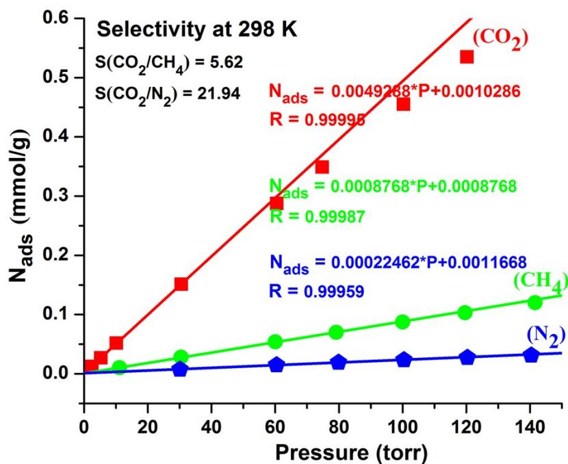
**Fig. S13.** The fitting initial slope for  $\text{CO}_2$ ,  $\text{CH}_4$  and  $\text{N}_2$  isotherms for HNUST-5 collected at 273 K and 298 K, respectively ( $N_{\text{ads}}$  = gas uptake;  $R$  = related coefficient). The calculated selectivity of  $\text{CO}_2/\text{CH}_4$  and  $\text{CO}_2/\text{N}_2$  is 7.3, 32.5 and 5.6, 21.9 at 273 K and 298 K, respectively.
