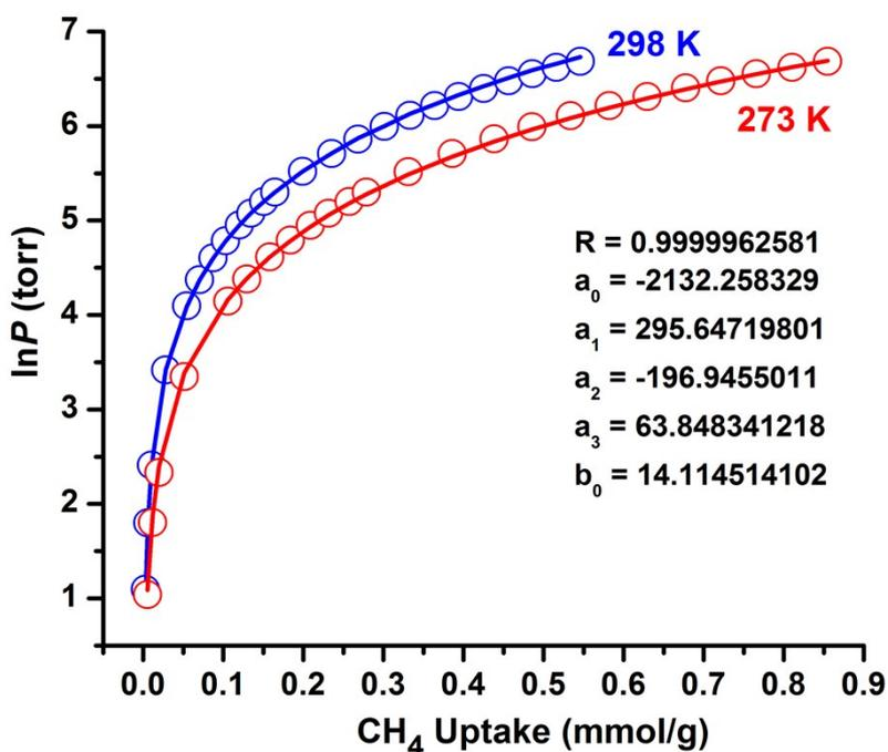
**Fig. S12.** Details of Virial equation (solid lines) fitting to the experimental gas adsorption data (symbols) for **HNUST-5** collected at 273 K and 298 K, respectively. CO<sub>2</sub> gas (upper); CH<sub>4</sub> gas (down).
