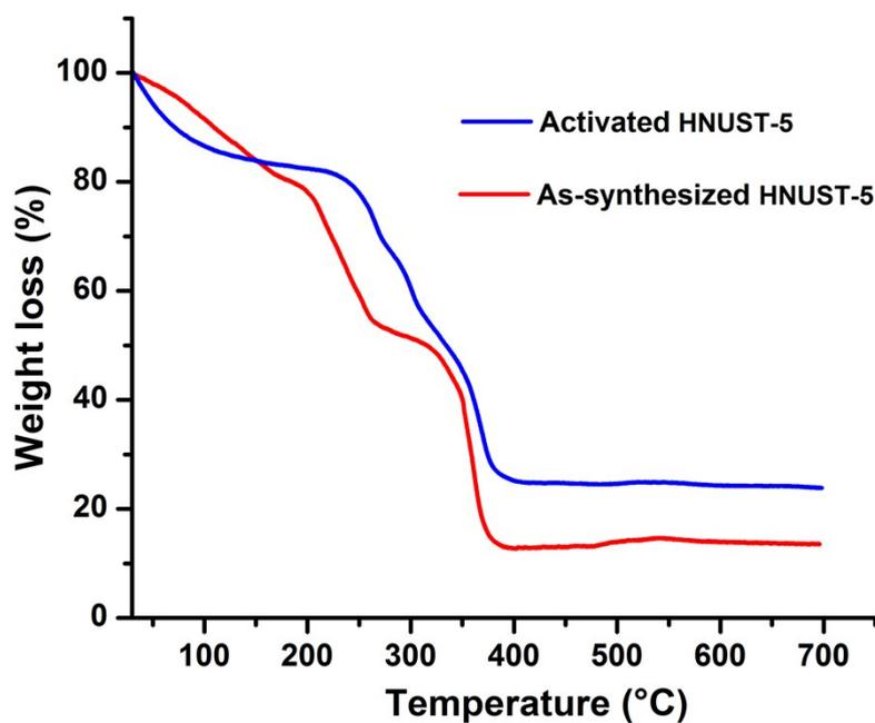
**Fig. S5.** TGA curve of the as-synthesized and activated **HNUST-5**, recorded under  $N_2$  flow with a heating rate of  $5\text{ }^\circ\text{C}/\text{min}$ .
