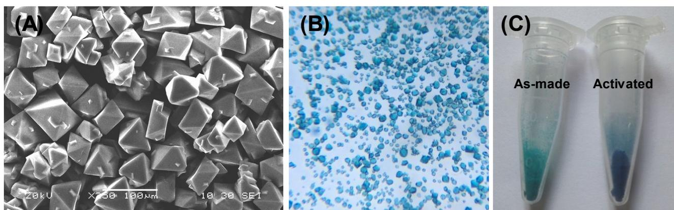
**Fig. S2.** (A) A representative SEM image of as-synthesized **HNUST-5**. (B) Photographic image of as-synthesized **HNUST-5**, the crystal size has been magnified about 80 times. (C) Visual color change of **HNUST-5** upon activation.
