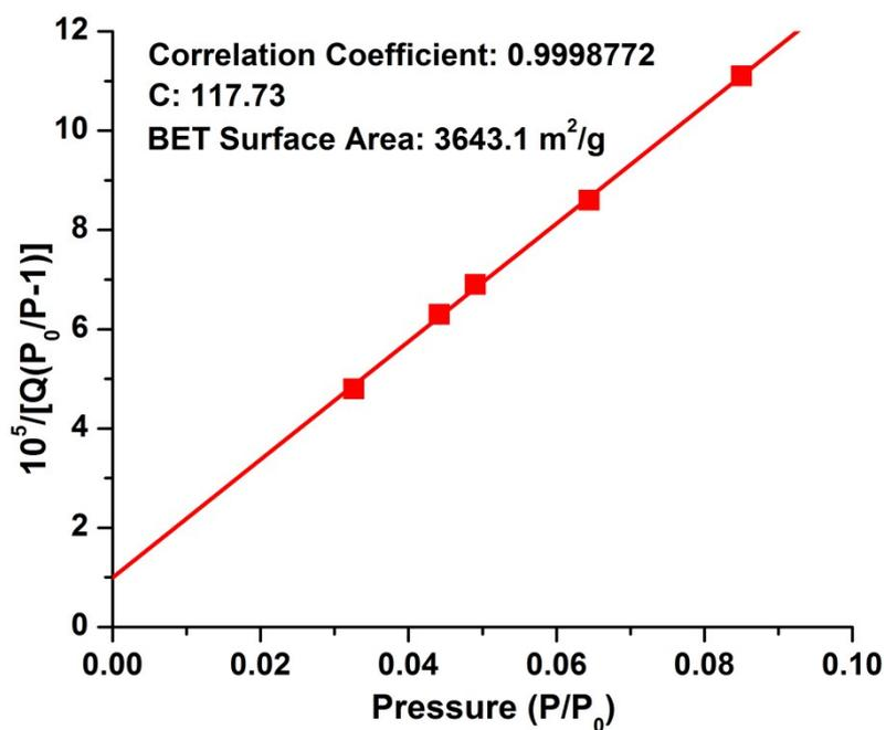
**Fig. S10.** BET plots for **HNUST-5** calculated from the N<sub>2</sub> adsorption isotherm at 77 K in the chosen range ( $P/P_0 = 0.02 - 0.1$ ).
