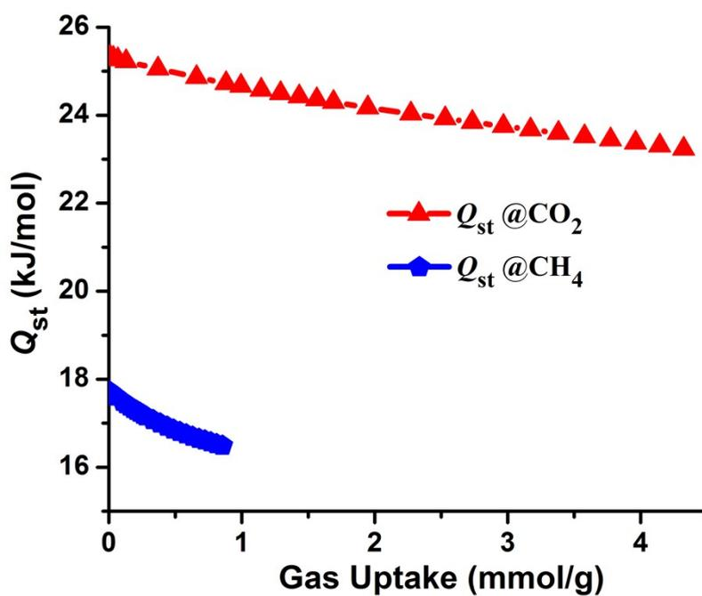
**Fig. S11.** The CO<sub>2</sub> and CH<sub>4</sub> isosteric adsorption enthalpies of **HNUST-5** calculated from the adsorptions at two different temperatures (298 K and 273 K) through the Virial method.
