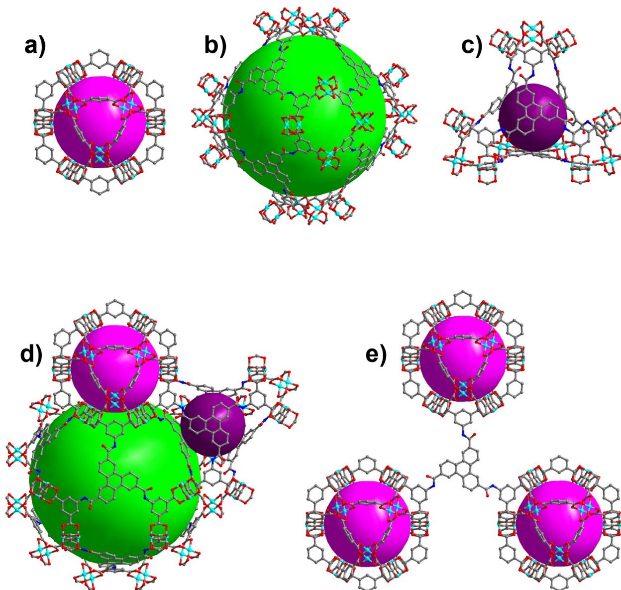
**Fig. S3.** Crystal structure of MOF **HNUST-5**. a-d) Three types of polyhedra (cuboctahedron, cub-Oh; truncated tetrahedron, T-Td and truncated octahedron, T-Oh), e) a portion of structure of the (3, 24)-connected *rht*-type framework. Coordinated water molecules have been omitted for clarity.
