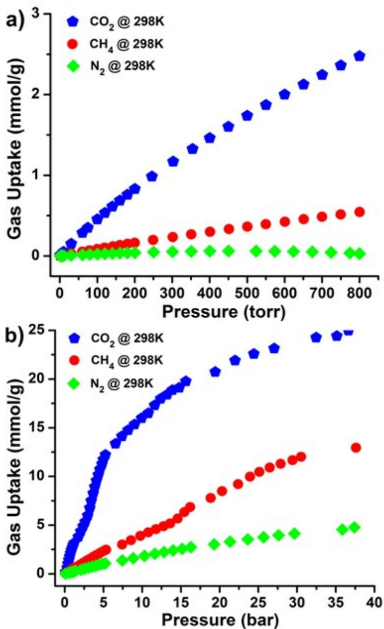
Fig. S9. Low- and high-pressure gas (CO<sub>2</sub>, CH<sub>4</sub> and N<sub>2</sub>) sorption isotherms of **HNUST-5** at 298 K.
