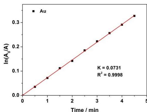
**Fig. S1** The linear fitting of absorption change at 387 nm of aqueous solution containing **AM** and  $\text{Na}_2\text{-ADPA}$  in the course of irradiation under white light.
