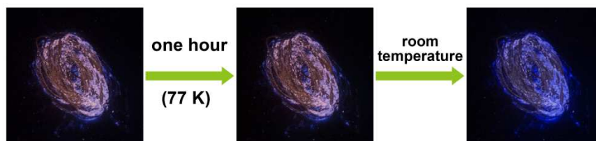
Fig. S16 Photographs of o -CH 3 - p -an after grinding one hour at 77 K and the temperature raised to r.t. ( \lambda_{\text{ex}} = 365 \text{ nm} ).
