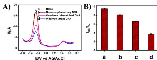
**Fig. S12** The specificity of the ratiometric electrochemical sensor for the discrimination of target DNA, one-base mismatched DNA and noncomplementary random DNA, the concentration of DNA is 50 pM; A) DPV spectra; B) histogram.
