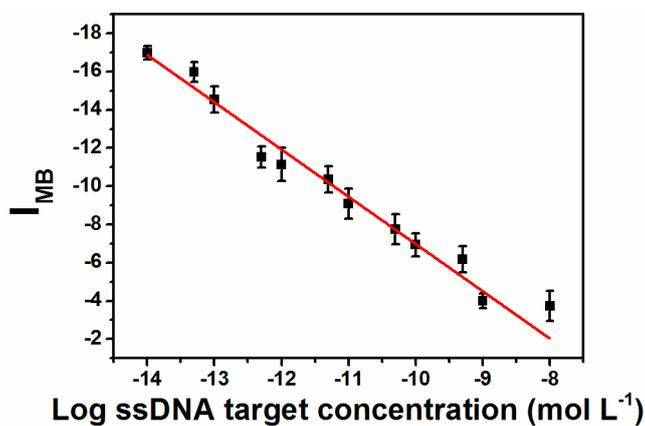
**Fig. S10** The linear relationship between the current  $I_{MB}$  and logarithm of target DNA concentration.
