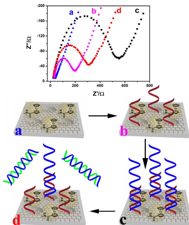
**Fig. S8** Electrochemical impedance spectroscopy of a) bare Fc-GSHs modified electrode; b) single-strand assistant DNA probe conjugated onto as-fabricated electrode in a); c) electrode b) treated with recognition DNA probe to form duplex DNA on GSHs surface; d) electrode c) cultured with target DNA.
