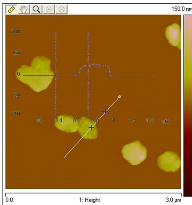
**Fig. S1** Representative AFM images of the as-synthesized hybridized nanomaterials GSHs and the corresponding height profiles along the line in AFM images.
