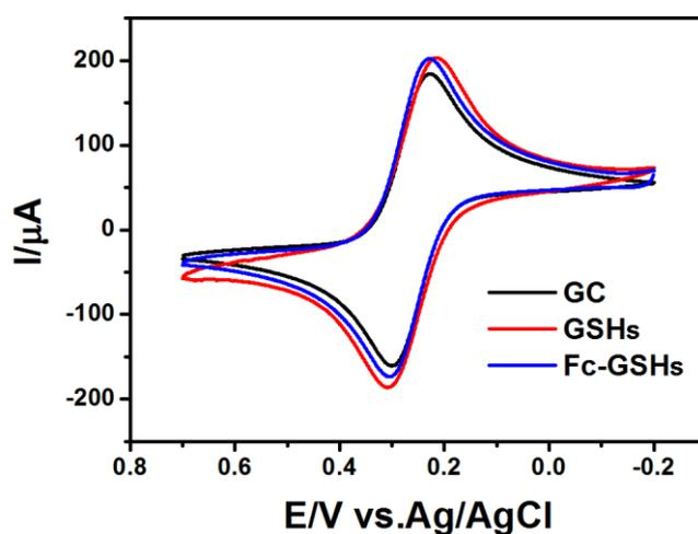
**Fig. S4** Cyclic voltammograms of bare glassy carbon (GC) electrode, GSHs and Fc-GSHs modified electrode in 10 mM  $K_3[Fe(CN)_6]$  containing 0.1M KCl.
