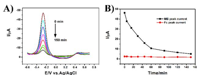
**Fig. S9** Release profiles of electro-active molecules MB from single-strand assistant DNA probe modified GSHs: A) DPV spectra; B) linear plot. The optimized culture time is 60 min according to the linear plot.
