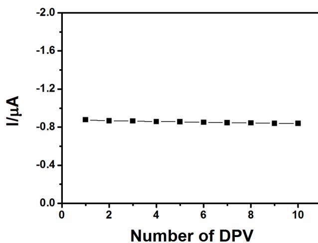
**Fig. S5** The stability of modified electrode surface for 10 measurements. DPV peak current of Fc in Fc-GSHs was recorded as the readout signal.
