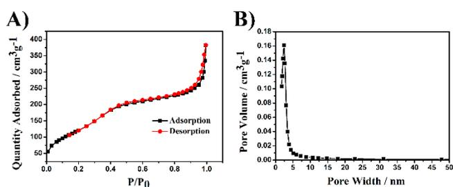
**Fig. S2** BET nitrogen adsorption–desorption isotherm (A) and BJH pore size distribution curve (B) of GSHs.
