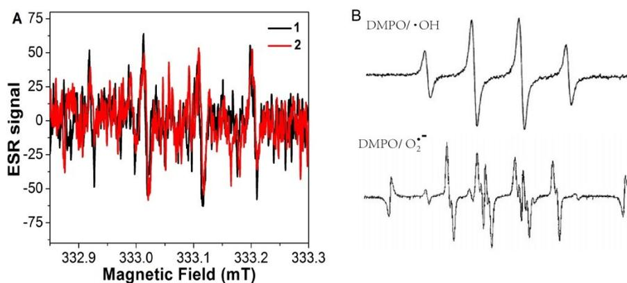
**Fig. S8** (A) ESR spectra of DMPO adduct by  $\cdot\text{OH}$  and  $\text{O}_2\cdot^-$  trapped with DMPO in (1) luminol solution and (2) FCNs-luminol system. (B) The specific ESR spectra of DMPO/ $\cdot\text{OH}$  and DMPO/ $\text{O}_2\cdot^-$  adduct which from [ref. 1](#) (Hui Chen et al. 2010) and [ref. 2](#) (Yasuko Noda et al. 1997).
