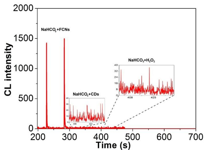
**Figure S6** The CL files  $\text{NaHCO}_3$ -FCNs,  $\text{NaHCO}_3$ -CDs and  $\text{NaHCO}_3$ - $\text{H}_2\text{O}_2$  system with the same NaOH concentration of 0.1M. Conditions: High voltage was -1.4kV; interval time was set for 0.1 s. The concentration of  $\text{NaHCO}_3$  is 0.1M; the FCNs is in the dilution of 1:5000 with water. The CDs is in the dilution of 1:100 with water.
