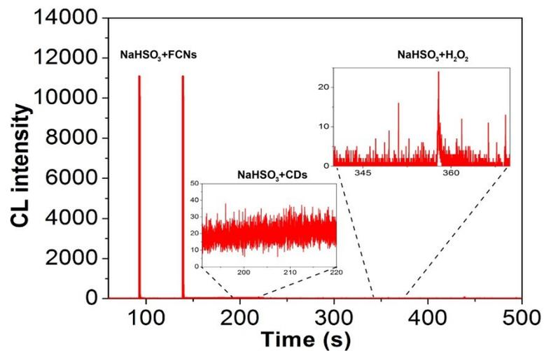
**Figure S7** The CL files  $\text{NaHSO}_3$ -FCNs,  $\text{NaHSO}_3$ -CDs and  $\text{NaHSO}_3$ - $\text{H}_2\text{O}_2$  system with the same NaOH concentration of 0.1M. Conditions: High voltage was -1.3kV; interval time was set for 0.1 s. The concentration of  $\text{NaHSO}_3$  is 0.1M; the FCNs is in the dilution of 1:5000 with water. The CDs is in the dilution of 1:100 with water.
