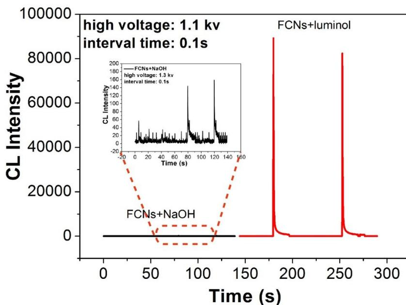
**Figure S4** The comparison of CL signal for FCNs-NaOH and FCNs-luminol system. Conditions: High voltage was -1.1 kV; interval time was set for 0.1 s. The concentration of luminol is  $10^{-5}$  M; The concentration of NaOH is 0.1 M; the FCNs is in the dilution of 1:5000 with water.
