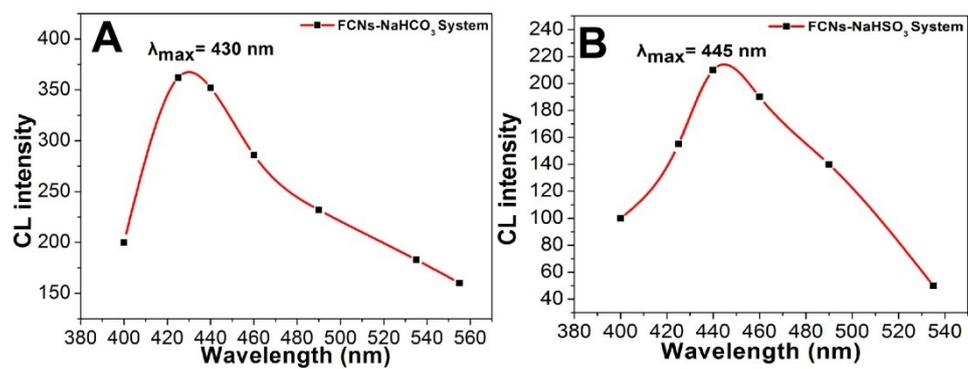
**Fig. S9** The CL spectra of FCNs-NaHCO<sub>3</sub> and FCNs-NaHSO<sub>3</sub> system
