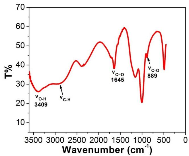
**Figure S10** The FTIR spectra of FCNs solution
