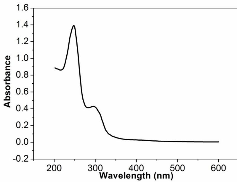
**Figure S11** The UV-vis spectra of FCNs solution
