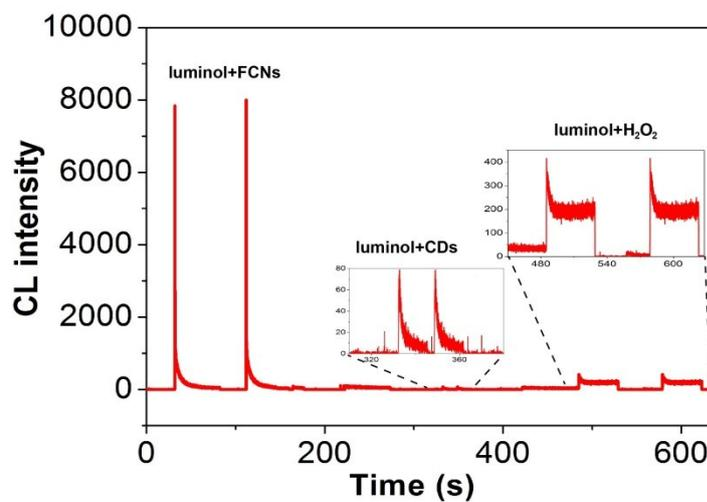
**Figure S5** The CL files luminol-FCNs, luminol-CDs and luminol-H<sub>2</sub>O<sub>2</sub> system with the same NaOH concentration of 0.1M. Conditions: High voltage was -1.2 kV; interval time was set for 0.01 s. The concentration of luminol is 10<sup>-5</sup> M; the FCNs is in the dilution of 1:5000 with water. The CDs is in the dilution of 1:100 with water.
