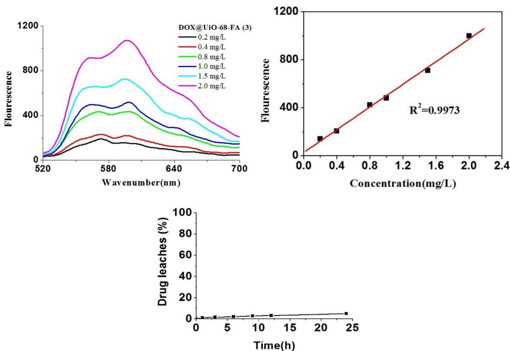
**Fig. S5** Top: luminescent intensities ( $\lambda_{\text{ex}} = 485 \text{ nm}$ ) at different concentrations of **3** and the linearity between relative luminescent intensities and concentrations. The DOX loading amount is 4.79 wt %. Bottom: the leaching experiment of **3** in PBS during 24 h, and only less than 5% of DOX loss was observed, indicating DOX was encapsulated in MOF pores.
