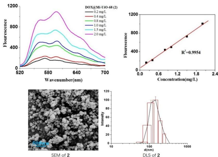
**Fig. S3** Top: Luminescent intensities ( $\lambda_{\text{ex}} = 485$  nm) at different concentrations of **2** and the linearity between the relative luminescent intensities and concentrations. The DOX loading amount is 4.84 wt %. Bottom: SEM image and DLS measurement of **2**. The NPs diameter of **2**
