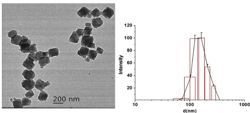
**Fig. S7** TEM image and DLS measurement of **3** in PBS. The Zeta potential of **3** in PBS is -12.8( $\pm$ 0.6) mV. These results indicate that **3** is stable in PBS.
