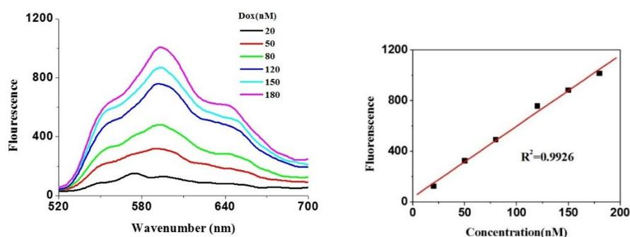
**Fig. S2** Free DOX luminescent intensities ( $\lambda_{\text{ex}} = 485$  nm) at different concentrations and the linearity between the relative luminescent intensities and concentrations of DOX.
