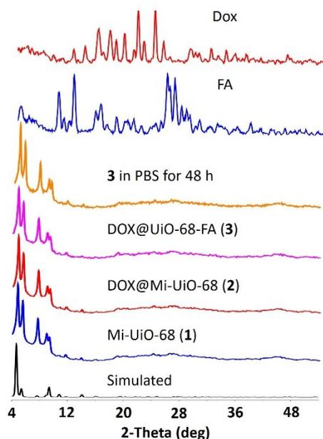
**Fig. S6** The XRPD patterns of **1-3**, Dox and FA. Compared to **1**, there are no characteristic differences in the intensities in XRPD peaks of **2** and **3** after Dox loading and FA decoration because of the low included amount of Dox and FA.
