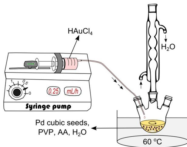
**Figure S1.** Schematic illustration of the experimental setup used for all seed-mediated syntheses where the rate of Au precursor addition was controlled by a syringe pump.
