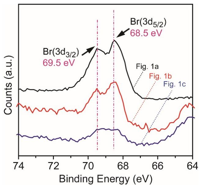
**Figure S6.** XPS spectra of structures derived from the slow-injection growth regime. Spectra were measured from structures seen in Figure 1a (black), 1b (red), and 1c (blue). Spectral signatures from Br<sup>-</sup> were detected at all stages of growth.
