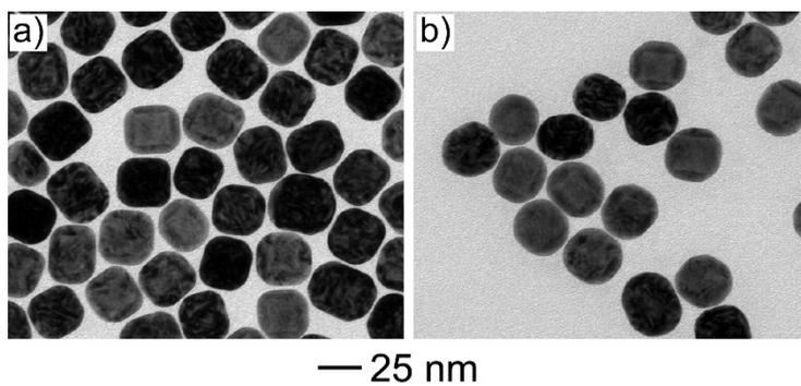
**Figure S3.** TEM images of Pd@Au core-shell nanocrystals obtained under different reaction conditions. (a) Structures produced using a similar protocol to the product shown in Fig. 2f except the reaction time was extended to 12 h. (b) The same Pd@Au nanocubes shown in Fig. 2f but after one month of aging at room temperature.
