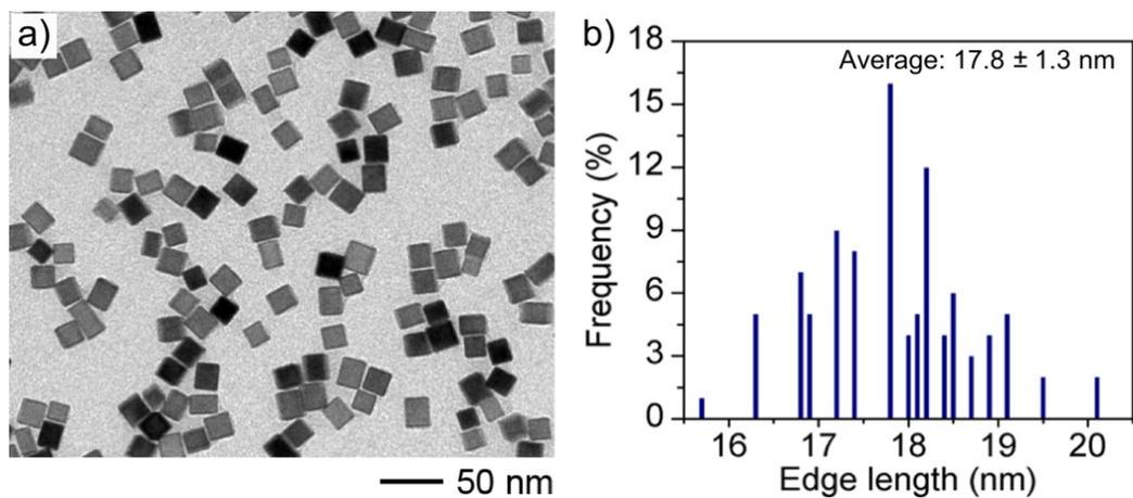
**Figure S2.** a) TEM image of the as-prepared Br<sup>-</sup> capped Pd cubic seeds and corresponding b) Histogram of the particle size distribution.
