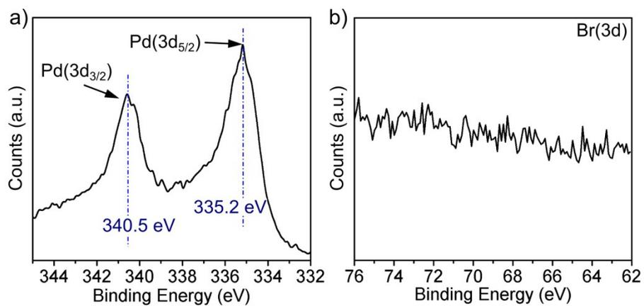
**Figure S7.** XPS spectra of a) Pd (3d) and b) Br (3d) that were collected from Pd nanocube seeds after removal of bromide ions. Spectral signatures from Pd<sup>2+</sup> and Br<sup>-</sup> were not detected.
