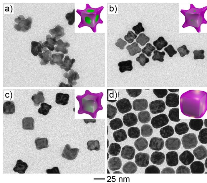
**Figure S4.** TEM images of Pd@Au nanocrystals obtained in a standard synthesis with Au precursor injected into the reaction solution at rates of a) 0.1 mL/h, b) 1 mL/h, c) 10 mL/h, and d) one-shot rapid injection.
