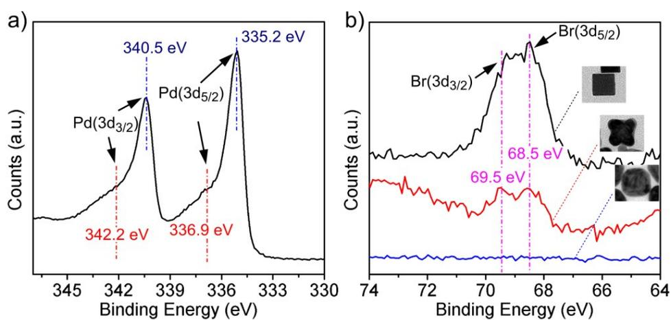
**Figure S5.** XPS spectra of Br<sup>-</sup> capped Pd nanocubes and Pd@Au core-shell nanocrystals. a) XPS spectrum of Pd (3d) obtained from the Pd nanocubes, and b) XPS spectra Br (3d) obtained from the capped Pd nanocube seeds, Pd@Au core-shell concave nanocubes, and Pd@Au core-shell nanocubes with flat surfaces, respectively.
