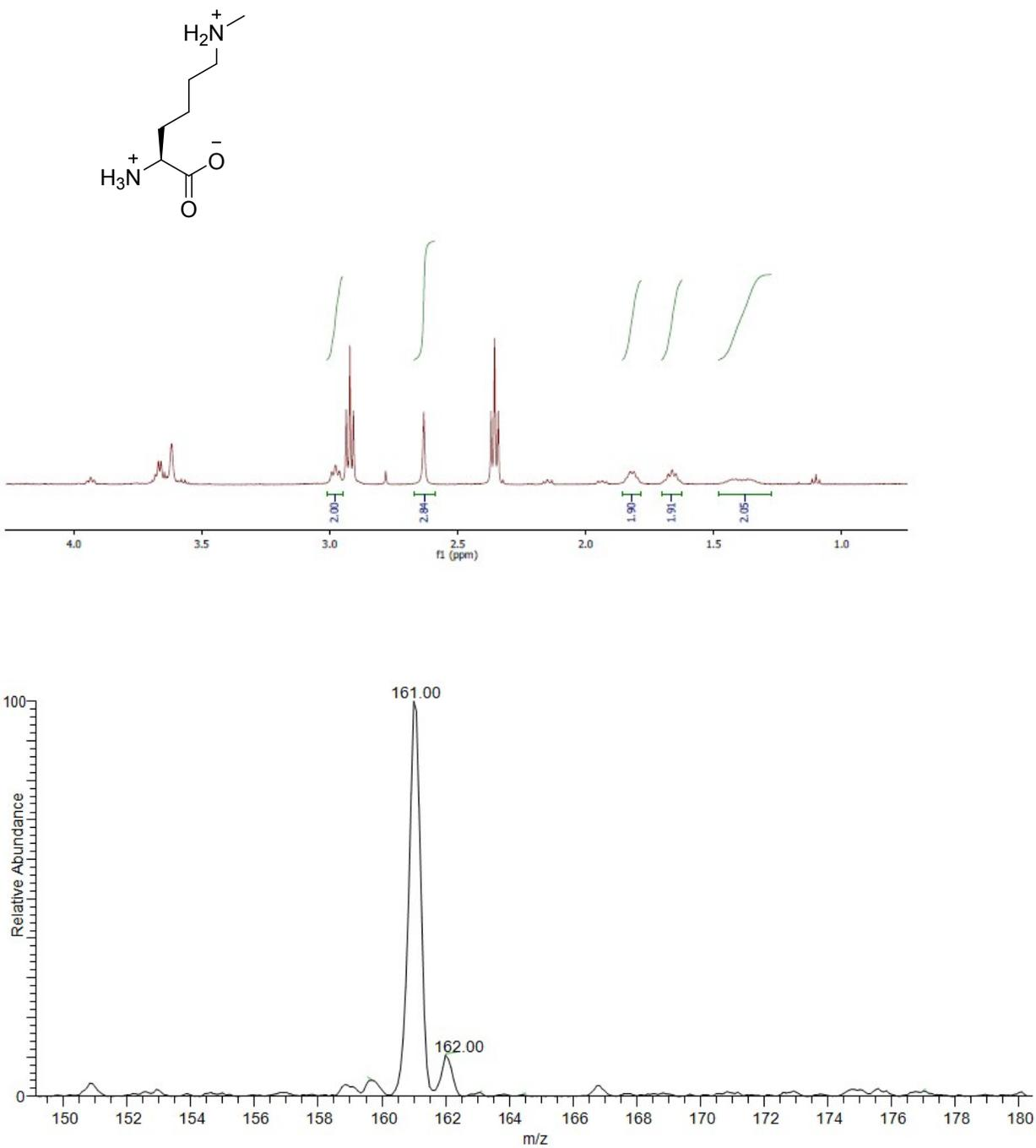
**Fig. S11** Hydroxylation of methyllysine (**3**) under standard conditions as analysed by  $^1\text{H}$  NMR (top) and LC-MS (bottom).
