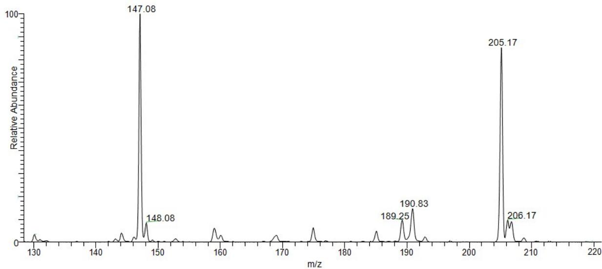
**Fig. S39** Hydroxylation of trimethyllysine (**1**) in the presence of 1 mM of mildronate (**20**) under standard conditions as analysed by LC-MS.
