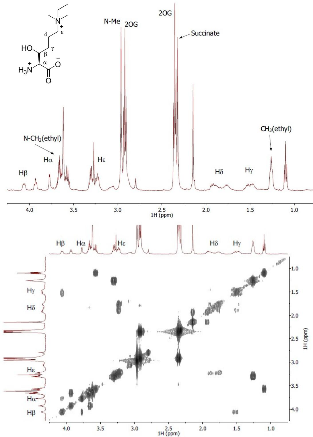
**Fig. S26** NMR analyses of TMLH-catalysed hydroxylation of dimethylethyllysine (**14**).  $^1\text{H}$  NMR data of TMLH-catalysed C-3 hydroxylation of dimethylethyllysine (top). COSY data of TMLH-catalysed C-3
