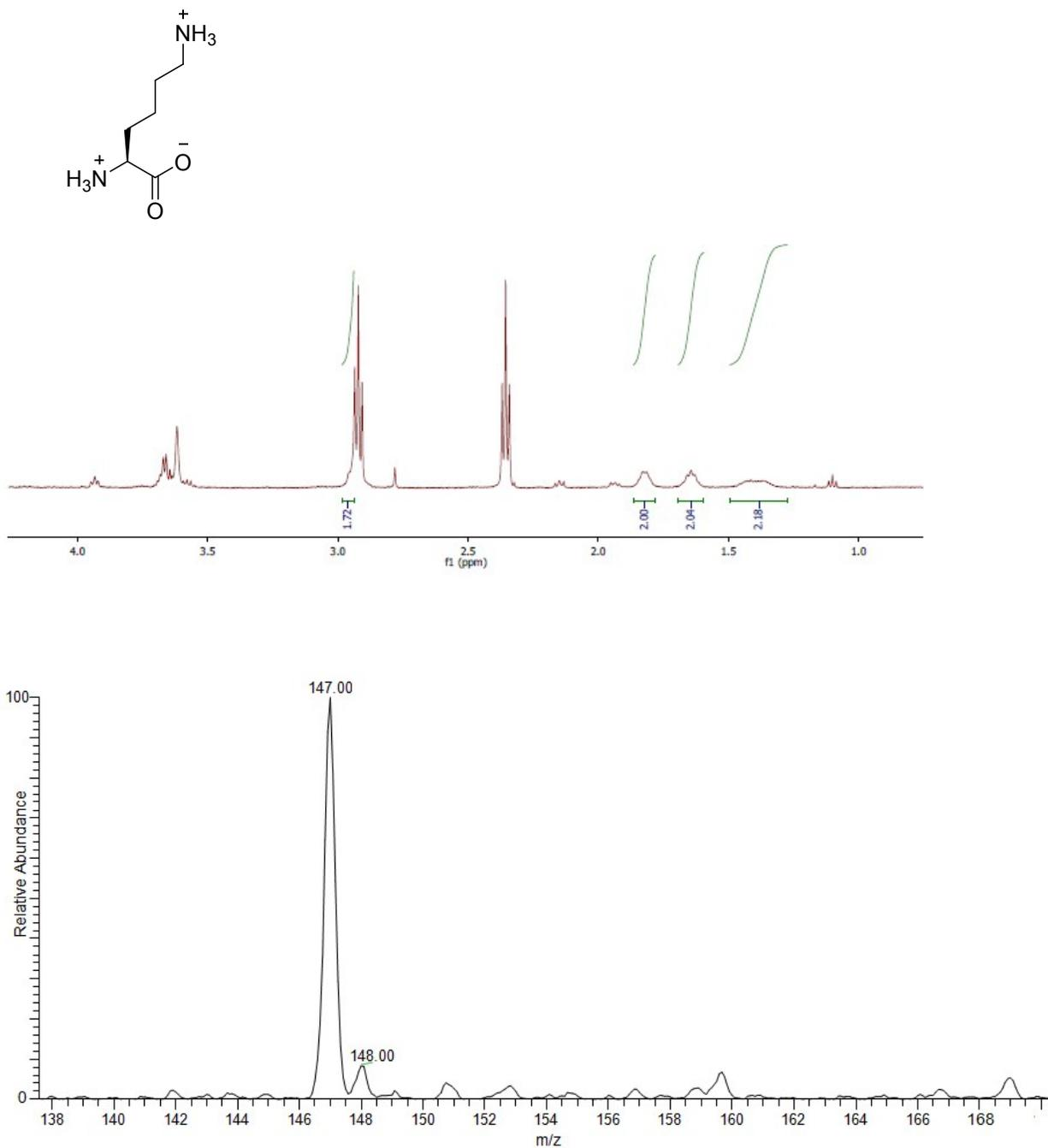
**Fig. S12** Hydroxylation of lysine (**4**) under standard conditions as analysed by <sup>1</sup>H NMR (top) and LC-MS (bottom).
