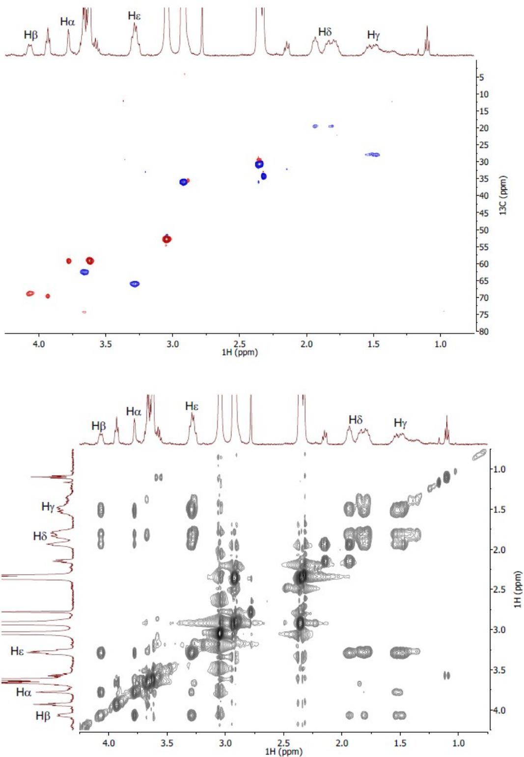
**Fig. S3** NMR analyses of TMLH-catalysed hydroxylation of trimethyllysine (**1**). Multiplicity-edited HSQC data of TMLH-catalysed C-3 hydroxylation of trimethyllysine (top; red = positive, CH/CH $_3$ , blue = negative, CH $_2$ ). TOCSY data of TMLH-catalysed C-3 hydroxylation of trimethyllysine (bottom).
