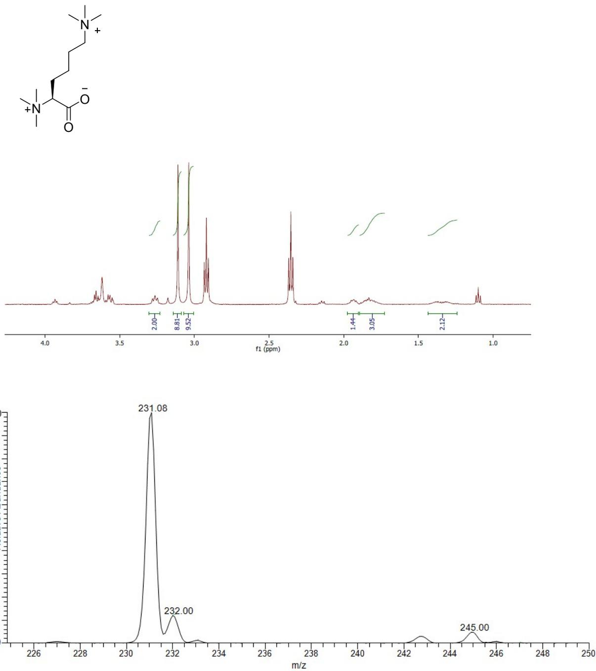
**Fig. S17** Hydroxylation of hexamethyllysine (**9**) under standard conditions as analysed by <sup>1</sup>H NMR (top) and LC-MS (bottom).
