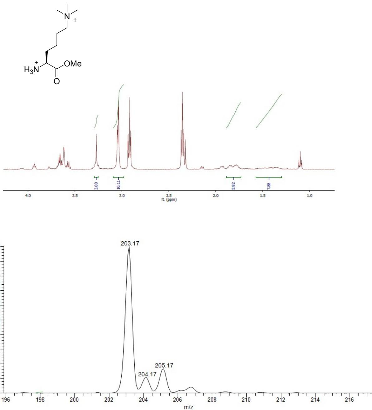
**Fig. S15** Hydroxylation of the methyl ester of trimethyllysine (7) under standard conditions as analysed by  $^1\text{H}$  NMR (top) and LC-MS (bottom). Small peaks of 3-hydroxytrimethyllysine derive from hydroxylation of trimethyllysine (a product of methyl ester hydrolysis under assay conditions).
