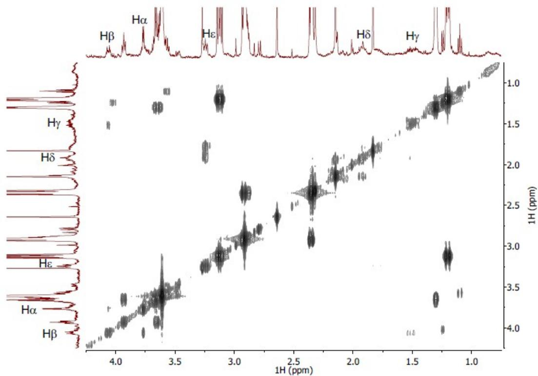
**Fig. S32** NMR analyses of TMLH-catalysed hydroxylation of dimethylisopropyllysine (**16**).  $^1\text{H}$  NMR data of TMLH-catalysed C-3 hydroxylation of dimethylisopropyllysine (top). COSY data of TMLH-catalysed C-3 hydroxylation of dimethylisopropyllysine (bottom).
