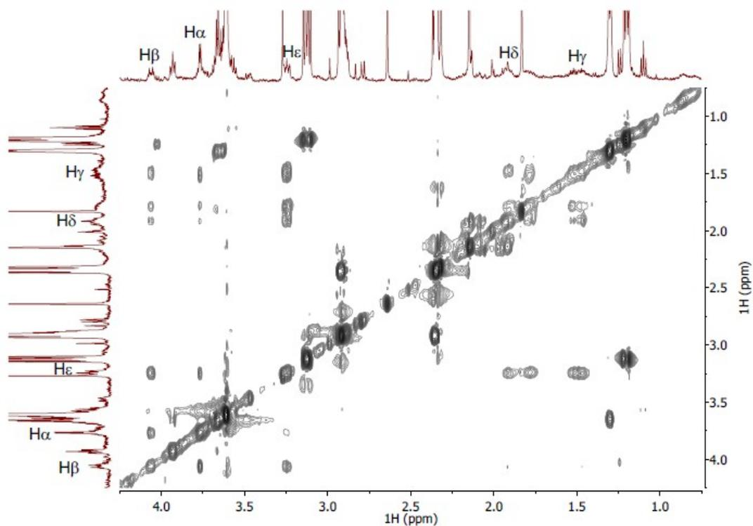
**Fig. S33** NMR analyses of TMLH-catalysed hydroxylation of dimethylisopropyllysine (**16**). Multiplicity-edited HSQC data of TMLH-catalysed C-3 hydroxylation of diimethylisopropyllysine (top; red = positive, CH/CH<sub>3</sub>, blue = negative, CH<sub>2</sub>). TOCSY data of TMLH-catalysed C-3 hydroxylation of dimethylisopropyllysine (bottom).
