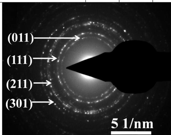
**Fig. S1** Selected area electron diffraction pattern of CoP NPs.
