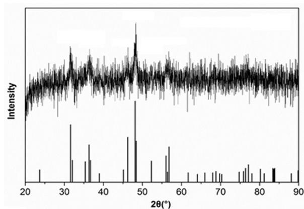
**Fig. S11** XRD pattern of CoP catalyst after recycling seven times for system containing aqueous solution of AB at 298 K.
