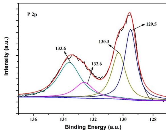
**Fig. S9** High-resolution XPS survey spectra of P 2p core level for CoP NPs after adding NaOH.
