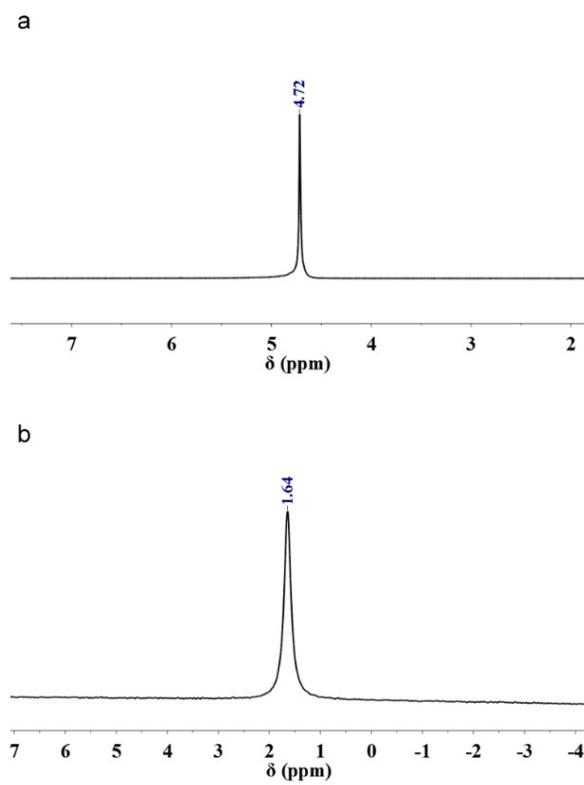
**Fig. S6**  $^1\text{H}$  NMR (a) and  $^{11}\text{B}$  NMR (b) spectra recorded after reaction of AB solution in  $\text{D}_2\text{O}$  containing CoP and 0.3 M NaOH at 298 K.
