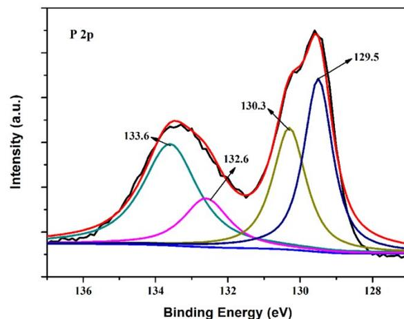
**Fig. S8** High-resolution XPS survey spectra of P 2p core level for CoP NPs before adding NaOH.
