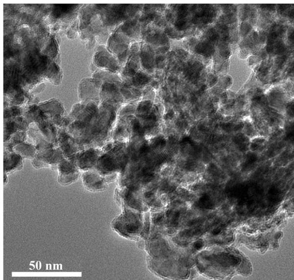
**Fig. S12** TEM image of CoP catalyst after recycling seven times for system containing aqueous solution of AB at 298 K.
