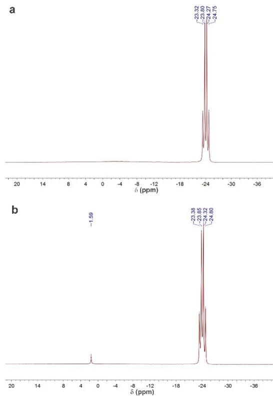
**Fig. S5**  $^{11}\text{B}$  NMR spectra of AB solution in  $\text{D}_2\text{O}$  at 298 K (a) after storing sample for 1 week and (b) after addition of NaOH and storing for 1 week.
