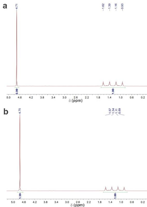
**Fig. S4** <sup>1</sup>H NMR spectra of AB solution in D<sub>2</sub>O at 298 K, (a) after storing sample for 1 week and (b) after addition of NaOH and storing for 1 week.
