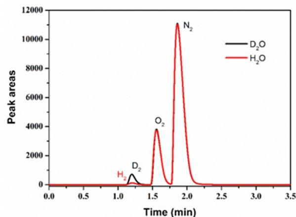
**Fig. S7** Recorded peak areas of isovolumetric gases corresponding to labeled and unlabeled  $\text{H}_2$  produced in reaction systems containing CoP (2 mg), AB (10 mg), NaOH (10 mg), and  $\text{D}_2\text{O}$  or  $\text{H}_2\text{O}$  (2 mL) at 298 K. Results are based on gas chromatographic response to  $\text{D}_2$  over  $\text{H}_2$ , with He as carrier gas.
