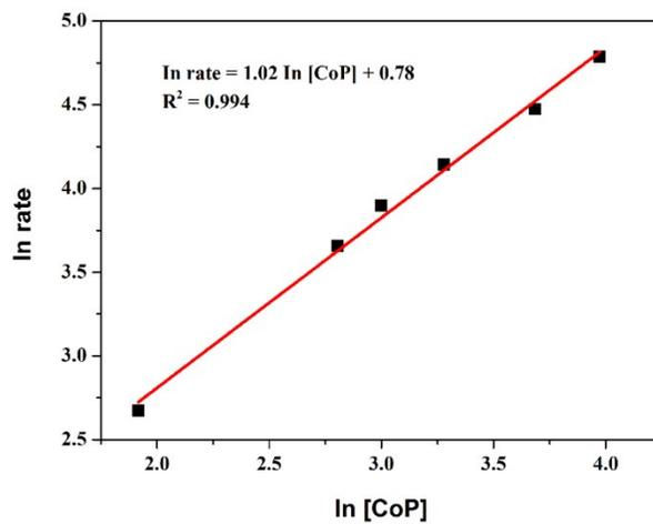
**Fig. S2** Logarithmic plots of  $H_2$  generation rate versus CoP concentration in pure  $H_2O$  at 298 K.
