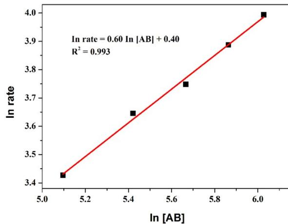
**Fig. S3** Logarithmic plots of H<sub>2</sub> generation rate versus AB concentration in pure H<sub>2</sub>O at 298 K.
