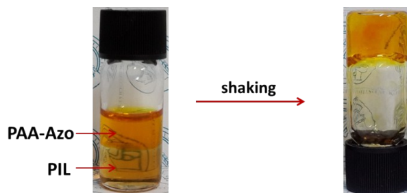
Figure S3 Photographs of PIL and PAA-Azo in DMF before and after shaking.
