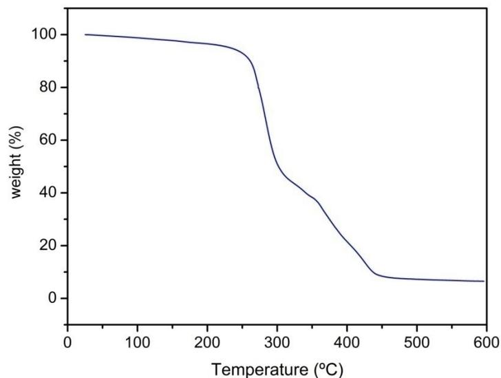
**Figure S17.** Thermogravimetric analysis for compound **3** in the range 25 - 600°C.
