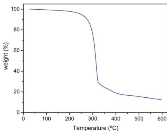
**Figure S5.** Thermogravimetric analysis for compound **1** in the range 25- 600 °C.
