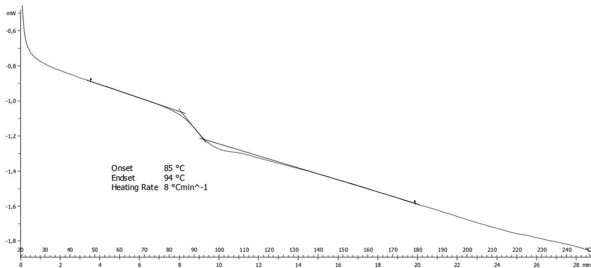
**Figure SI- 26.** Differential scanning calorimetry of poly(*N*-methyl-2-vinylazaborine) (**3**) under a nitrogen atmosphere; sample weight: 4.4292 mg; heating rate: 8.00 K/min; crucible: 40  $\mu$ L aluminium; T<sub>g</sub>: 85 °C (onset); exo up.
