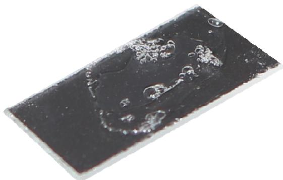
**Figure SI- 28.** Transparent film of poly(*N*-methyl-2-vinylazaborine) (**3**) on a glass plate after removing the solvent from the dichloromethane solution on a heating plate at 40 °C under inert conditions.
