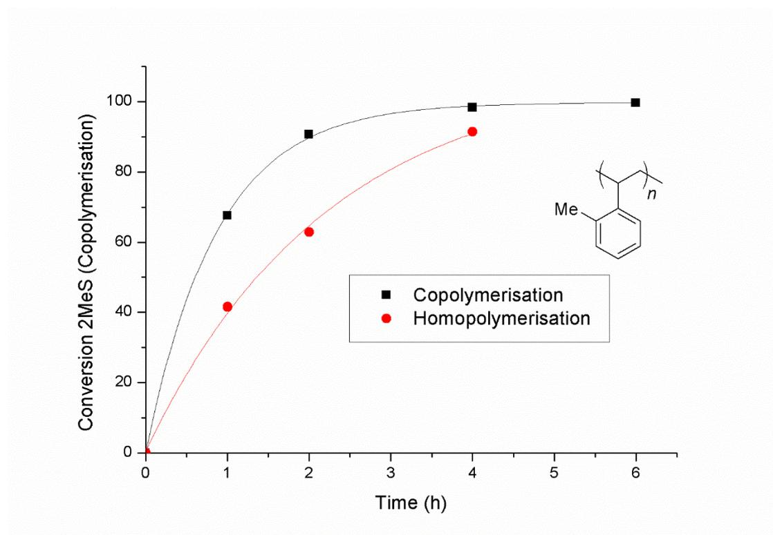
Figure SI- 52. Monomer conversion of polymerizing 2-methylstyrene (5).
