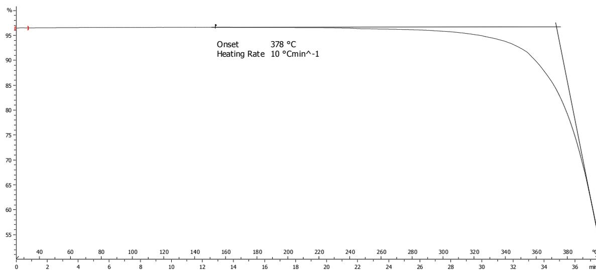
**Figure SI- 36.** Thermogravimetric analysis curve of copolymer **6** under nitrogen atmosphere; sample weight: 11.5770 mg; heating rate: 10 K/min; crucible: 40  $\mu$ L aluminium;  $T_d$ : 378 °C (onset).
