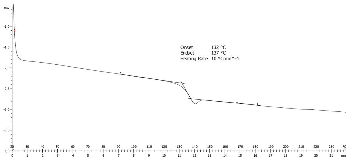
**Figure SI- 44.** Differential scanning calorimetry curve of poly(2-methylstyrene) (**4**) under a nitrogen atmosphere; sample weight: 8.2736 mg; heating rate: 10 K/min; crucible: 40  $\mu$ L aluminium;  $T_g$ : 132 °C (onset); exo up.
