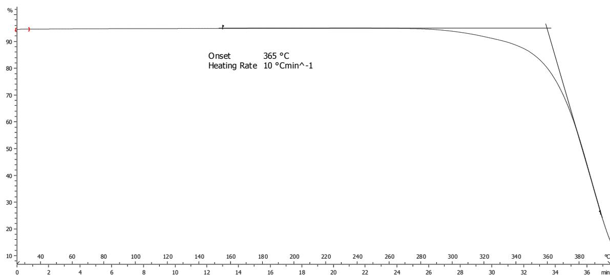
**Figure SI- 45.** Thermogravimetric analysis curve of poly(2-methylstyrene) (**4**) under a nitrogen atmosphere; sample weight: 7.1067 mg; heating rate: 10 K/min; crucible: 40  $\mu$ L aluminium;  $T_d$ : 365 °C (onset).
