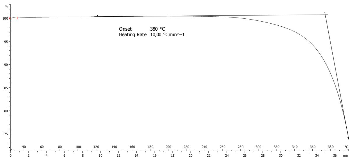
**Figure SI- 27.** Thermogravimetric analysis curve of poly(*N*-methyl-2-vinylazaborine) (**3**) under a nitrogen atmosphere; sample weight : 7.1430 mg; heating rate: 10.00 K/min; crucible: 40  $\mu$ L aluminium;  $T_d$ : 380 °C (onset); exo up.
