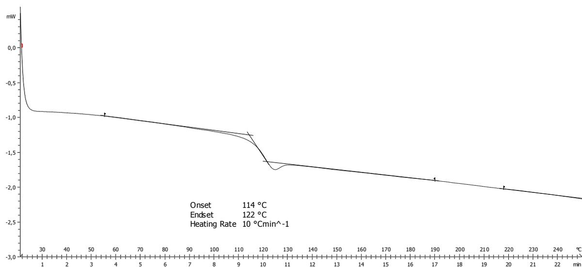
**Figure SI- 35.** Differential scanning calorimetry curve of copolymer **6** under a nitrogen atmosphere; sample weight: 8.4226 mg; heating rate: 10 K/min; crucible: 40  $\mu$ L aluminium;  $T_g$ : 114 °C (onset); exo up.
