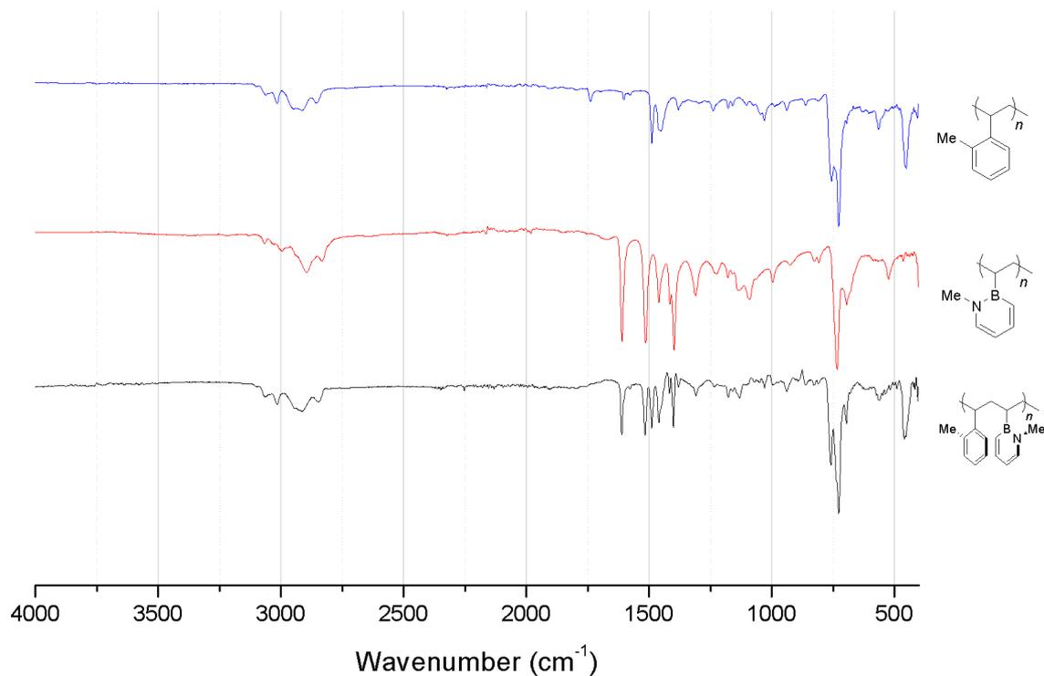
Figure SI- 49. Stacked IR spectra of the homopolymers 3, 4 and copolymer 6.
